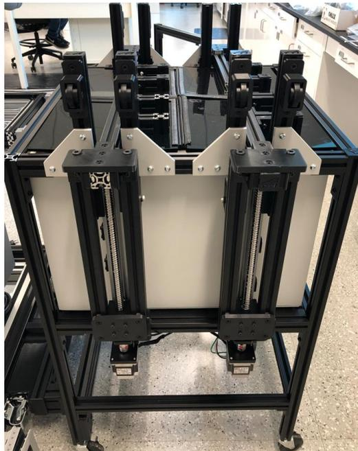
**Figure 7. Specimen Conditioning Unit for IDEAL-CT (or IDEAL-RT)**
