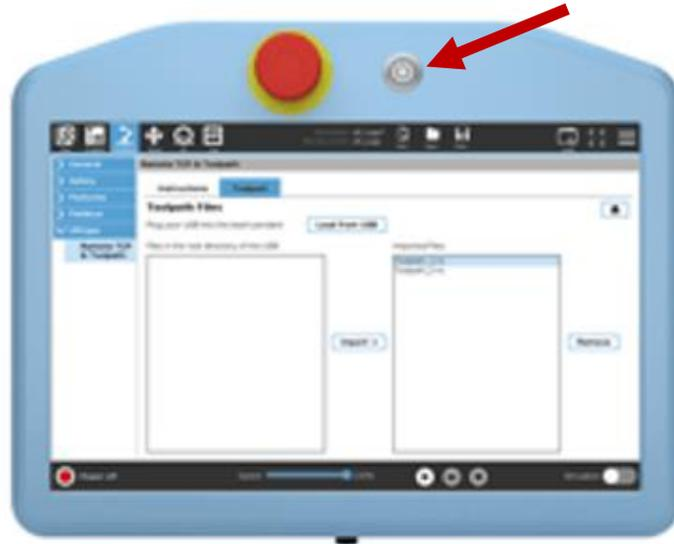
**Figure 14. Robot Arm Power Button**
