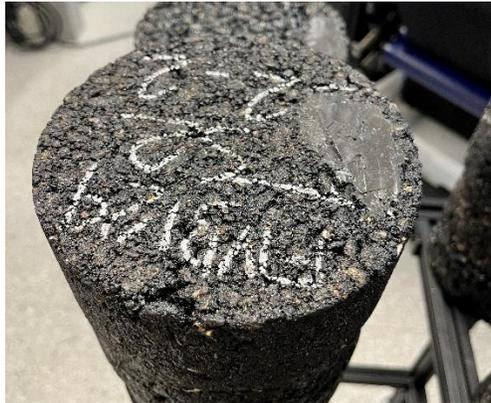
**Figure 12. RFID Tag on Asphalt Specimen**
