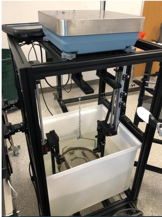
**Figure 5. Weight Measurement Component**
