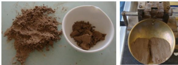
Sandy Clay soil Loop 480 (Laredo District) Station 2154+00
