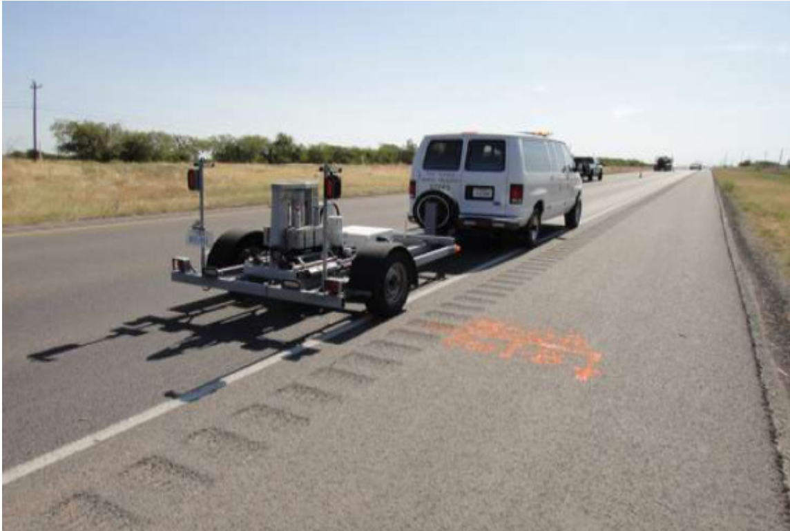
Figure 5-5. FWD Testing on SH 114 (Fort Worth, Summer 2011).
