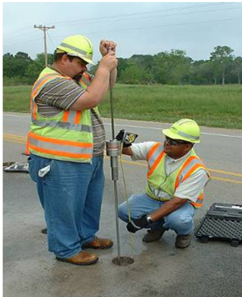
Figure 5-1. Illustration of DCP Testing.
