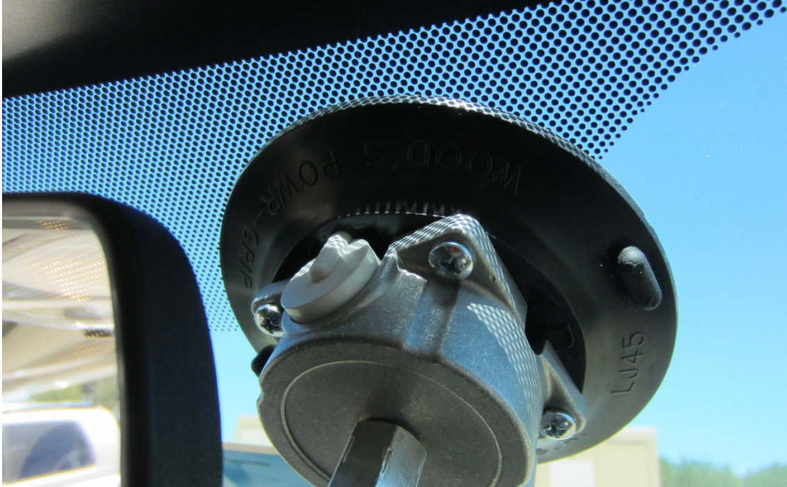
Figure 14. Potential Mounting Problem from Tint and Proximity to Rearview Mirror.
