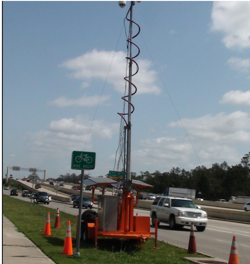
Figure 38. TTI Data Collection Trailer Deployed at a Freeway Ramp Location in Houston.
