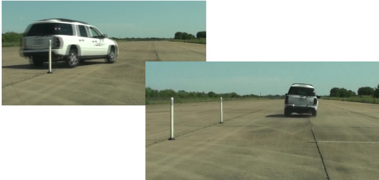
Figure 64. Test Vehicle Encroaching 1/4 Lane after Weaving between Pylons.
