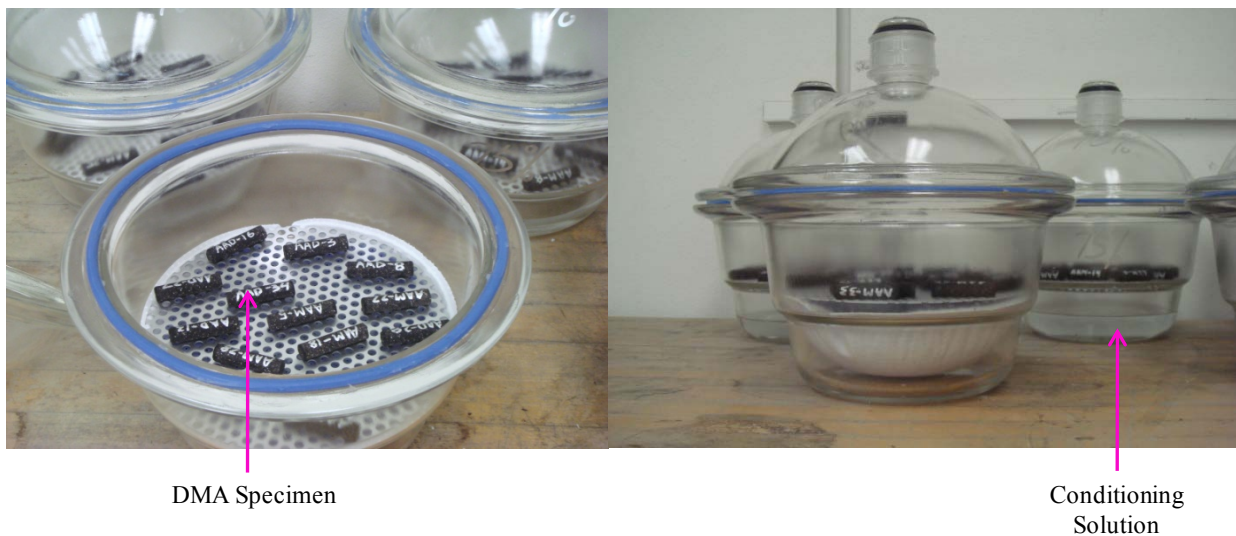
Figure 104. DMA Specimens Conditioning in Desiccators.
