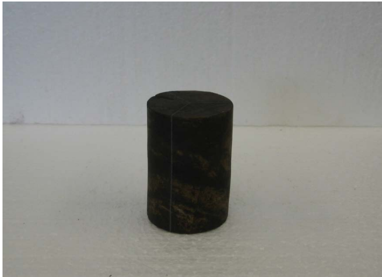
(b) Limestone Specimen Soaked in AAD Asphalt Binder for 32 Hours
