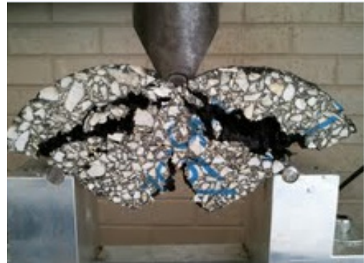
Multiple cracking in R-SCB specimens
