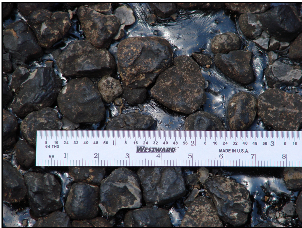
Figure 1. Grade 3 Lightweight Aggregate Seal Coat.
