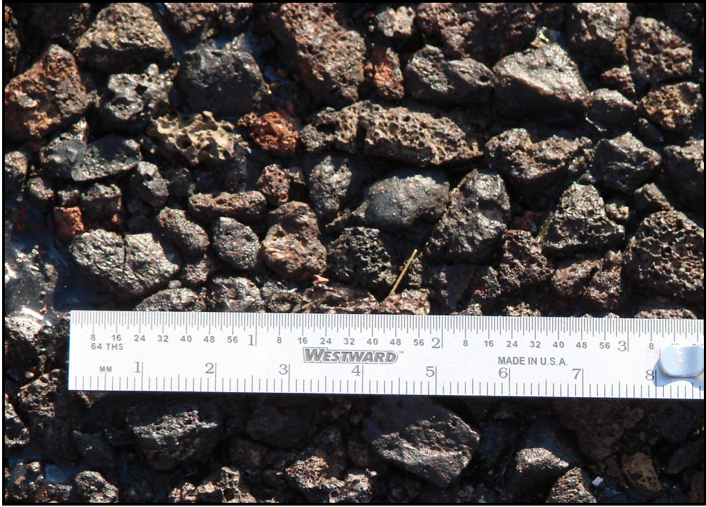
Figure 8. Grade 4S Scoria Aggregate Seal Coat.
