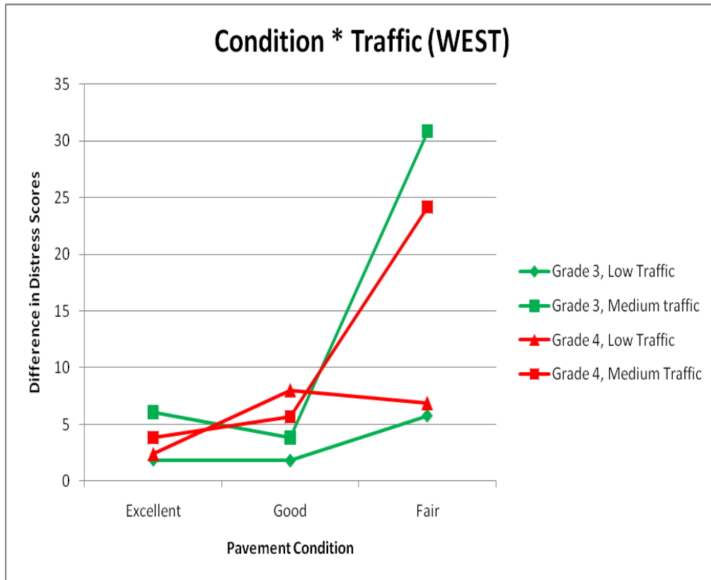
Figure 33. Interaction Plot for 1998 Pre-Construction Pavement Condition and Traffic Level by Grade, Western Region.
