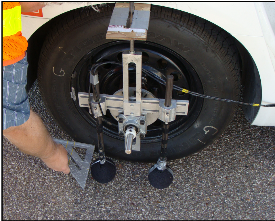
Figure 9. Mounted TxDOT OBSI Noise Testing Equipment.
