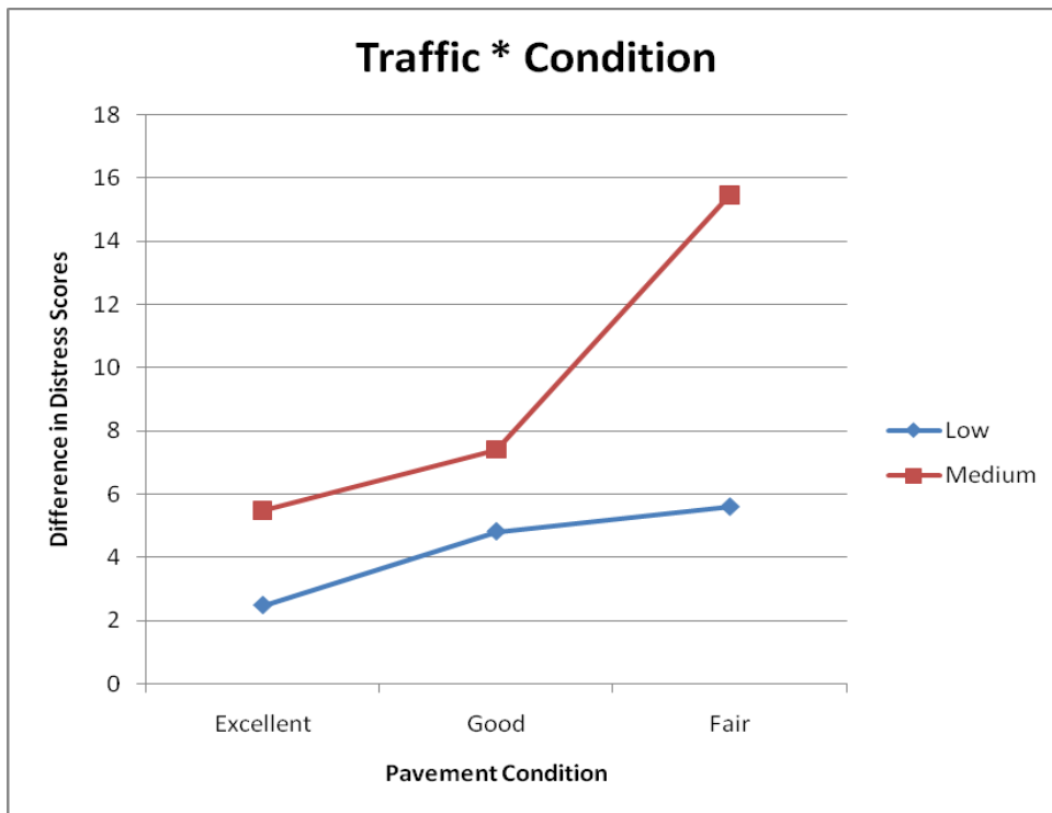
Figure 31. Interaction Plot for 1998 Traffic Level and Pre-Construction Pavement Condition.
