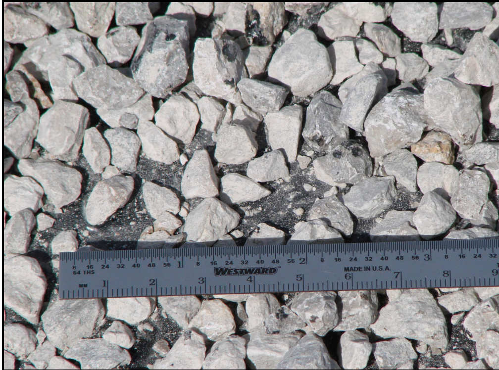
Figure 5. Grade 4 Limestone Aggregate Seal Coat (1CY/120SY).
