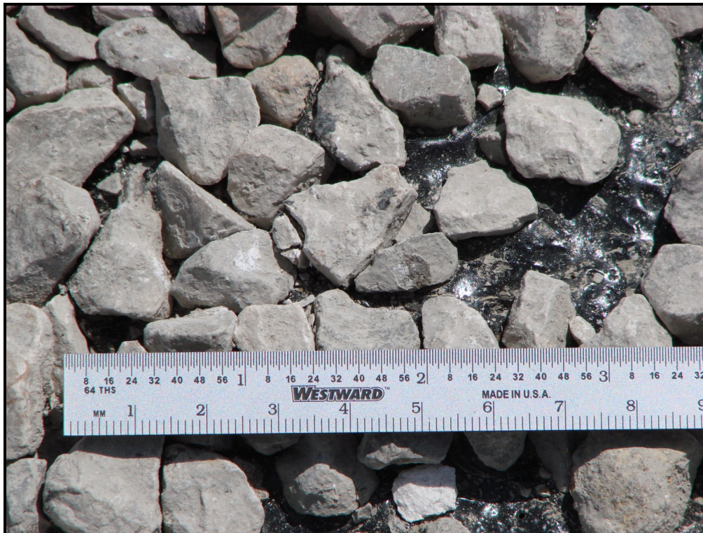
Figure 4. Grade 3 Limestone Aggregate Seal Coat (1CY/85SY).
