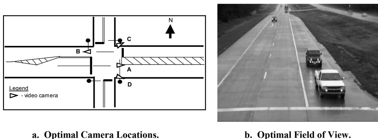
**Figure C-5. Illustrative Optimal Camera Location and Field of View.**
