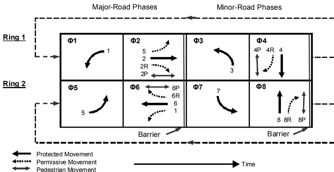
**Figure 2-2. Dual-Ring Structure with Illustrative Movement Assignments.**
