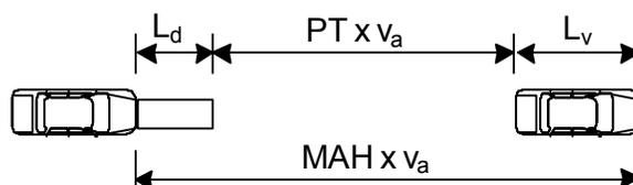
**Figure 2-5. Relationship between Passage Time and Maximum Allowable Headway.**
