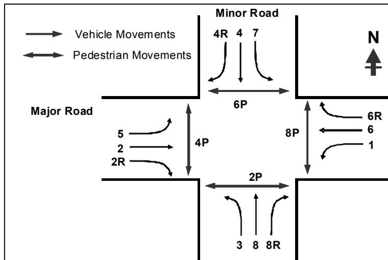
**Figure 2-1. Intersection Traffic Movements and Numbering Scheme.**
