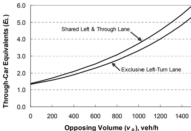
**Figure 3-7. Through-Vehicle Equivalents for Permissive Left-Turn Vehicles.**
