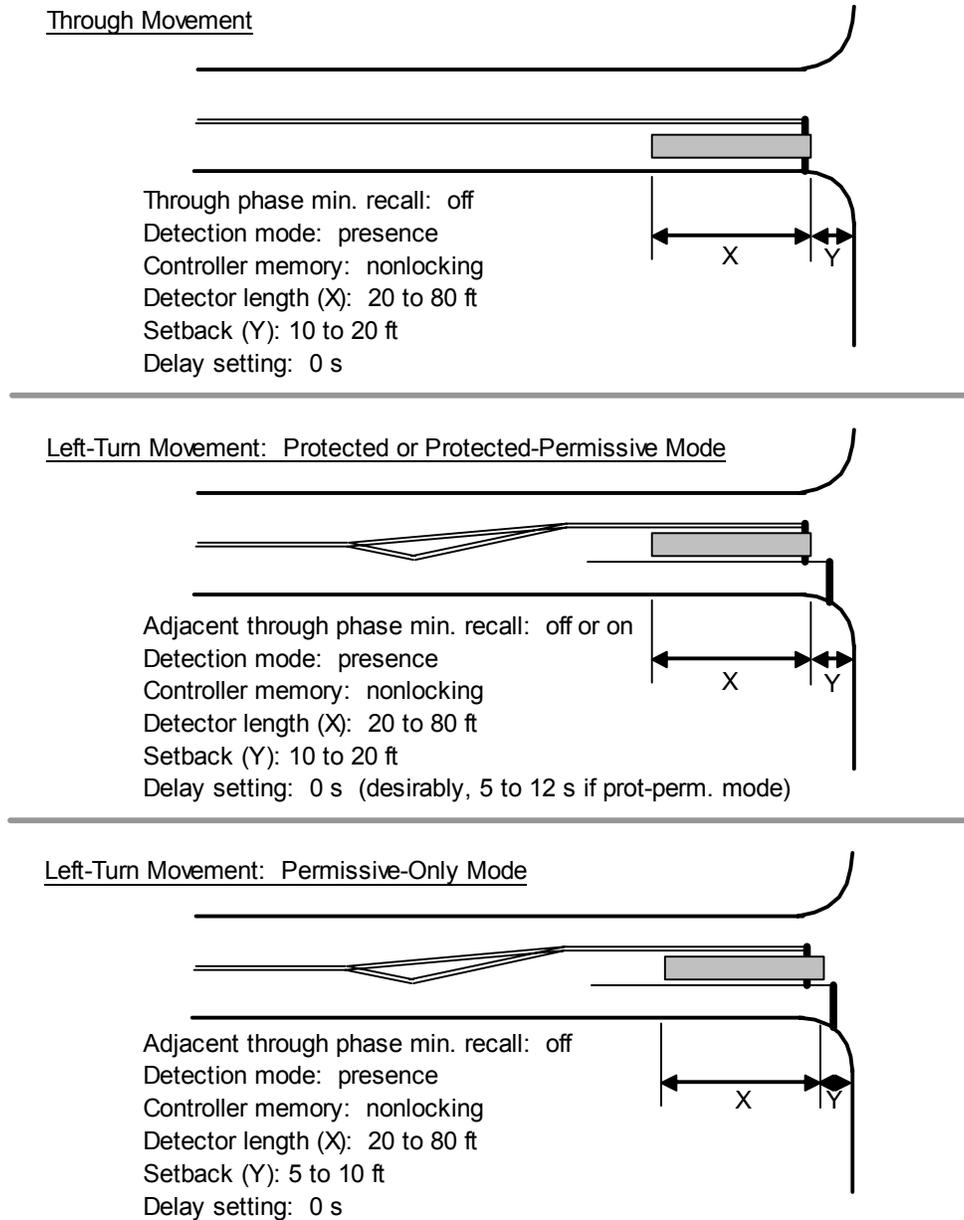
**Figure C-3. Left-Turn and Through Movement Detection Designs.**
