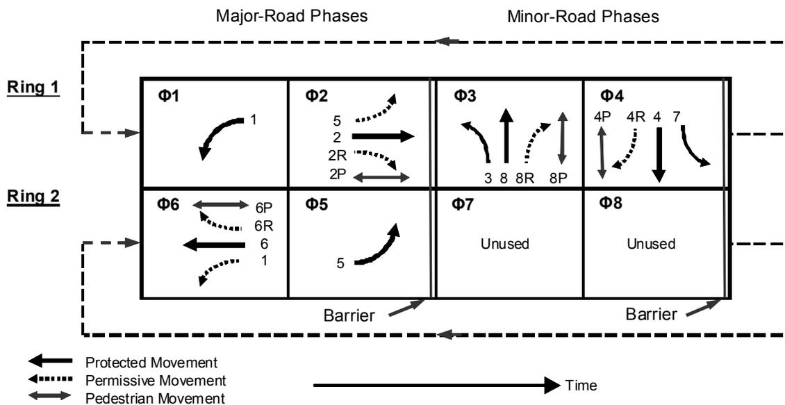
Figure A-3. Illustrative Lead-Lag and Split Phasing.
