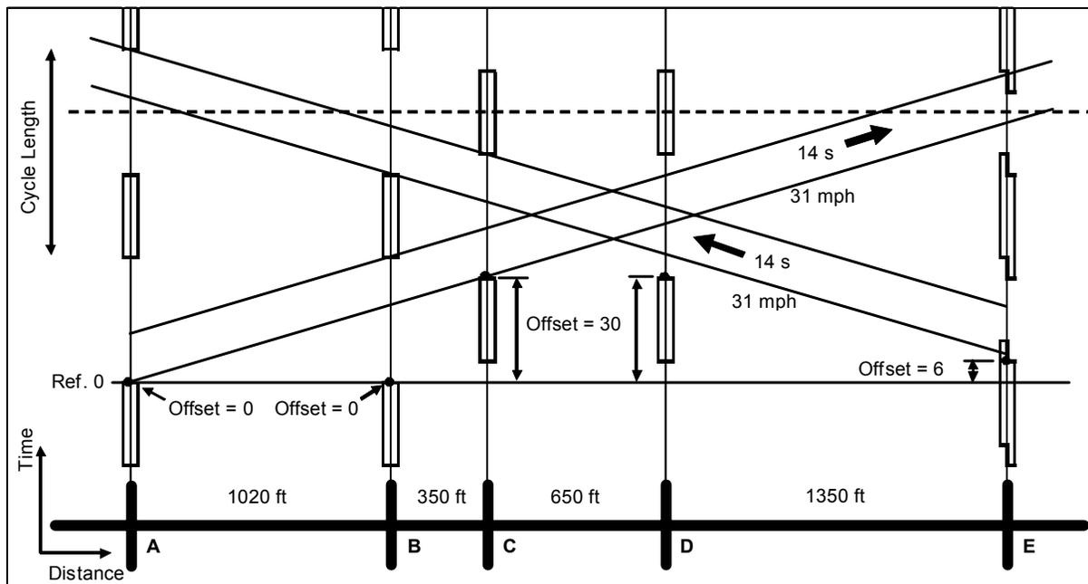
Figure 3-5. Completed Time-Space Diagram.
