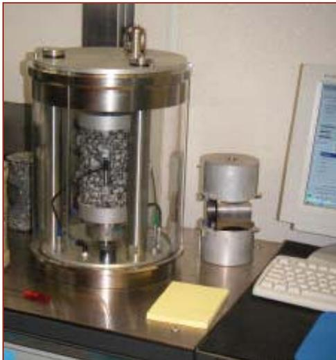
Dynamic modulus testing setup
