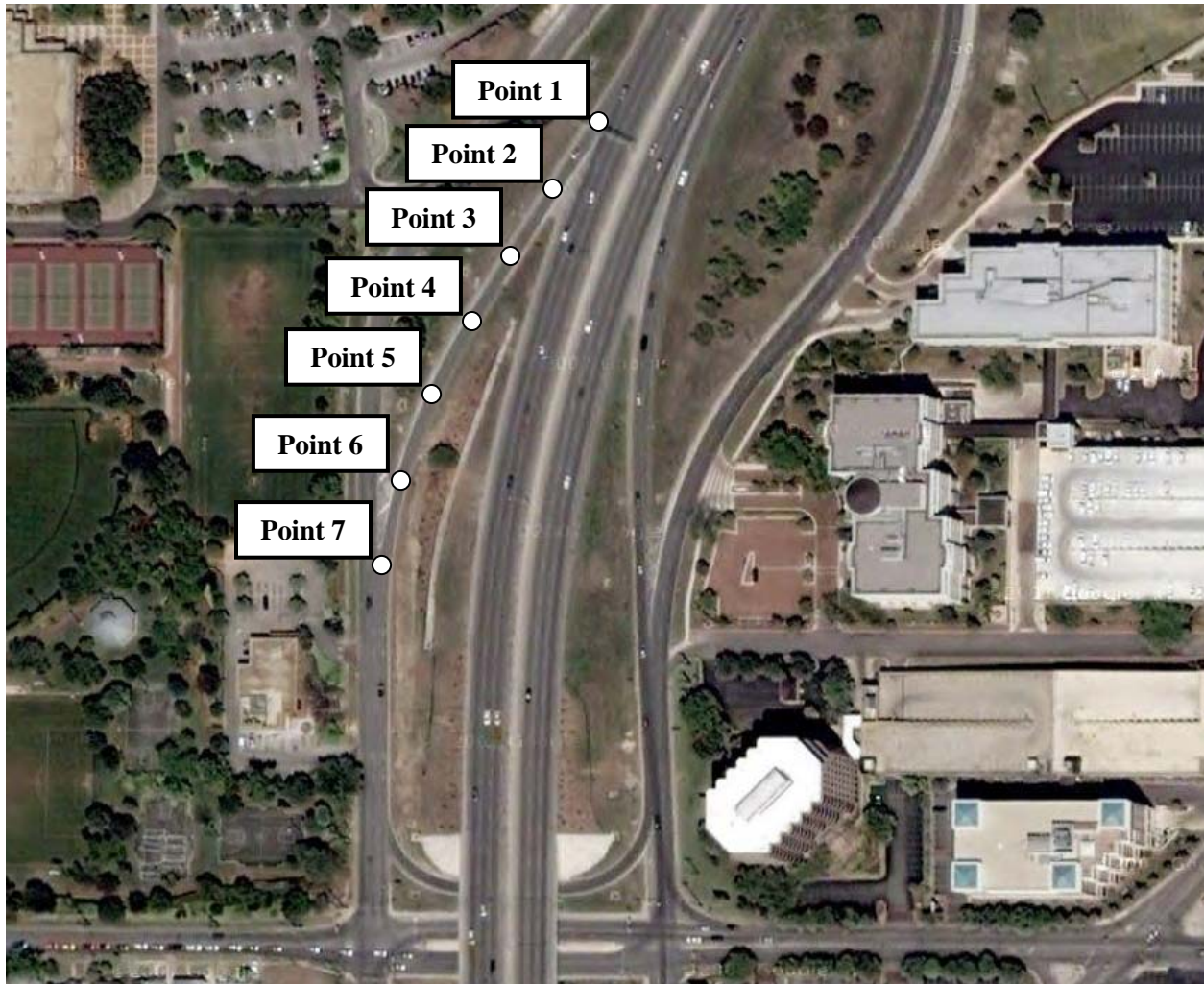
Figure 22. Exit Ramp Speed Check Points for US 281 Southbound Exit to Mulberry, San Antonio, Texas.
