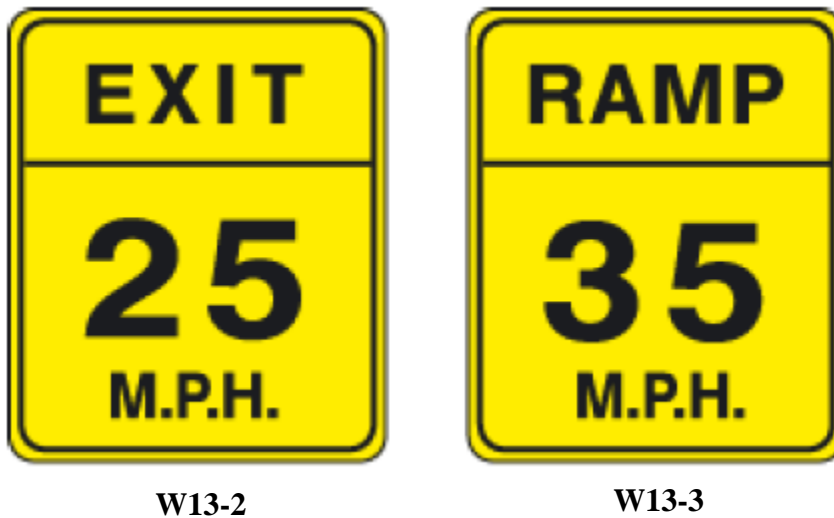
Figure 1. Exit Speed and Ramp Speed Signs (1).
