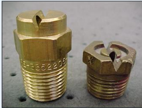
Figure 1 – Taller Nozzle for Outside Wheel Paths, Shorter Nozzle for Wheel Paths
