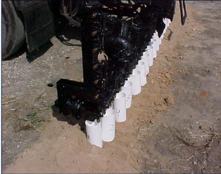
Figure 4 – Cylinders Placed Under the Nozzles
