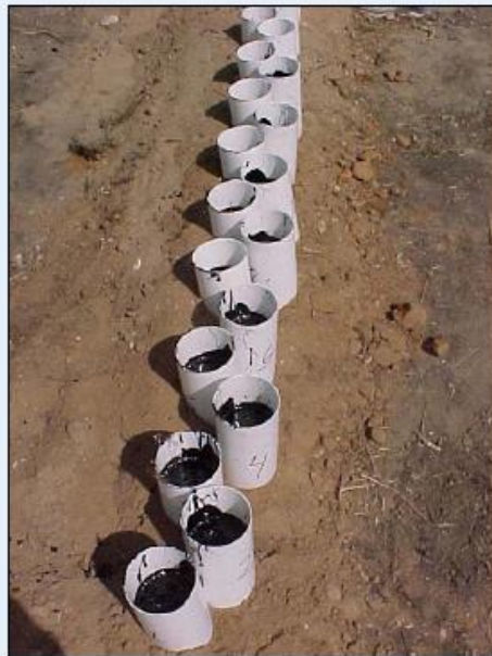
Figure 5 – Cylinders \frac{3}{4} Filled with Asphalt
