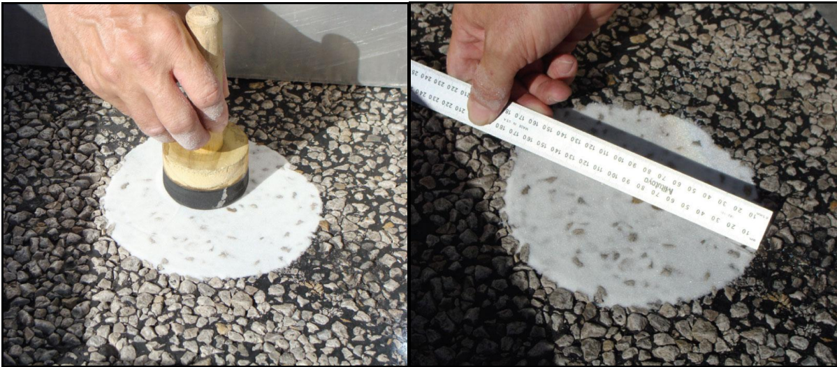
Figure 14. Sand Patch Test Equipment.
