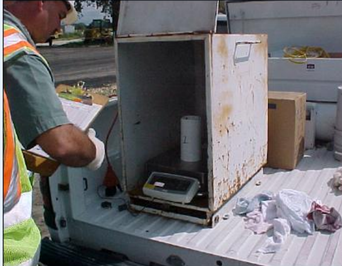
Figure 6 – Weighing Cylinders to Nearest Gram
