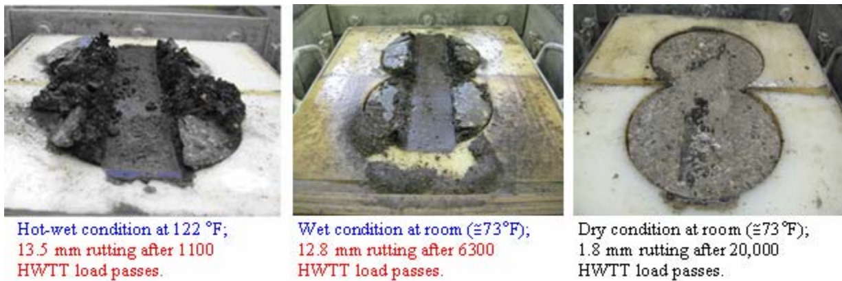
Figure 5-4. Hamburg Results (Cores) – FM 140/SH 97 Intersection (Charlotte).
