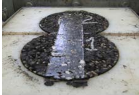
Hamburg dry condition at room (73 °F); 1.3 mm rutting after 20,000 HWTT load passes.
