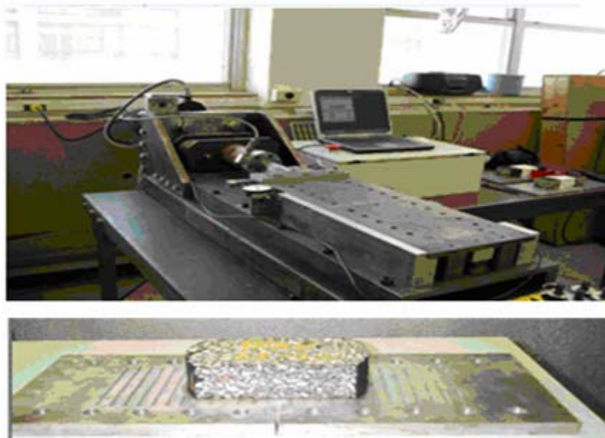
Figure 4-2. The Overlay Tester and Specimen Setup.
