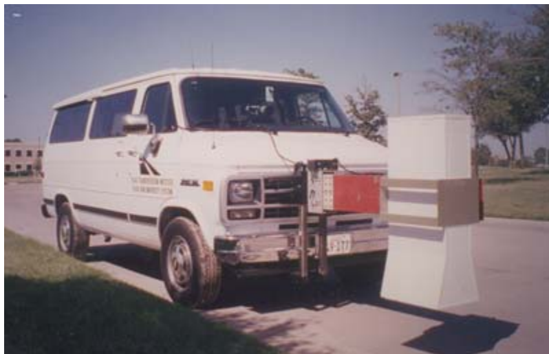
Figure 4-5. TTI's GPR System Setup.
