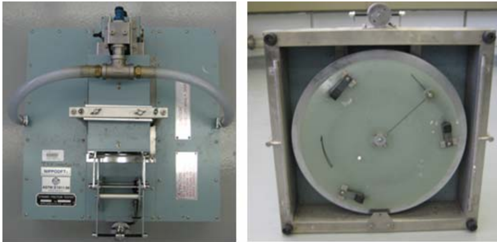
Figure 4-4. TTI’s Newly Acquired Dynamic Friction Tester Device.
