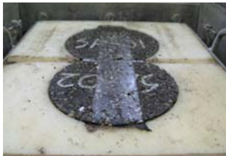
Hamburg dry condition at room (73 °F); 1.7 mm rutting after 20,000 HWTT load passes.
