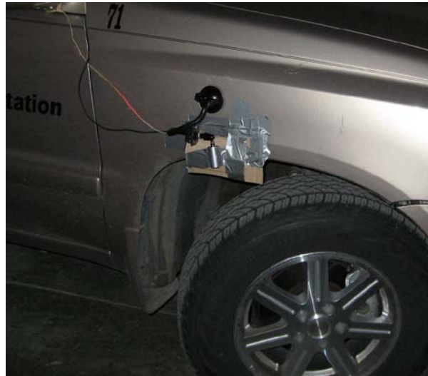
Figure 18. Camera Mounted over Front Right Wheel.
