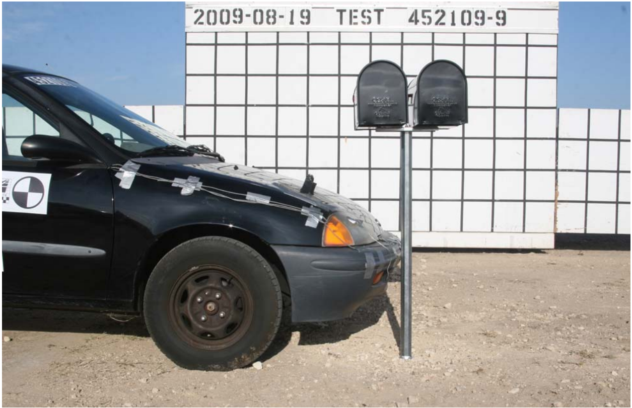
Figure 5. Vehicle/Installation Geometrics for Test No. 452109-9.
