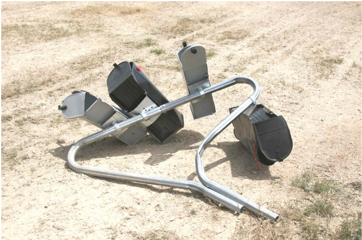
Figure 15. Installation after Test No. 452109-10.
