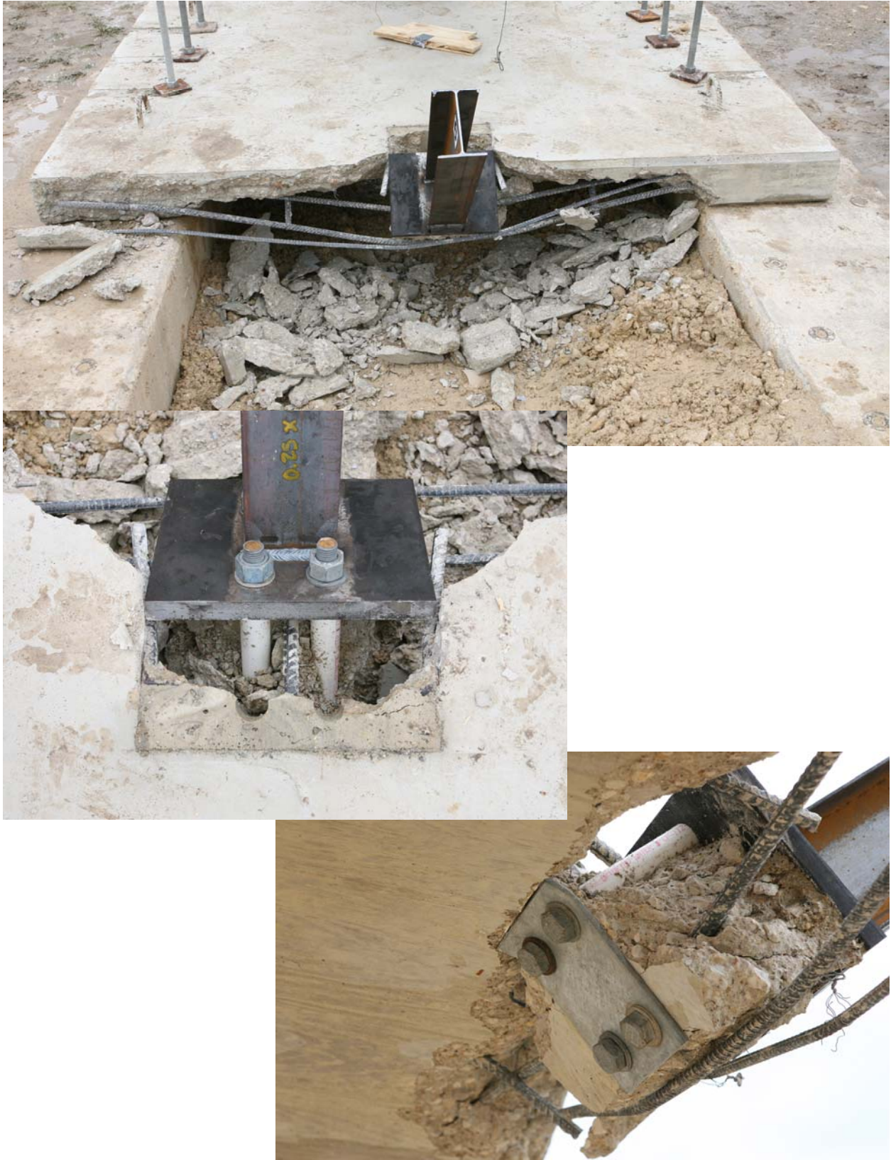
Figure 4.16. T8 Post with 3/4-Inch Slots after Test 452107-P6.
