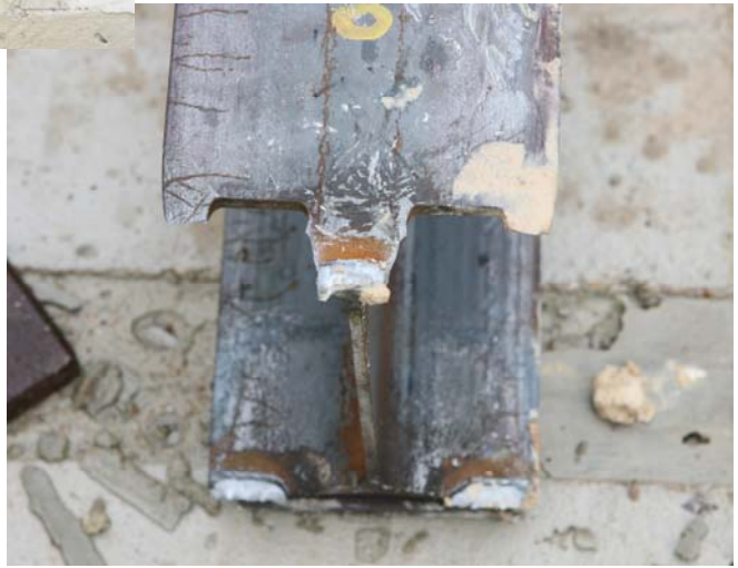
Figure 4.14. T8 Post with 1-Inch Slots after Test 452107-P5.
