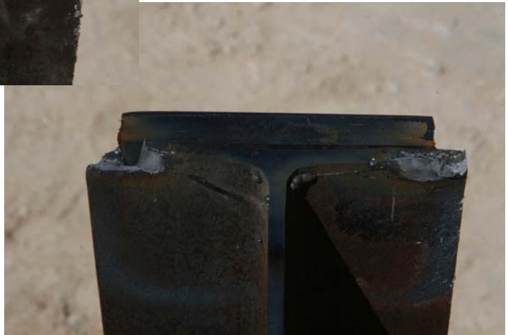
Figure 4.6. T8 Post with \frac{3}{4} -Inch Slots after Test 452107-P2.
