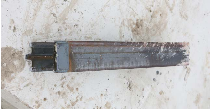
Figure 4.20. T8 Post with 7/8-Inch Slot after Test 452107-P8.
