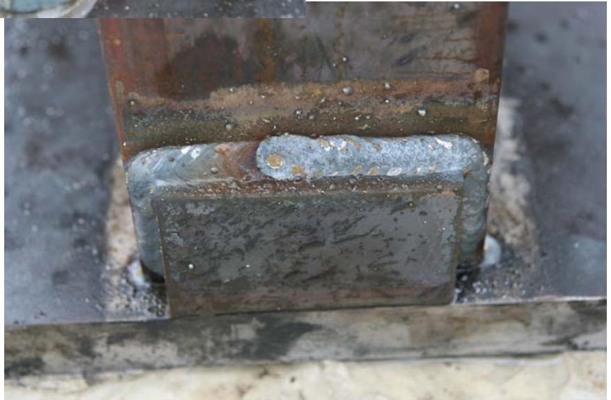
Figure 4.13. T8 Post with 1-Inch Slot before Test 452107-P5.
