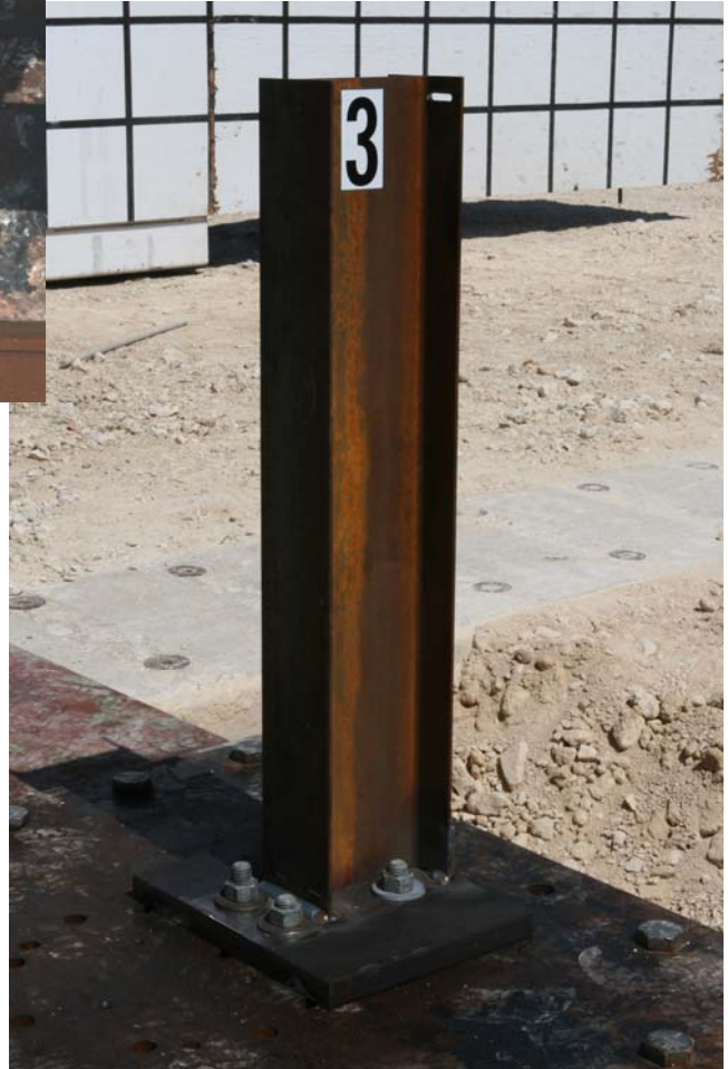
Figure 4.7. T8 Post with 1-Inch Slot before Test 452107-P3.
