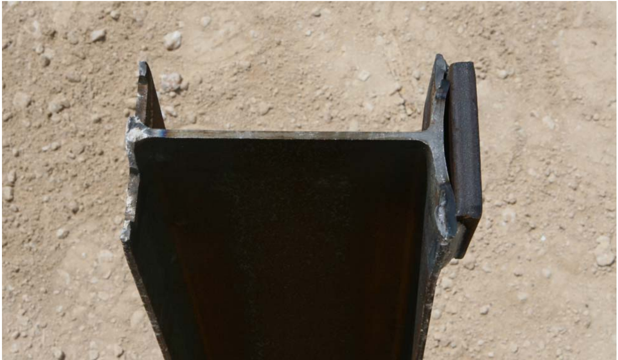
Figure 4.10. T8 Post with 1-Inch Slot after Test 452107-P4.
