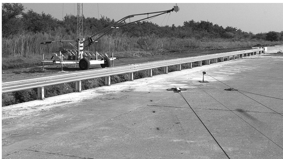
Figure 1.1. T-6 Bridge Rail System.
