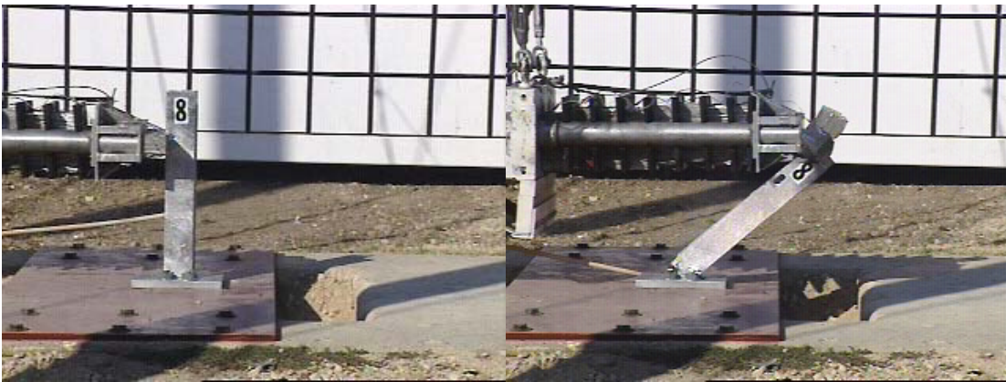
Figure 2.2. Weak Axis Pendulum Test of T6 Breakaway Post.
