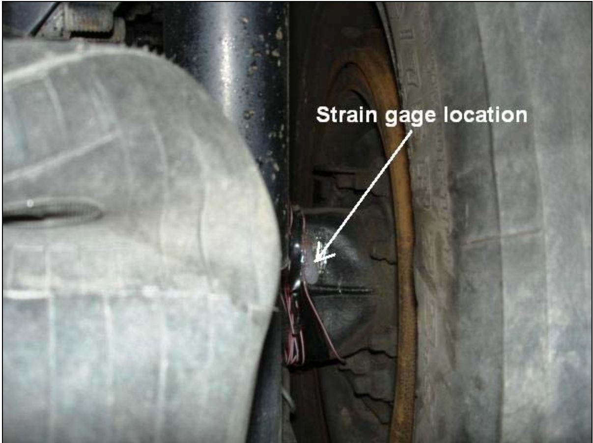
Figure 2.17. Strain Gage Mounted on Drive Axle.
