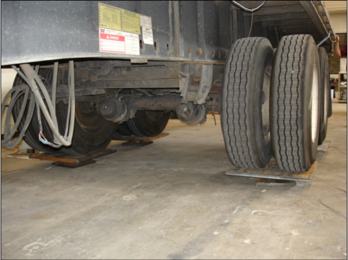
Figure 2.19. Load Cells Positioned under Dual Tires of Trailer Axle Assembly.
