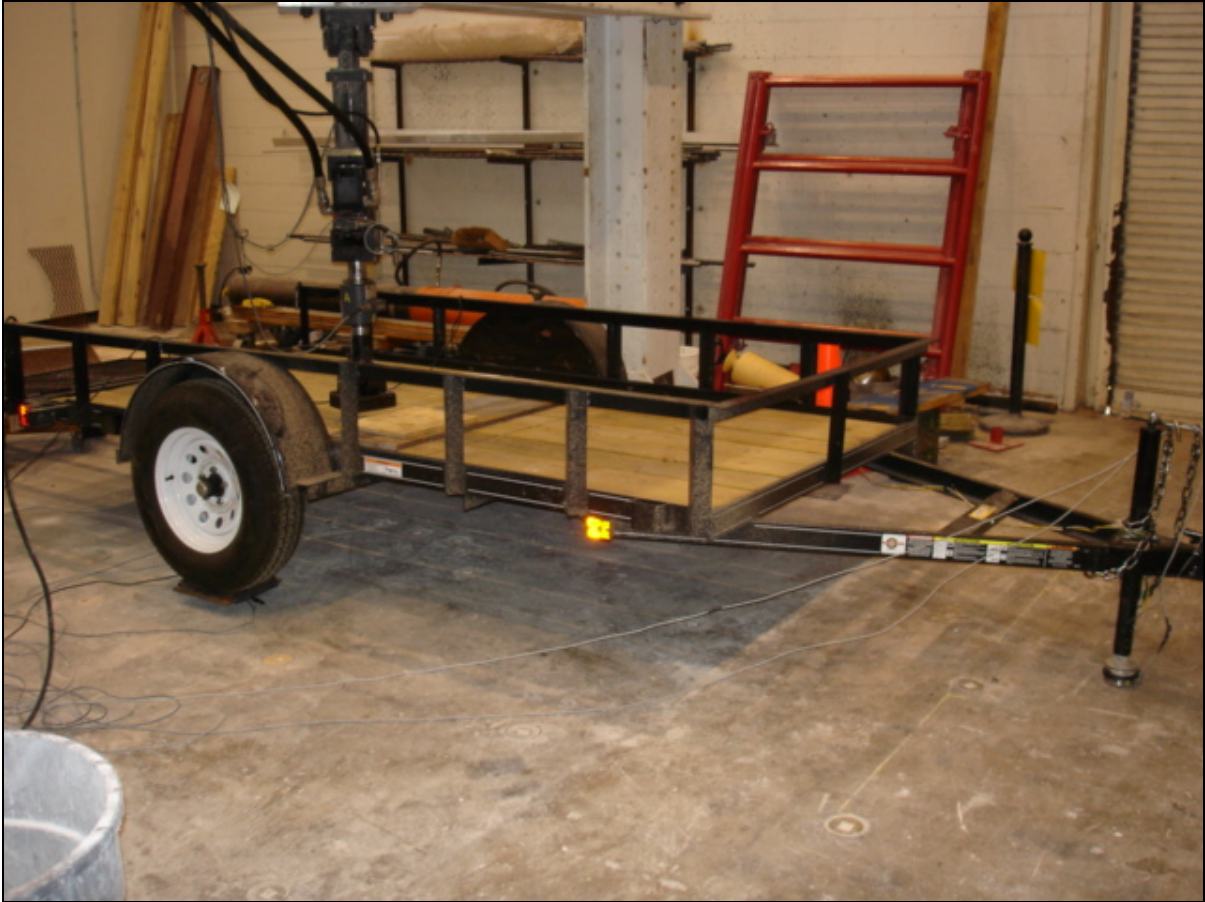
Figure 2.5. Small-Scale Trailer Used to Verify Strain Measurement Methodology.
