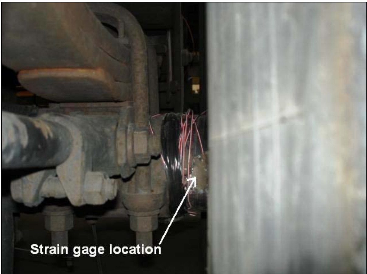
Figure 2.16. Strain Gage Mounted on Trailer Axle.
