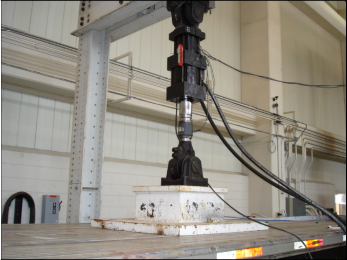
Figure 2.18. Application of Load to Axle Assembly through Loading Plate. (axle assembly underneath the loading plate and load ram)
