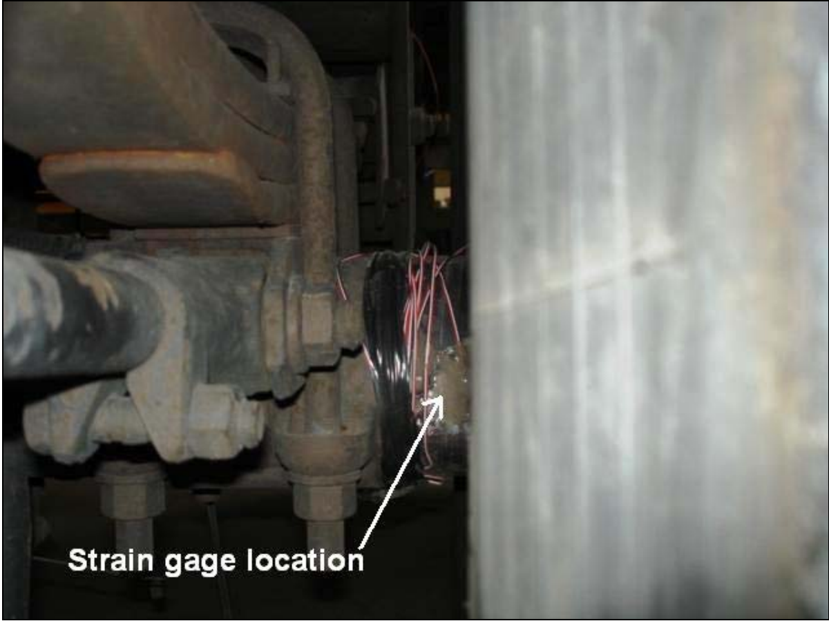
Figure 2.16. Strain Gage Mounted on Trailer Axle.
