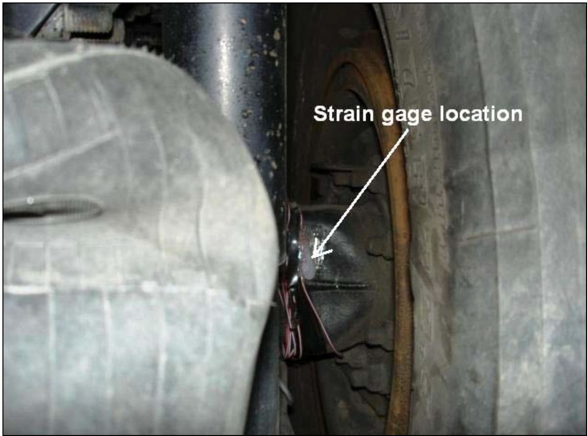
Figure 2.17. Strain Gage Mounted on Drive Axle.
