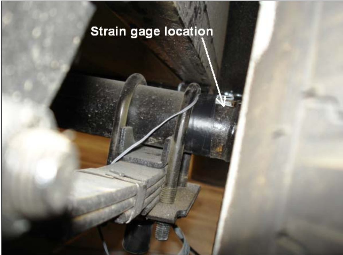
Figure 2.6. Strain Gages Positioned between Suspension and Tire of Small Trailer.
