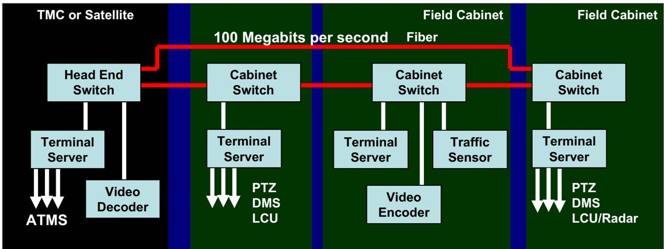
Figure 3. Ethernet Replacing T1.
