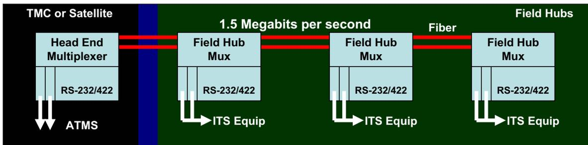
Figure 1. Traditional T1 Field Hub and Satellite Architecture.
