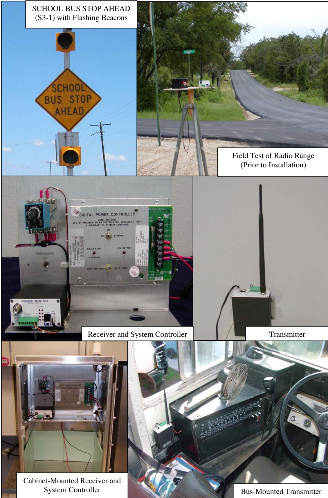
Figure 3. Active Advance Warning Device Components for School Bus Loading/Unloading Zones.
