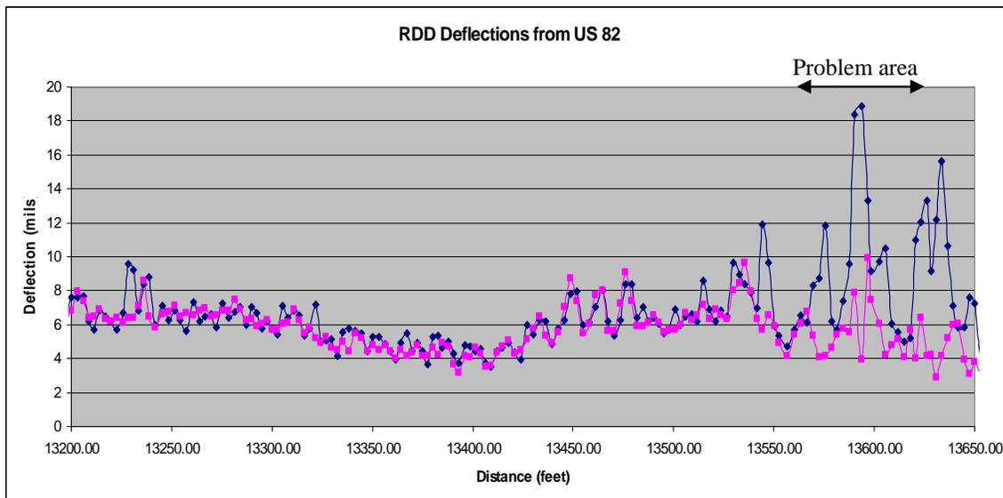
**Figure 14. Typical RDD Profile from US 82 Showing both Low Deflection and High Deflection Areas.**
