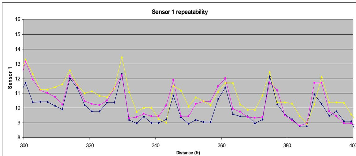
**Figure 10. Maximum Deflection from Replicate Runs of the RDD over Seven Joints at TTI's Riverside Campus.**
