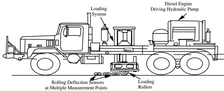
**Figure 1. TxDOT's Rolling Dynamic Deflectometer ([Lee et al., 2004](#)).**
