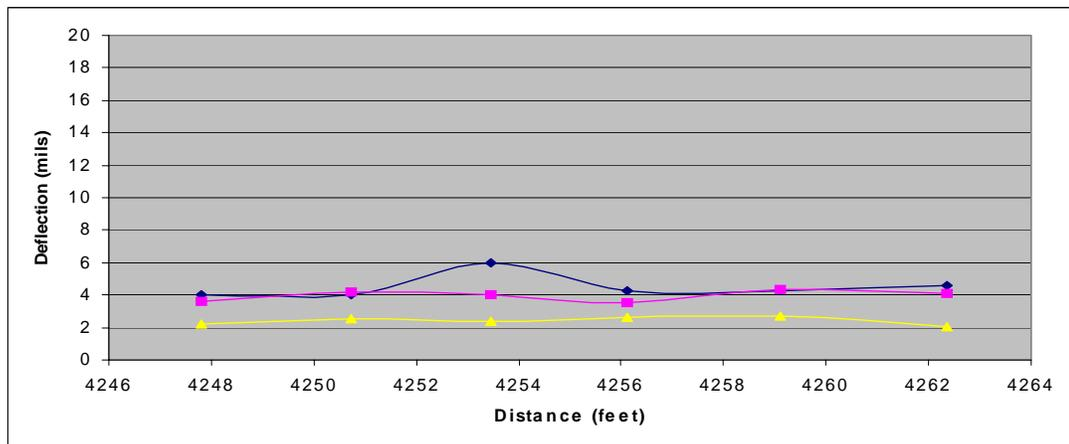
**Figure 7. RDD Data from an Ideal Joint Deflection Pattern.**
