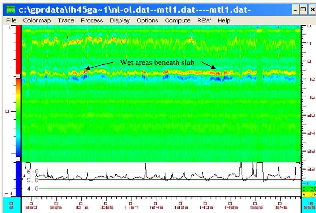
**Figure 17. COLORMAP Display from a Section of JCP with Possible Problem Areas.**
