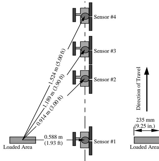
**Figure 2. RDD Loading and Sensor Locations ([Lee et al., 2004](#)).**
