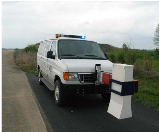
**Figure 15. TxDOTs Air-Coupled GPR Unit.**
