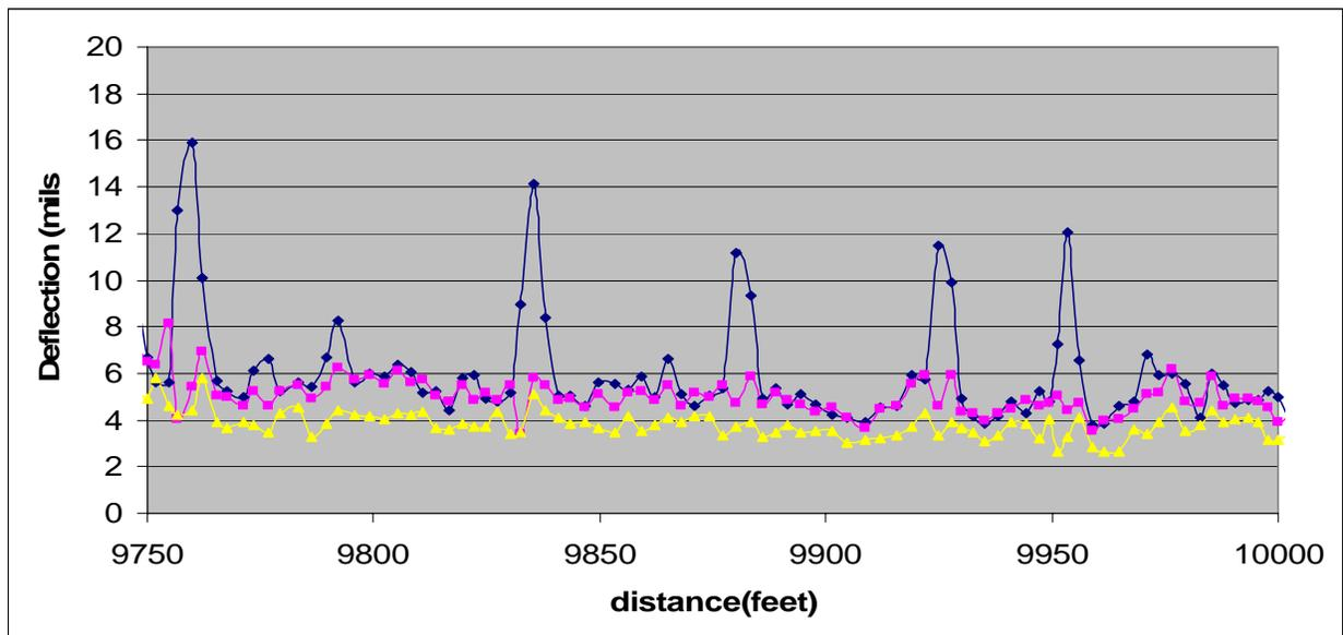
**Figure 4. Typical RDD Three-Channel Deflection Plot for a Section of Jointed Concrete Pavement (Blue, red, and yellow lines are sensors 1, 3, and 4 as described in [Figure 2](#)).**
