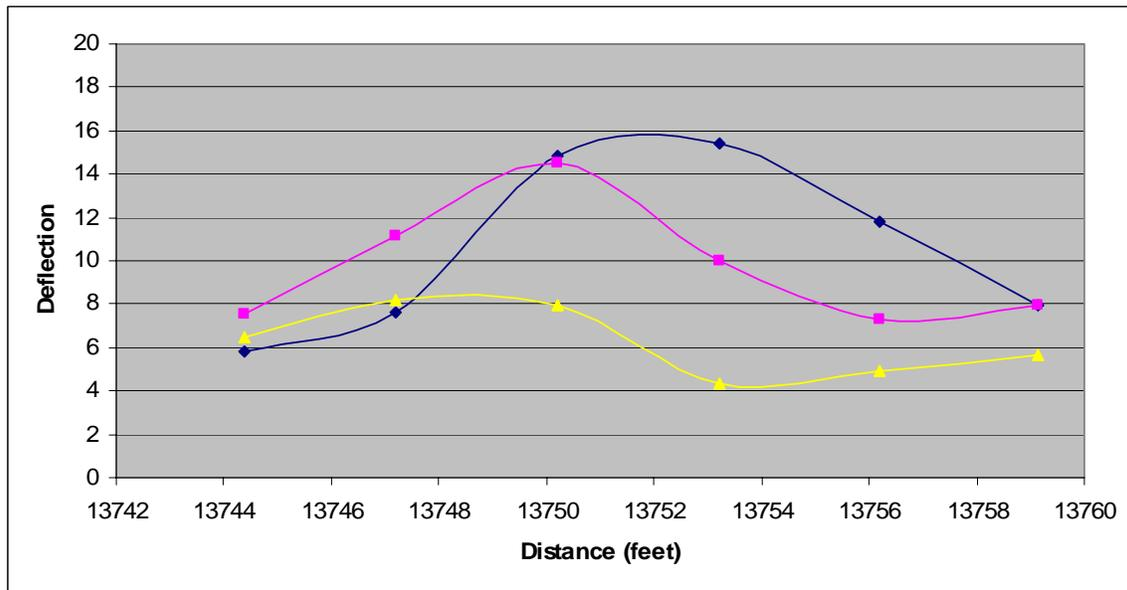
**Figure 8. RDD Data from a High Joint Deflection Location on US 82. (Interpretation: reasonable load transfer, poor slab support)**
