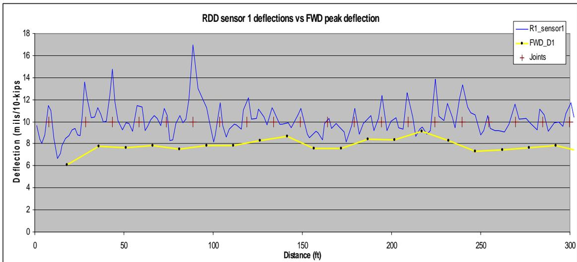
**Figure 12. Comparison of RDD Deflection Profile with FWD Center Slab Deflection Normalized to 10,000 lb.**
