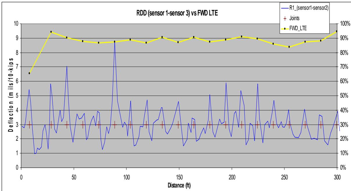
**Figure 13. Comparison of RDD Difference in Deflection between Sensors 1 and 3 against Load Transfer Efficiency Measure by the FWD.**
