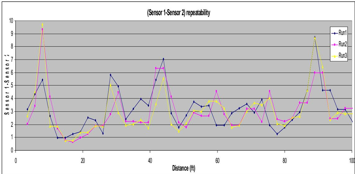
**Figure 11. Difference in Deflection (mils) versus Distance from Three Repeat Runs of the RDD.**
