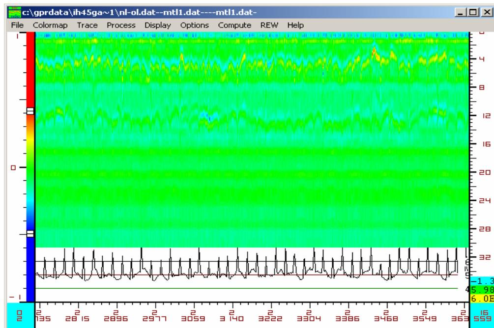
Figure 16. GPR Data from a JCP with no Obvious Sub-Slab Problems.
