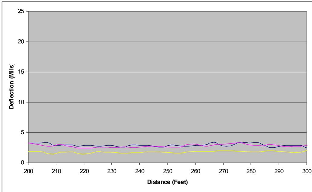
**Figure 6. RDD Deflections from a Low Deflection Area on US 82 (contrast with Figure 5).**
