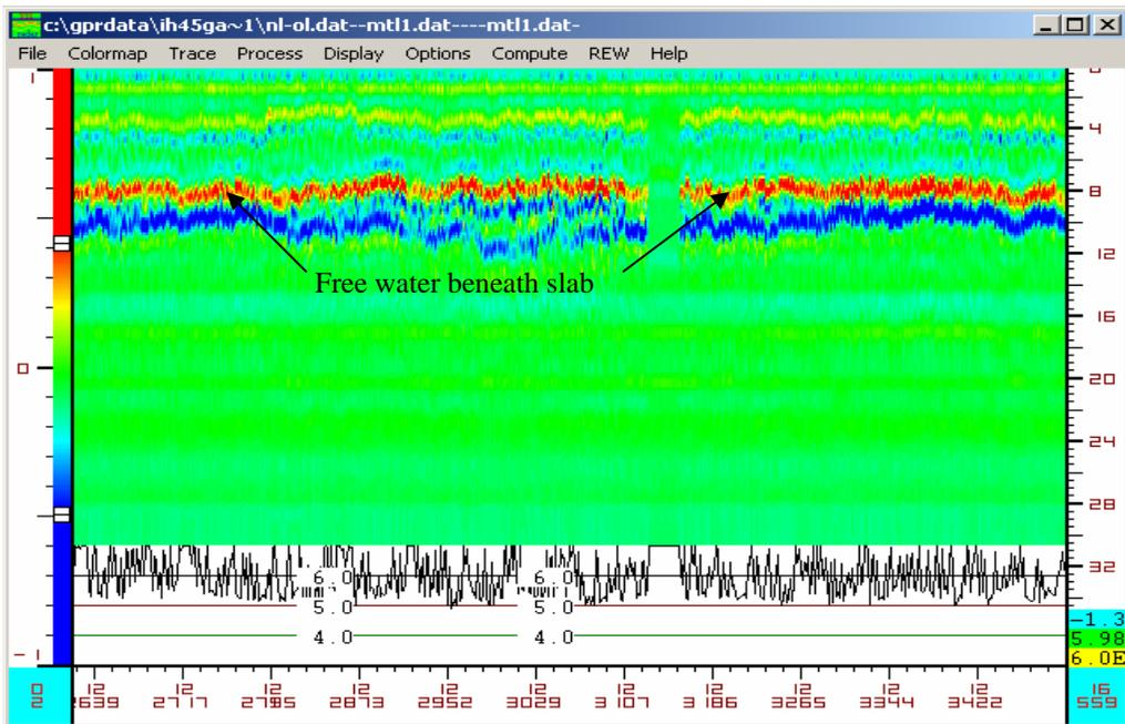
**Figure 18. COLORMAP Display from an Area Where Free Water Exists Beneath the Slab.**
