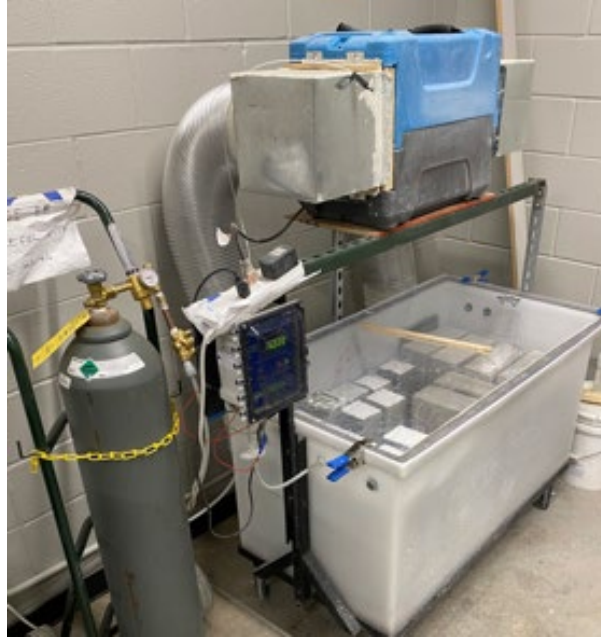
Figure 7.1: Accelerated carbonation chamber
