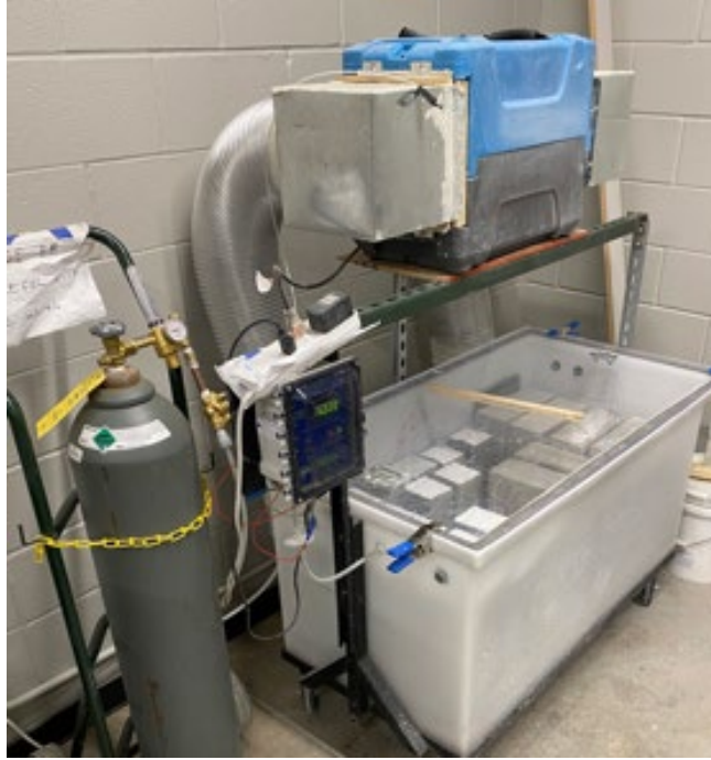
Figure 9.3: Accelerated carbonation chamber.
