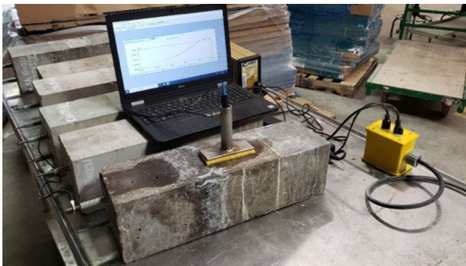
Figure 10.2: Microcell measurement set up for outdoor corrosion samples
