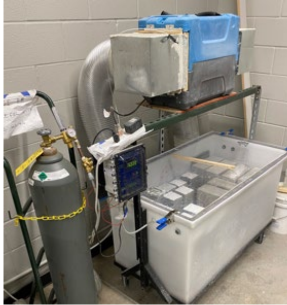
Figure 6.1: Accelerated carbonation chamber
