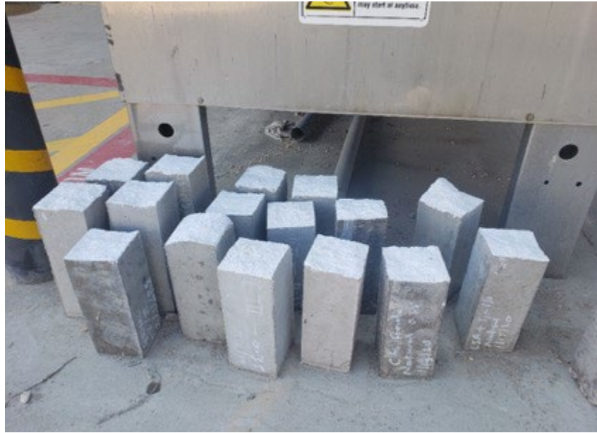
Figure 8.1: Natural unsheltered carbonation environment.
