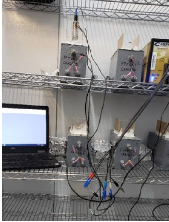
Figure 9.4: Configuration for microcell corrosion measurement
