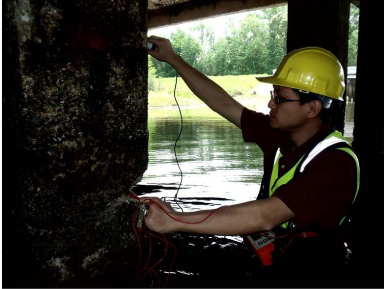
**Figure 8. Half-Cell Corrosion Potential Test.**
