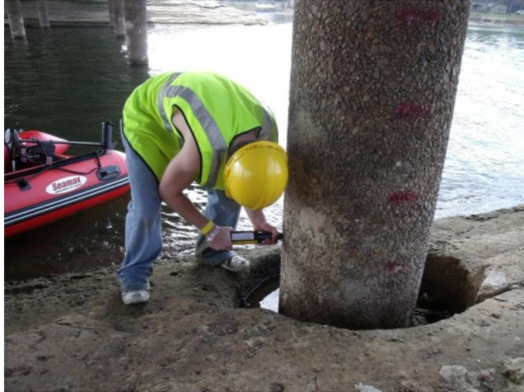
**Figure 5. Schmidt Rebound Hammer Test.**
