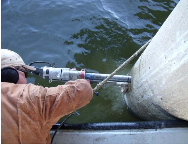
**Figure 11. Core Specimen Collection.**
