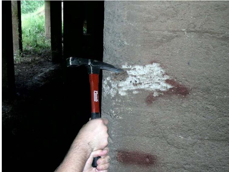
**Figure 4. Hammer Test of Concrete Condition.**
