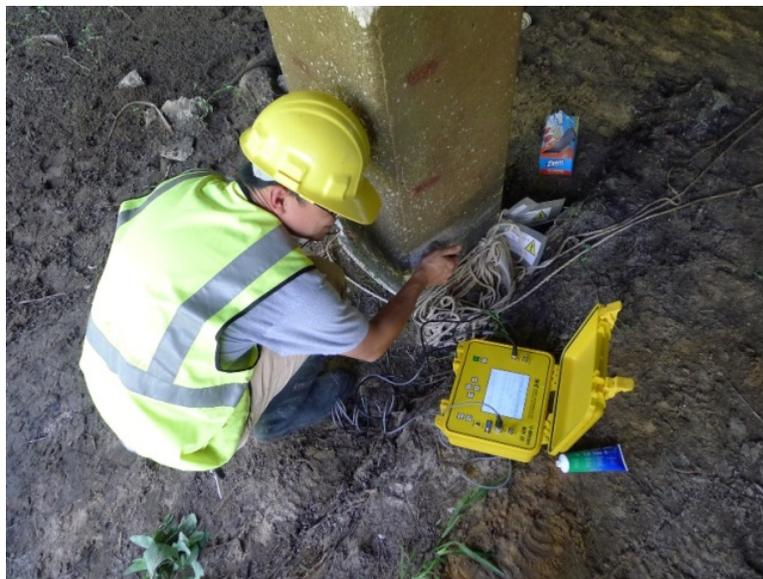
**Figure 6 Ultrasonic Pulse Velocity (UPV) Test.**
