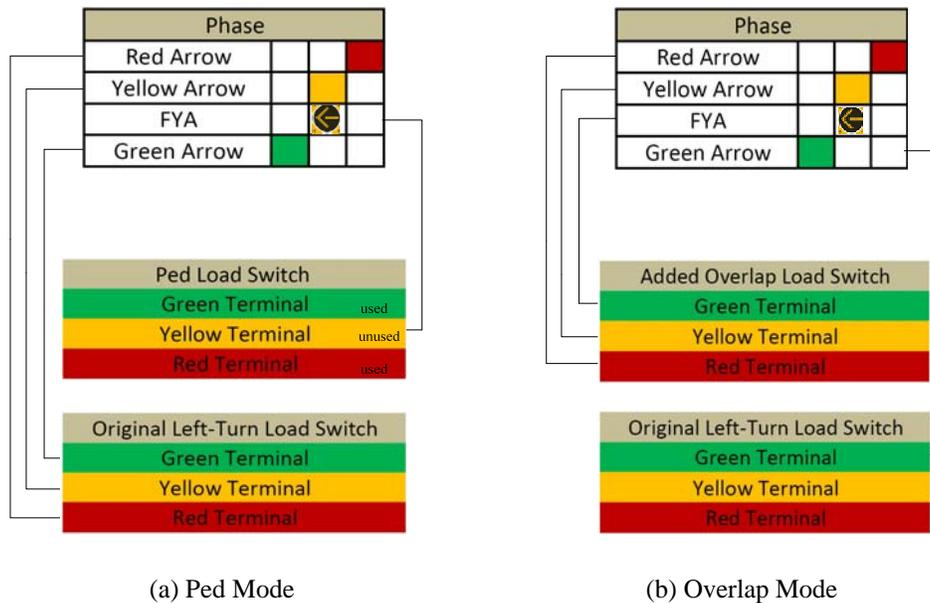
**Figure 7: Typical Overlap Programming Methods for FYA PPLT**
