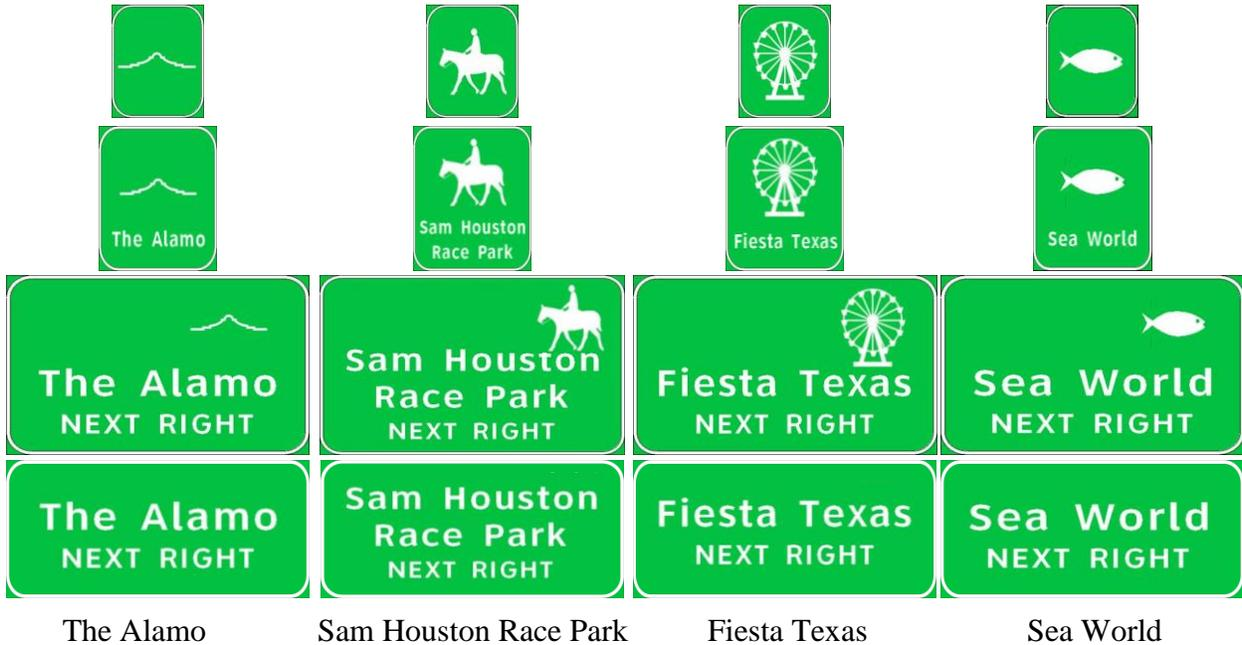
**Figure 26 Four Types of MTG Symbols**
