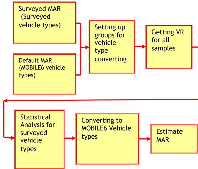
Figure 3 Modeling process for adjusting vehicle mileage accumulation rates
