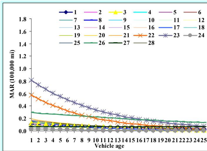
FIGURE 6 Corrected local mileage accumulation rate for El Paso area.
