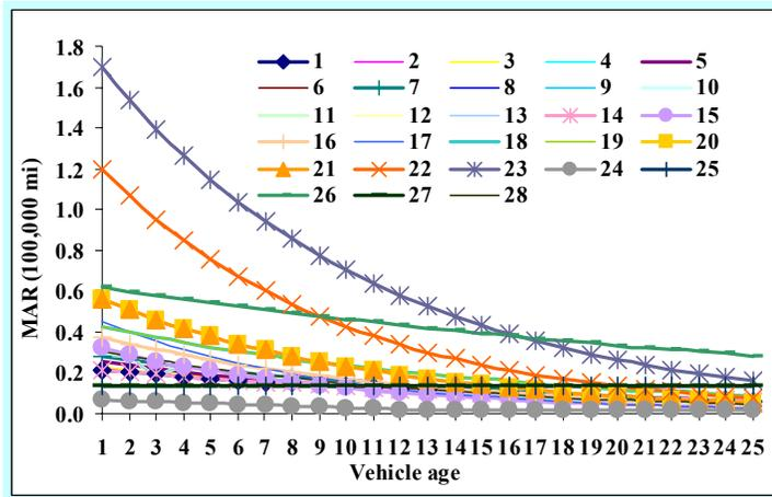
FIGURE 5 Corrected local mileage accumulation rate for Houston.
