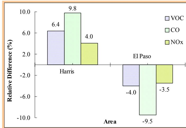
Figure 7 Relative differences of emission factors when compared adjusted mileage accumulation rates with MOBILE6 default values for Houston and El Paso.
