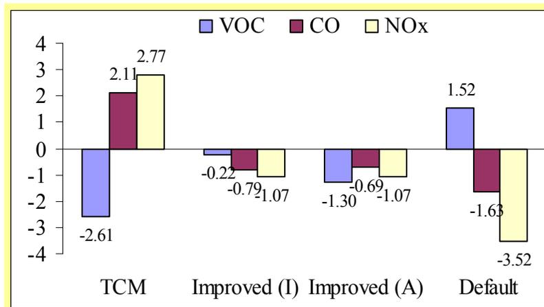
**Figure 9 Relative errors (%) for estimates of emission factors based on different scenarios.**
