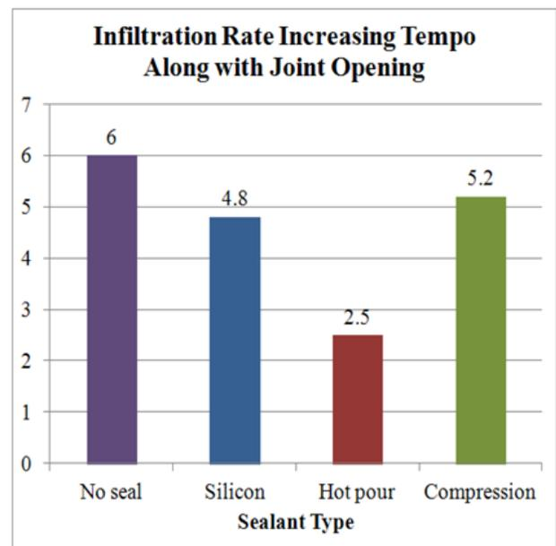
related This study emphasizes that the presence of water on the interface coupled with the effect of traffic and erodibility are the three main elements of the erosion process. The study states that the most valuable outcome of the research is the demonstration of the role of joint sealing on the service life of jointed concrete pavements.
