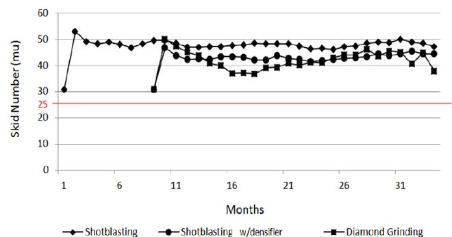
Comparison of Friction Treatments on Concrete Pavements
