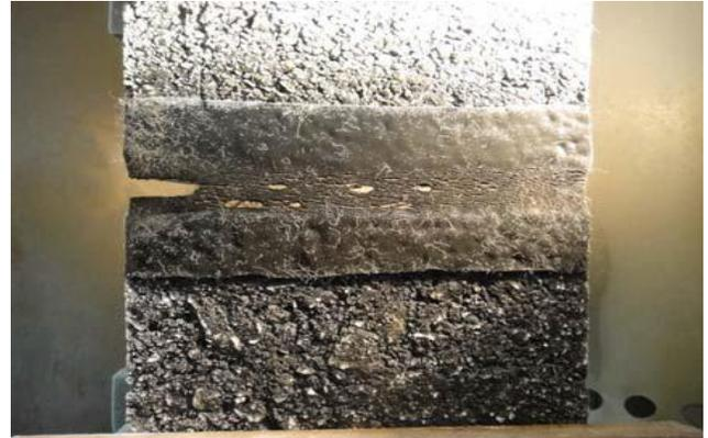
**Example of Cohesion Failure**
