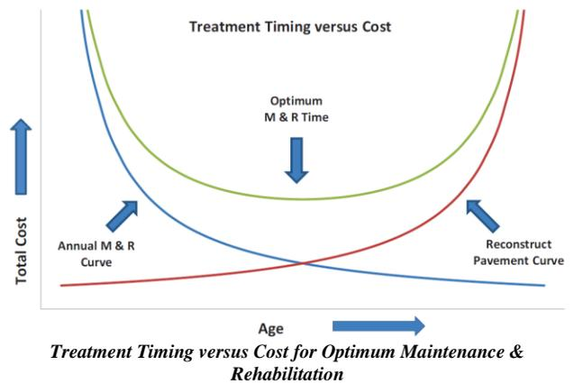
Treatment Timing versus Cost for Optimum Maintenance & Rehabilitation
