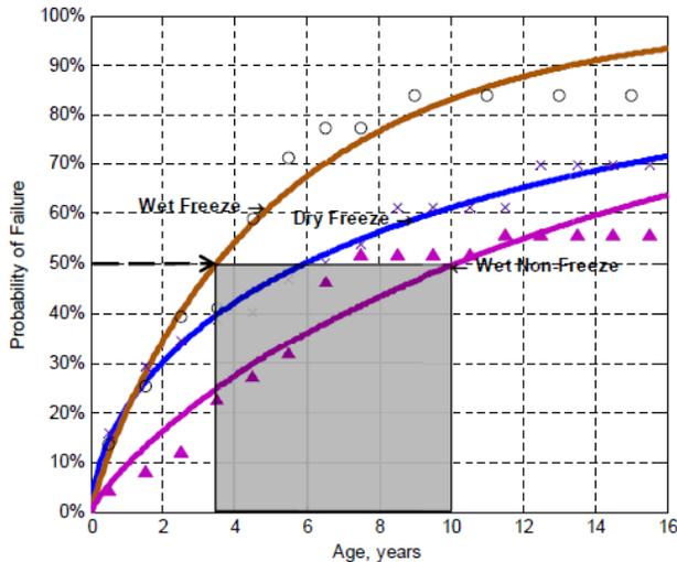
**Chip Seal Age-Failure Graph in Different Climactic Conditions**
