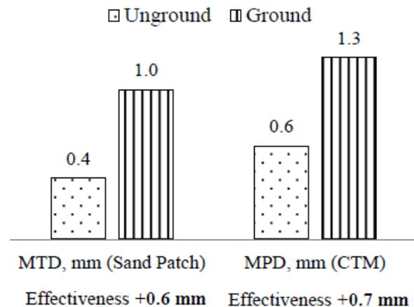
This study provides sufficient statistical evidence for the claim that grinding operations produce a relatively uniform surface in terms of macrotexture, skid, roughness and noise levels regardless of the variation in pre-existing conditions of CRC pavements. Despite this conclusion, monitoring the rate of deterioration of such pavements is recommended for assessing the overall efficiency and cost-effectiveness of surface grinding operations.
