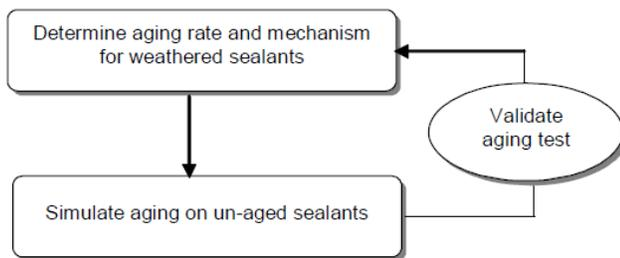
**Schematic of Aging Procedure**
