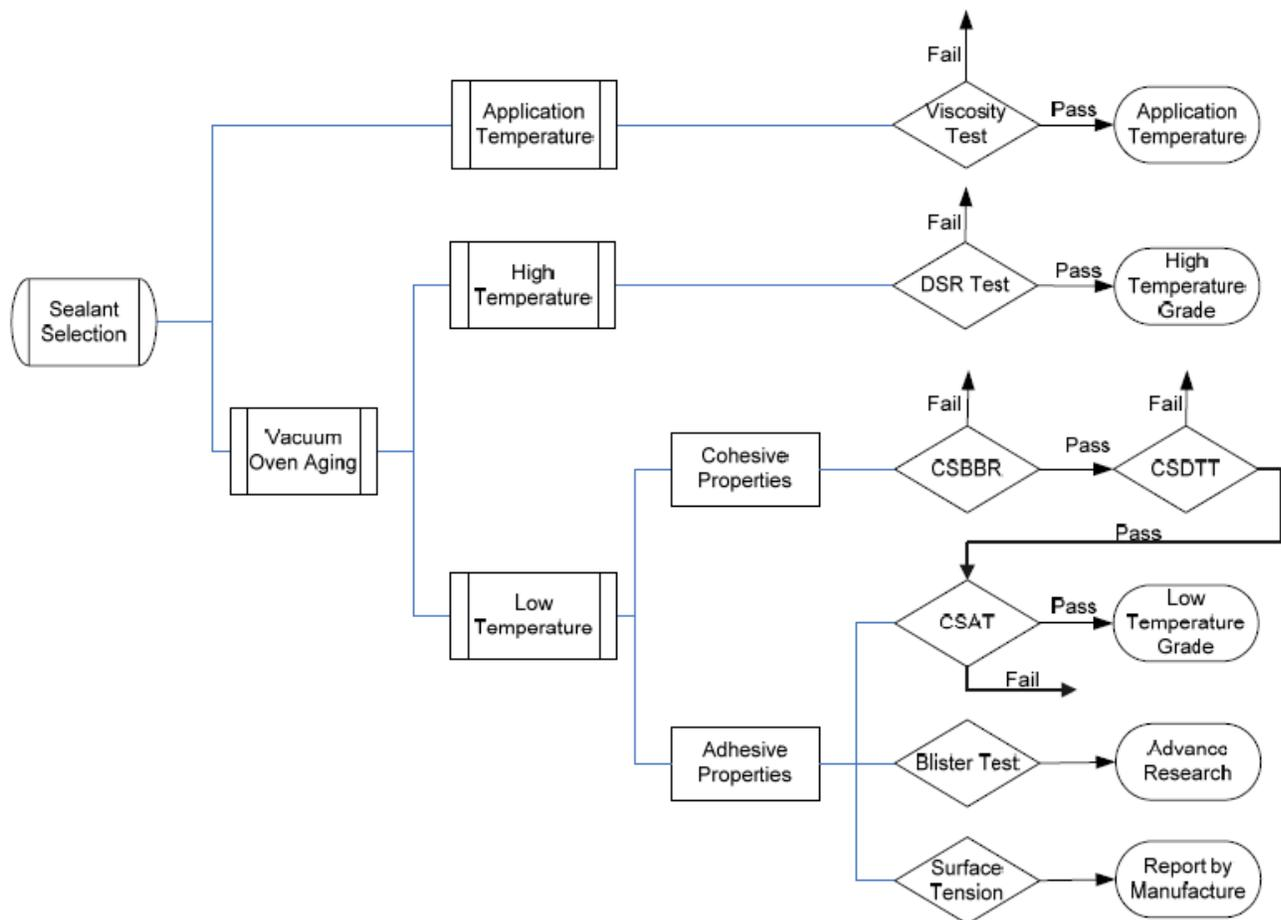
**Process for Selection of Bituminous-Based Sealants**
