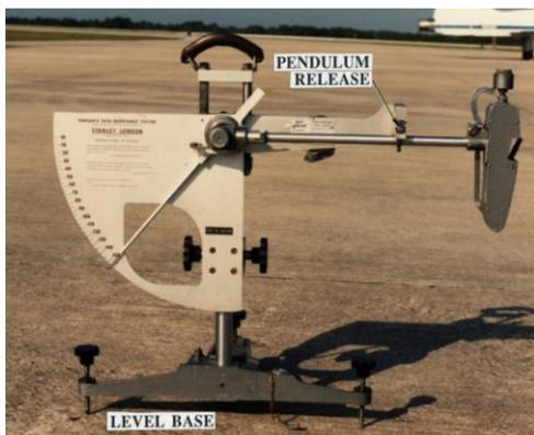
**British Pendulum Texture Measurement Device**
