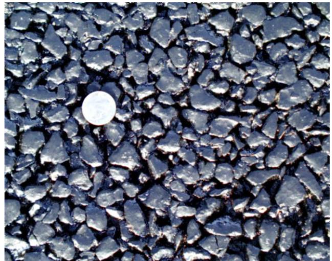
Porous PFC Mix Asphalt
