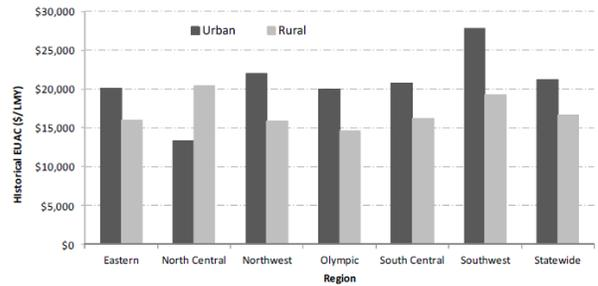
Figure 9 - EUAC for asphalt pavements within each of WSDOT's six regions.
