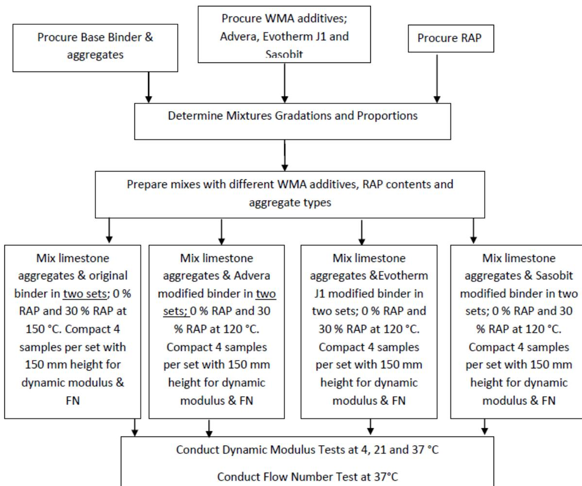
Figure 11 – Experimental set up.
