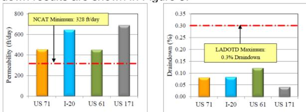
Figure 3 – Permeability and Drain down results.
