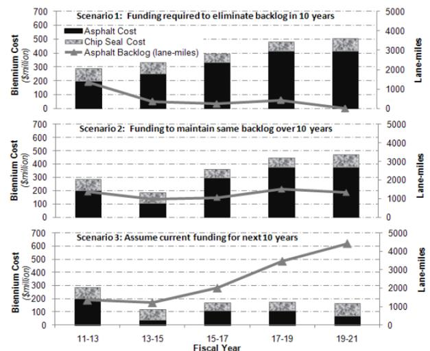
Figure 10 - The estimated cost and backlog lane-miles of WSDOT flexible pavement network under the three funding scenarios for next 10 years.
