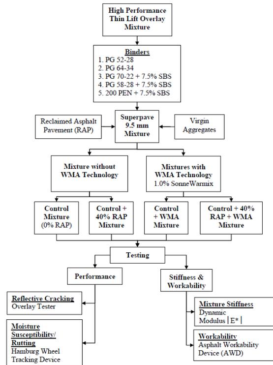
Figure 12- Experimental Set up.
