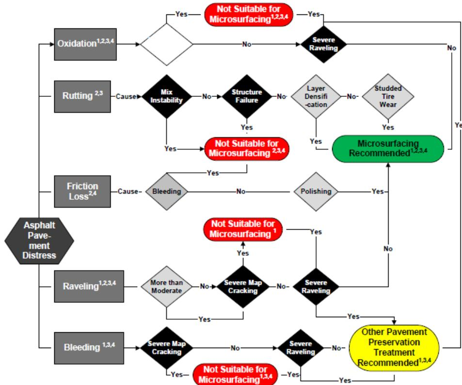
Figure 4 – Microsurfacing project selection framework for asphalt pavements.
