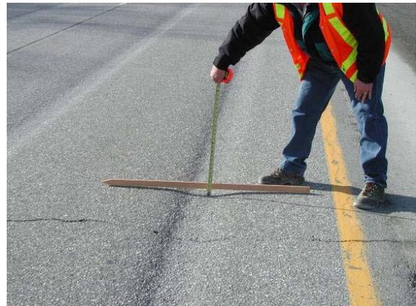
**Studded Tire Damage (wear) to HMA in Washington State (TRB 09-2205 pg. 4)**
