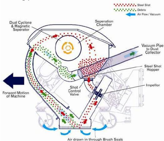
**Typical Shotblasting Apparatus Process**
