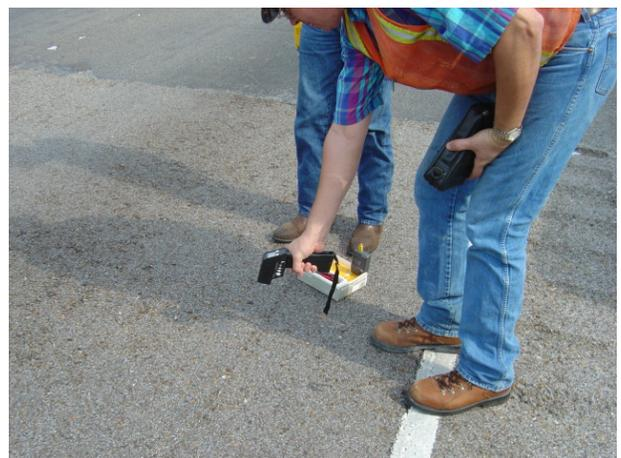
Temperature measurements for Falling Weight Deflectometer
