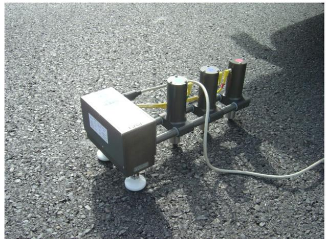
Portable Seismic Pavement Analyzer Equipment
