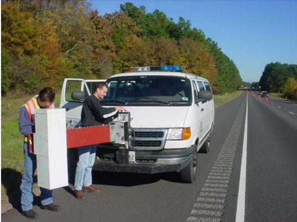
Ground Penetrating Radar Equipment
