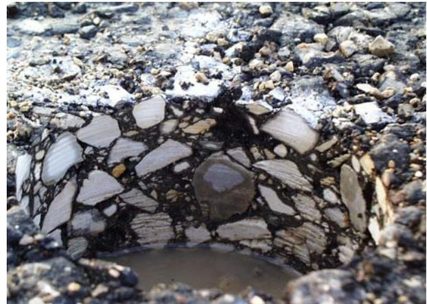
**Aggregate breakdown during coring operation**
