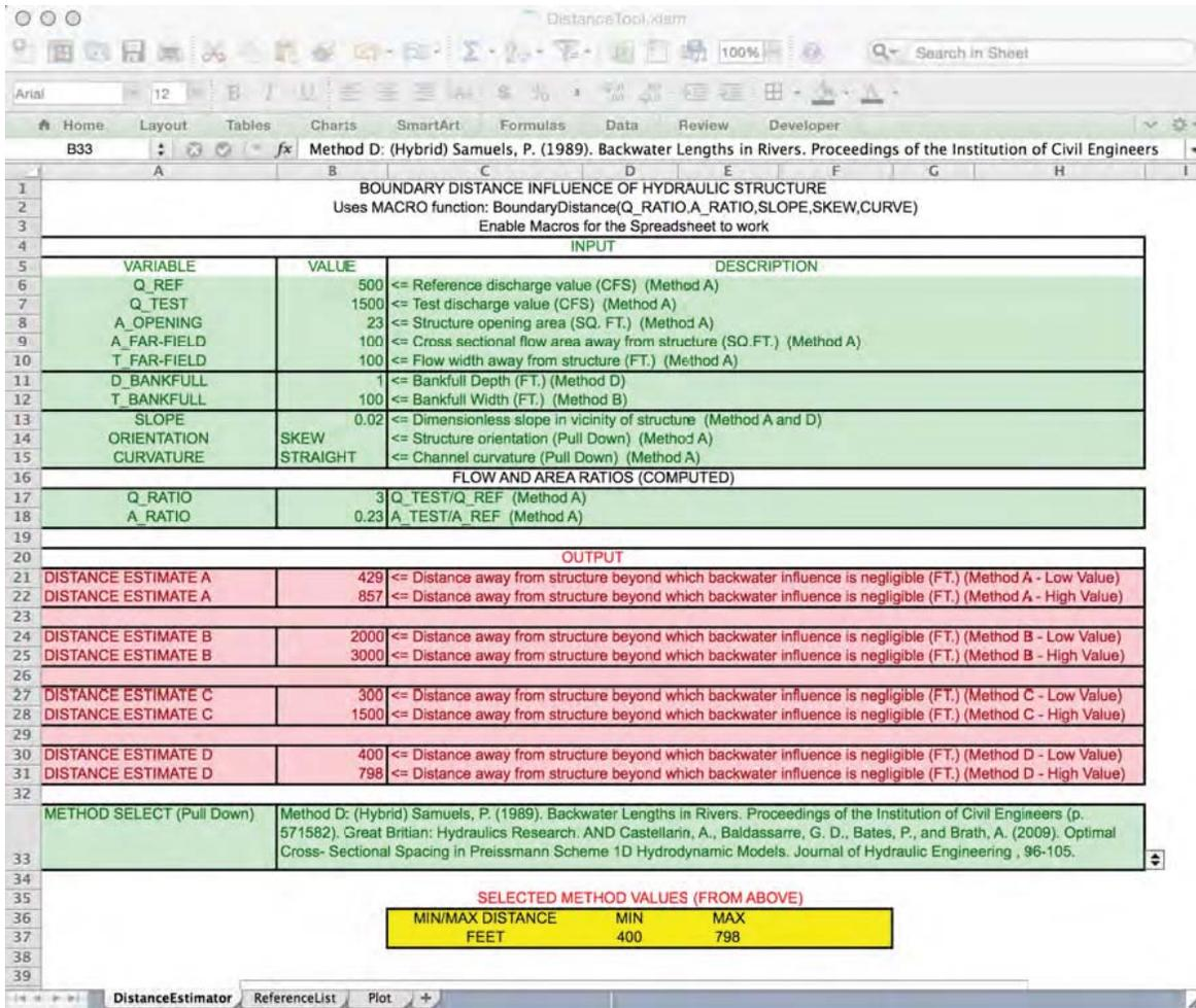
Figure 1. Screen capture of boundary distance estimation tool.
