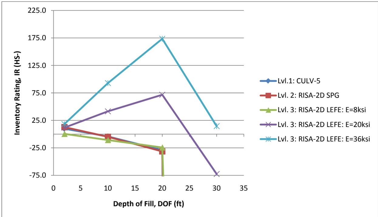
FIGURE 5.9. INVENTORY RATING VS. DEPTH OF FILL FOR MC7-1 3 7X6W2.
