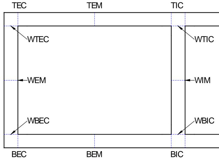
FIGURE 4.7. MOMENT CRITICAL SECTIONS FOR CULVERTS WITHOUT HAUNCHES.
