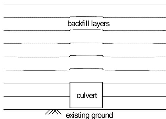
FIGURE 2.1. EMBANKMENT CULVERT
