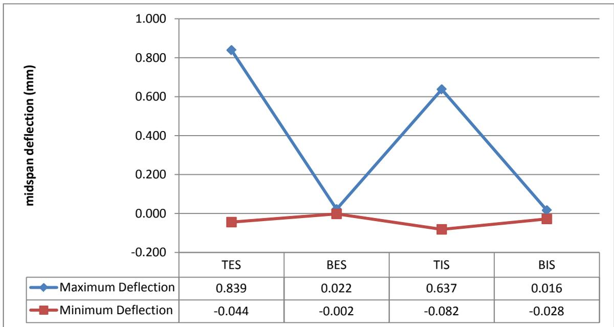
FIGURE 6.14. MEASURED DEFLECTIONS IN MILLIMETERS FOR THE SHALLOW WATER CULVERT: 2' OF FILL
