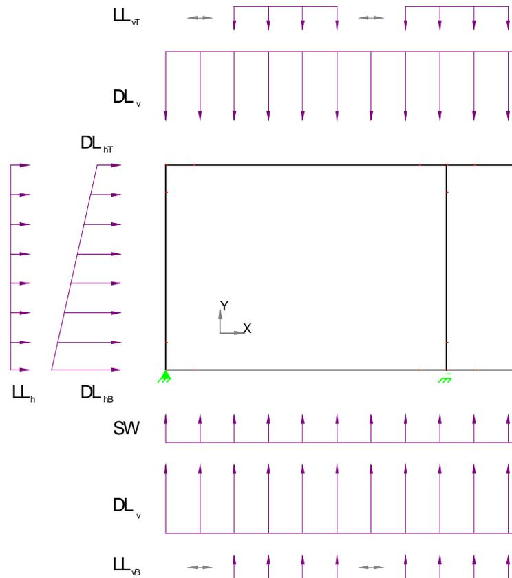
FIGURE 3.3. PREPACKAGED, TWO-DIMENSIONAL CULVERT MODELS LOADING DIAGRAM. (TXDOT, 2009).
