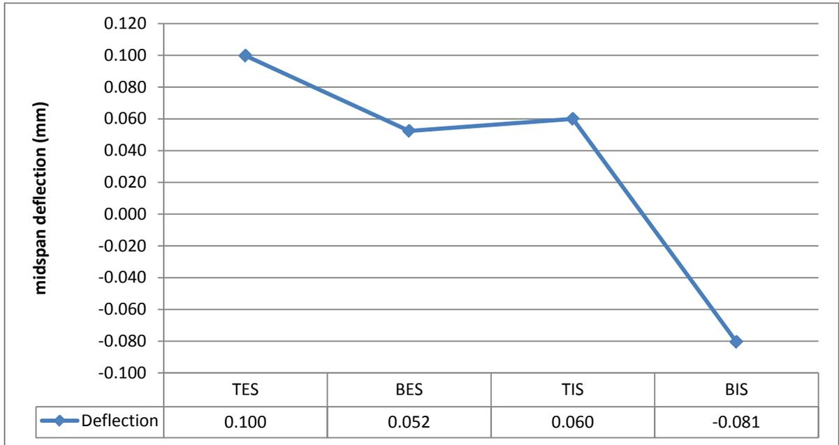
FIGURE 6.39. MEASURED DEFLECTIONS IN MILLIMETERS FOR THE SHALLOWATER CULVERT FROM 2' TO 4' OF FILL
