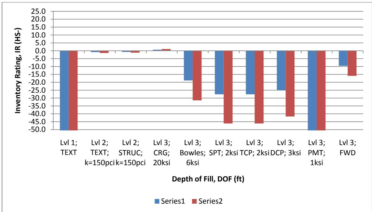
FIGURE 6.15. LOAD RATING FOR SHALLOWATER CULVERT: 4' OF FILL
