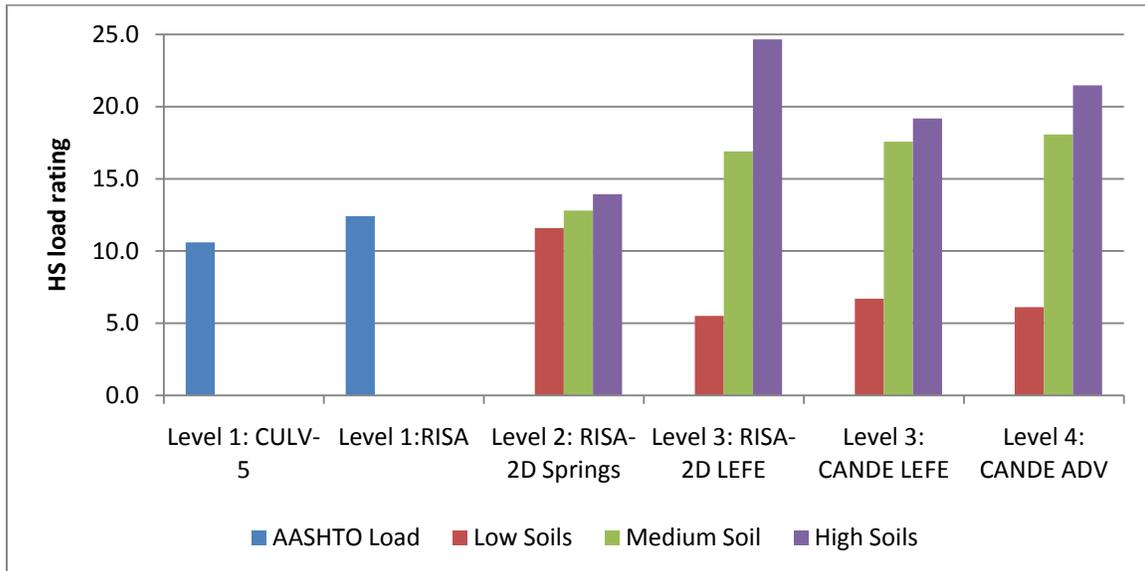
FIGURE 3.11. LOAD RATING COMPARISON OF FULL SCALE CULVERT
