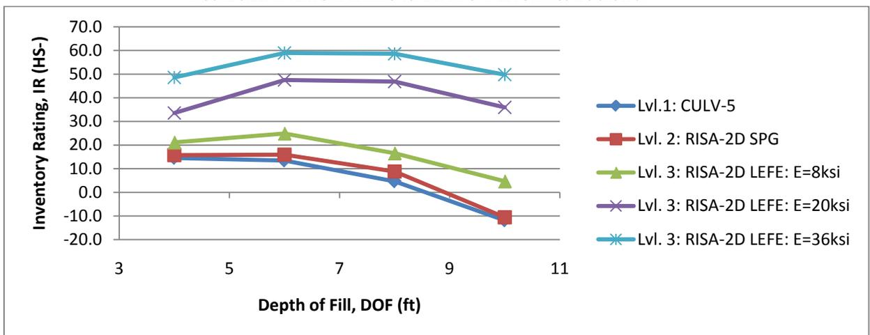
FIGURE 5.12. INVENTORY RATING VS. DEPTH OF FILL FOR MBC-5-34 5 9X8W0.
