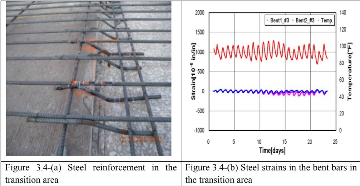
Figure 3.5-(a) compares steel strains at longitudinal steel and bent bar at location 2, which is 4 in. north from the intersection between normal overlay and transition area. Very little variation was observed in the steel strain in the bent bar, whereas quite large variations in steel strain, up to 1,300  $\mu\epsilon$  a day, were observed in the longitudinal steel.
