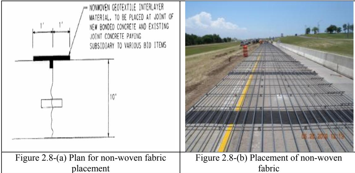
Figure 2.8-(a) Plan for non-woven fabric placement
