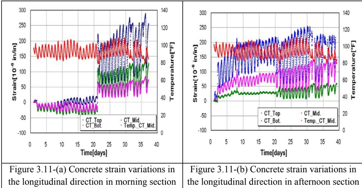
Figure 3.11-(a) Concrete strain variations in the longitudinal direction in morning section
