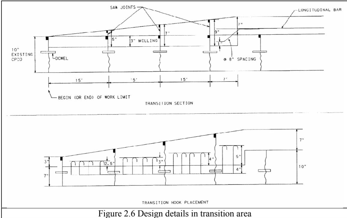
Figure 2.6 Design details in transition area
