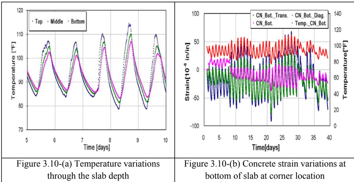
Figure 3.10-(b) shows the concrete strains at the bottom of the 7 in. CRCP at the corner in three directions in the afternoon section where fabric was removed. Compared with Figure 3.9-(b), the same trend is observed and it appears that the interface bond condition doesn't affect the bottom concrete strains at the corner.
