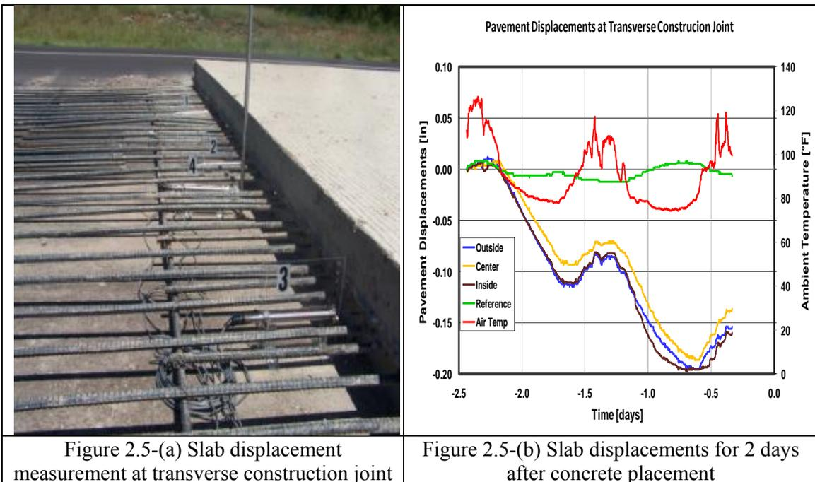
Figure 2.5-(a) Slab displacement measurement at transverse construction joint
