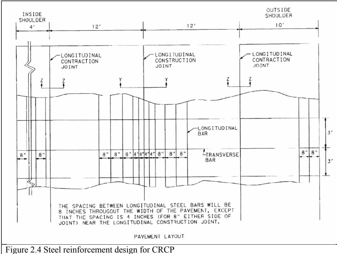
Figure 2.4 Steel reinforcement design for CRCP
