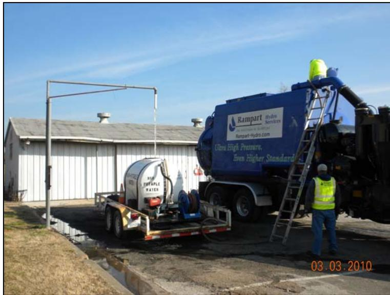
**FIG 31.** Use of a water trailer when insufficient overhead clearance exists for the UHP water cutter truck.
