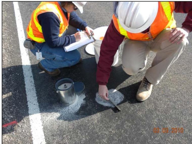
**FIG 21.** Sand patch test (TEX-436-A) to measure pavement texture.
