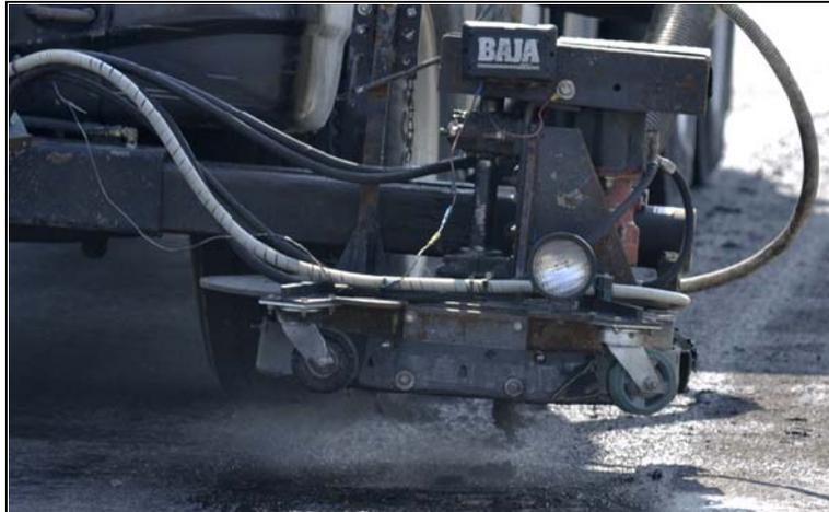
**FIG 11.** The BlasterVac cutting head. *Image courtesy TTI Visual Media.*
