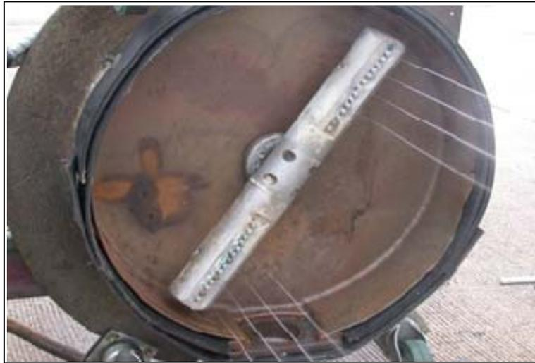
**FIG 8.** The rotating spray bar and nozzle configuration.
