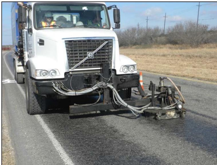
**FIG 7.** The UHP water cutter system.
