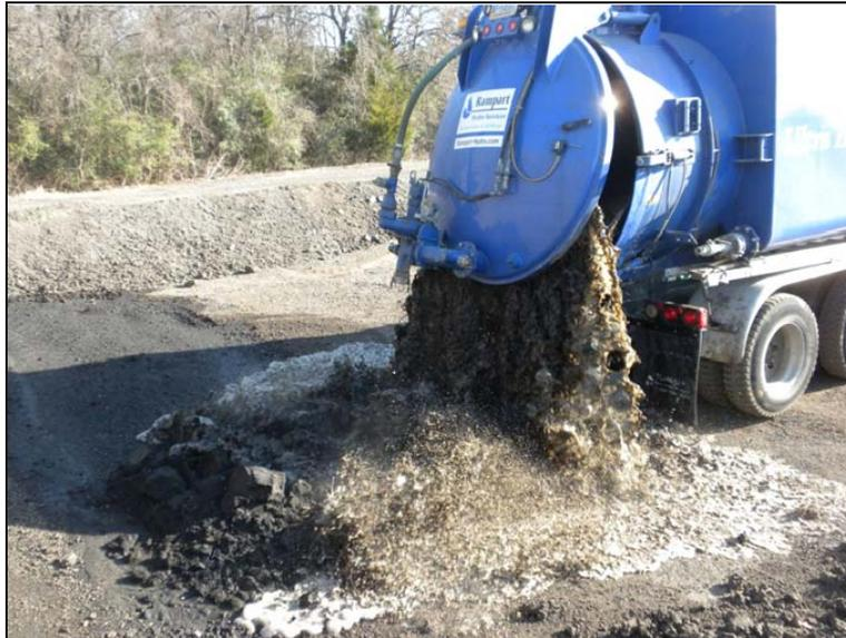
FIG 12. Debris tank and dump, Rampart BlasterVac truck.
