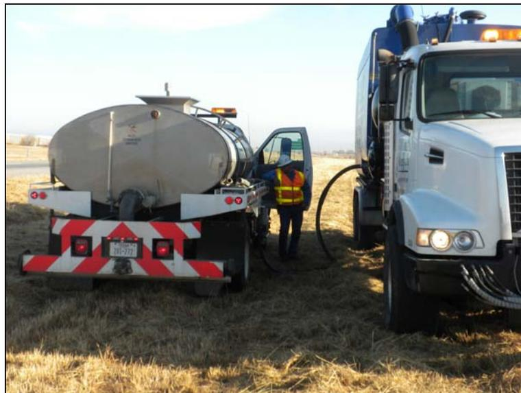
**FIG 13.** Filling the Rampart BlasterVac truck on the roadside using a support water truck.
