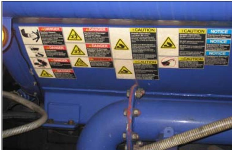
**FIG 17.** UHP water cutter equipment safety warnings.
