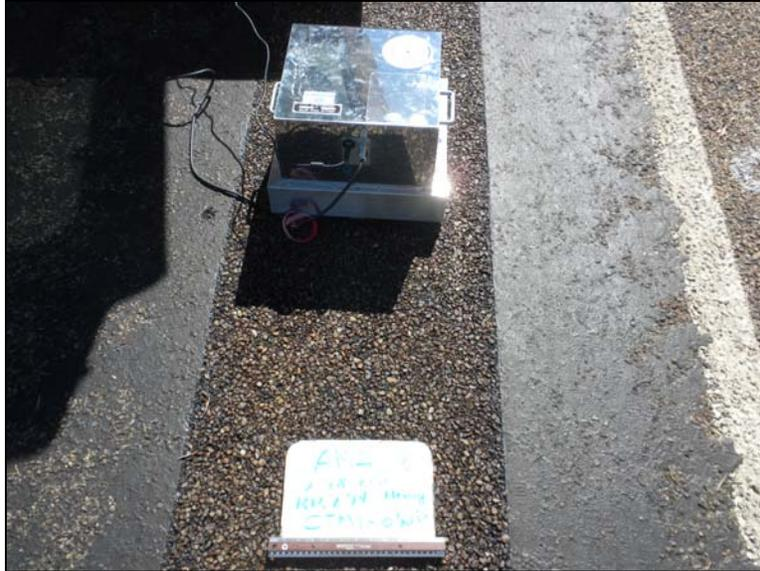
**FIG 22.** Circular Track Meter (CTM) test (ASTM E-2157) to measure pavement texture.
