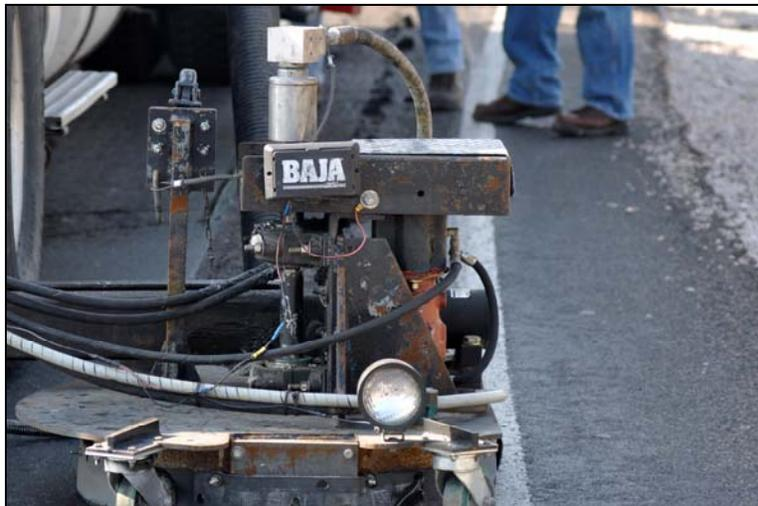
**FIG 33.** Rotational speed for the spray bar influences UHP water cutter effectiveness. *Image courtesy TTI Visual Media.*
