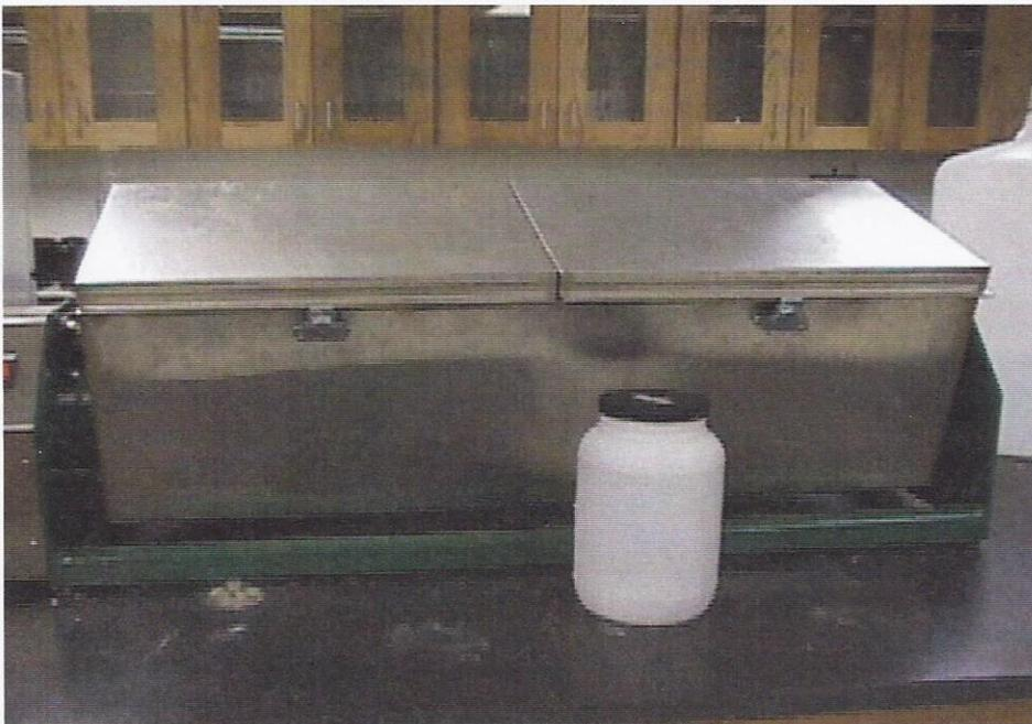
**Figure 2: Extraction Vessel and Tumbler**
