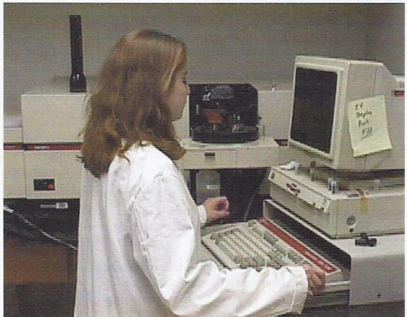
Figure 1. Graphite Furnace Atomic Absorption Spectrometer
