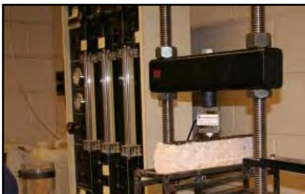
**Figure 3.5** Flexural Strength Testing Arrangement
