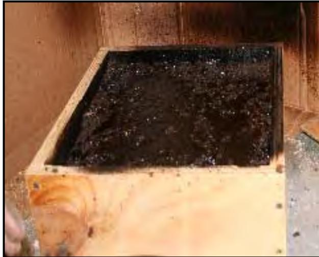
**Figure 3.3** Prime Coated Specimen after Curing
