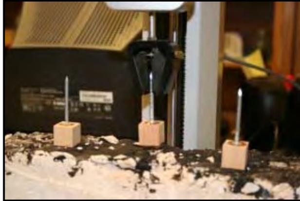
**Figure 3.6** Pullout Strength Testing Arrangement
