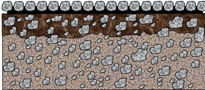
**Figure 2.2** Schematic of a Typical One-Course AST.
