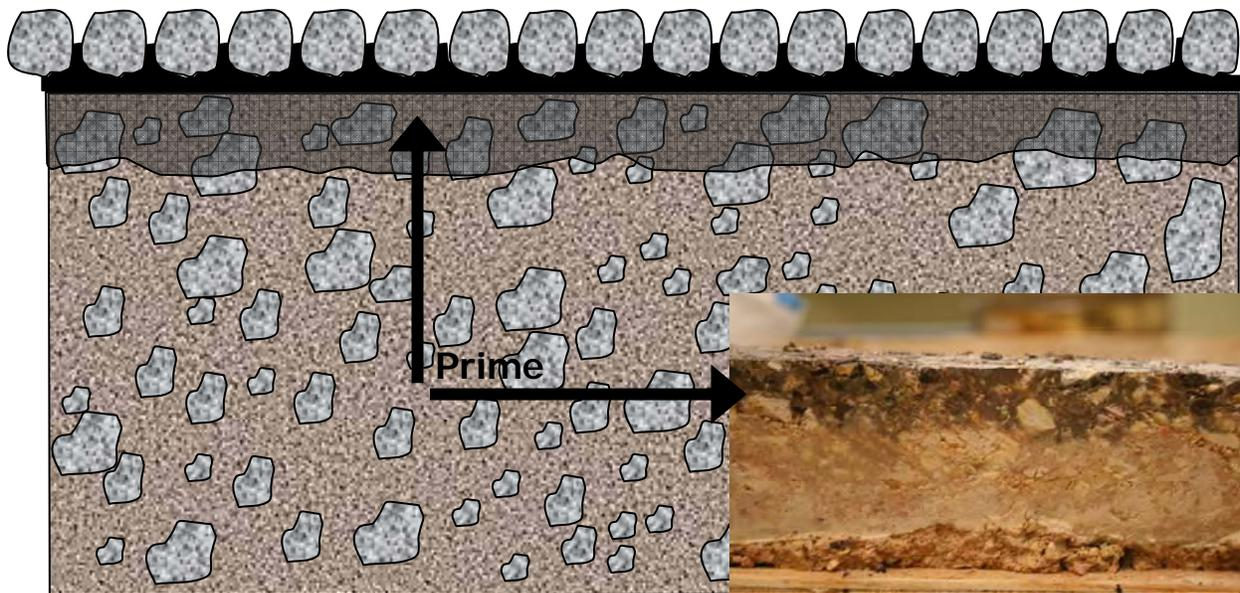
**Figure 4.5** Schematic of Prime Coat Penetration into Base
