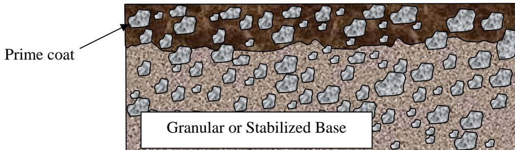
**Figure 2.1** Schematic of Prime Coat Penetration into Base Layer
