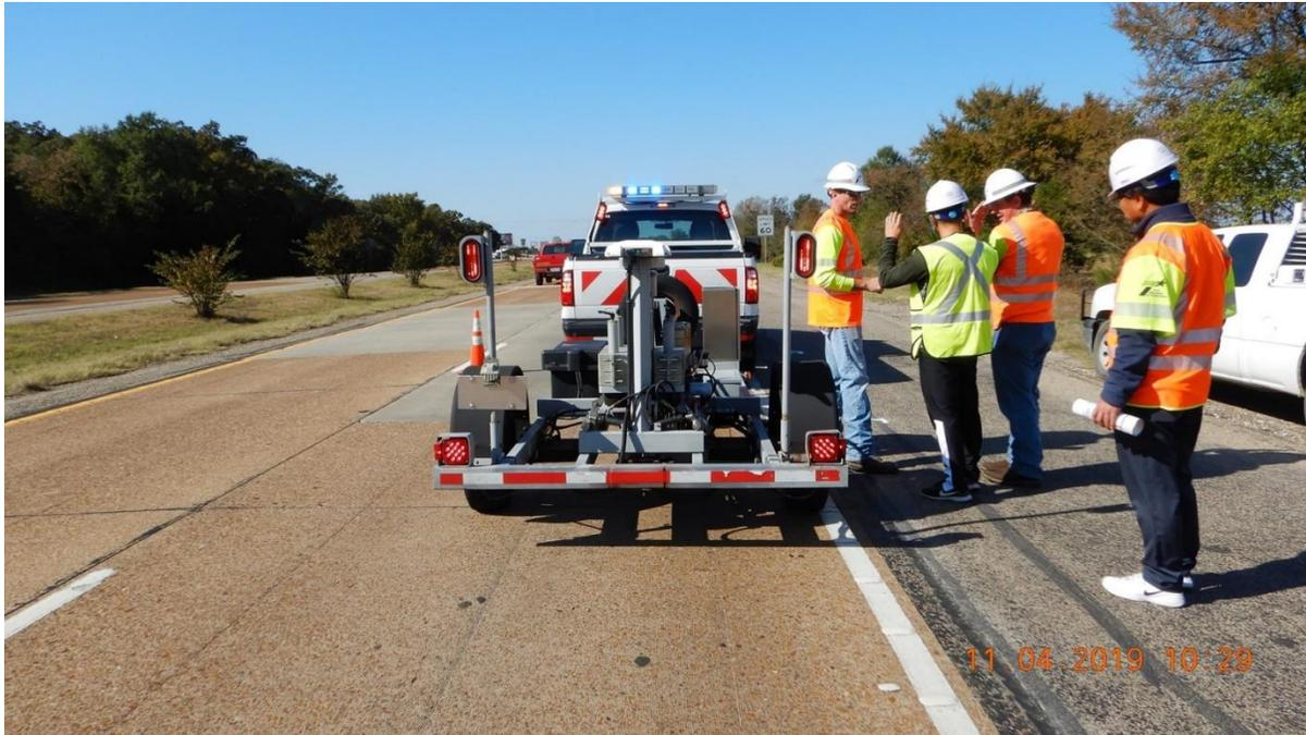
**Figure 7 FWD testing on existing CPCD**
