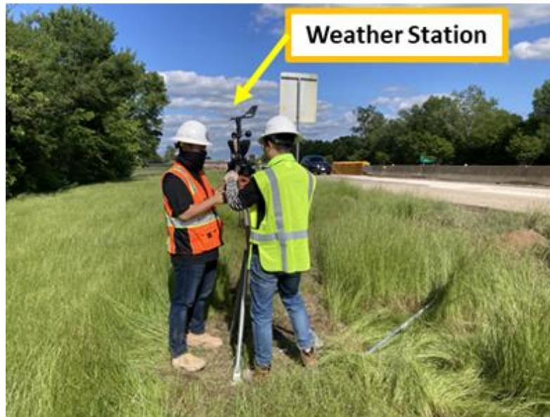
Figure 28 Davis weather station installed in field test site
