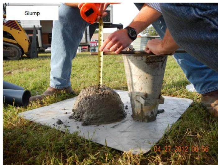
Figure 3.8 Concrete Slump Test
