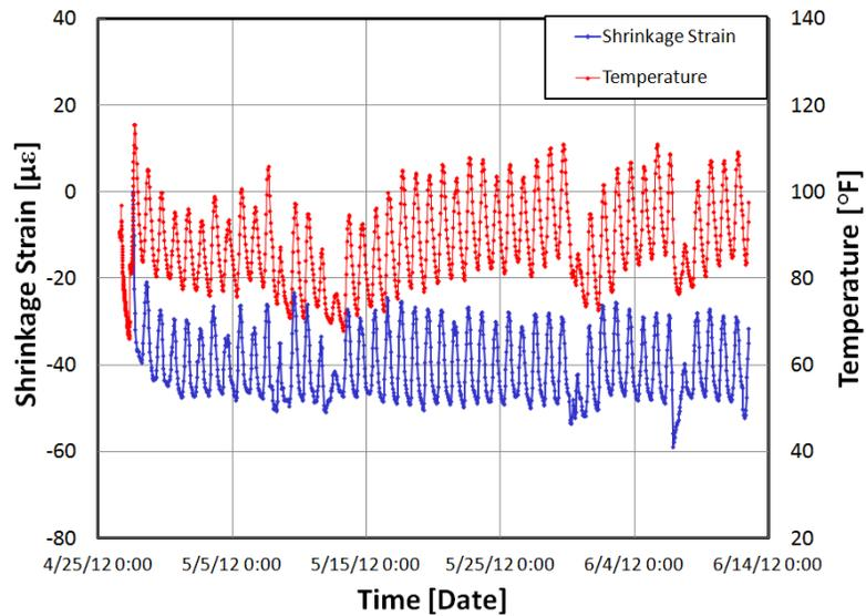
**Figure 3.11 Concrete Drying Shrinkage Evaluated from PNC and INC**
