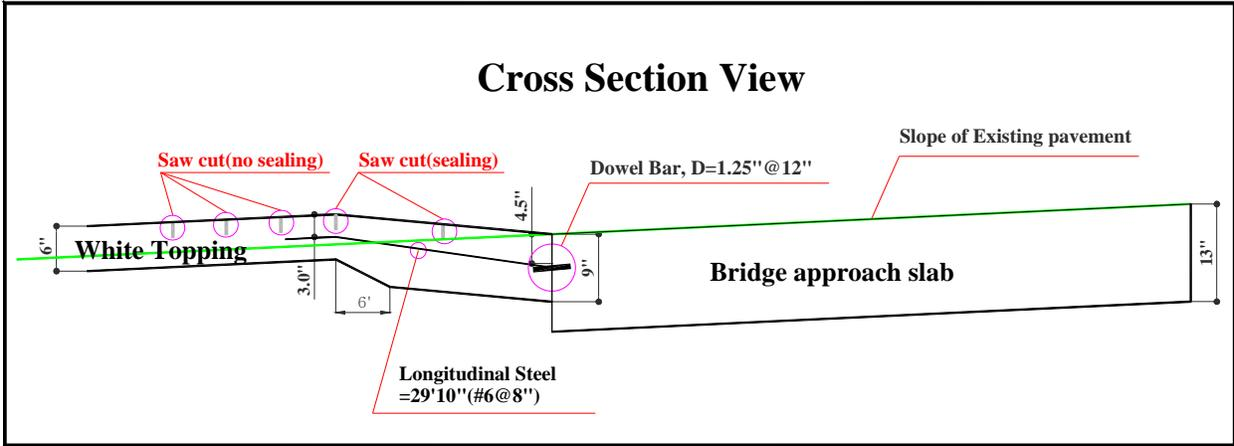
**Figure 2.8 Transition Section Design (cross section view)**
