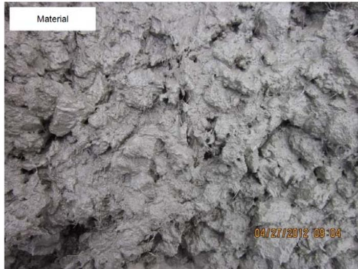
**Figure 3.9 Fiber in Concrete**
