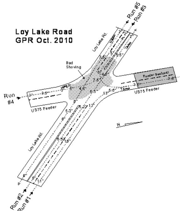
**Figure 2.3 Existing Asphalt Thickness (Loy Lake Road)**
