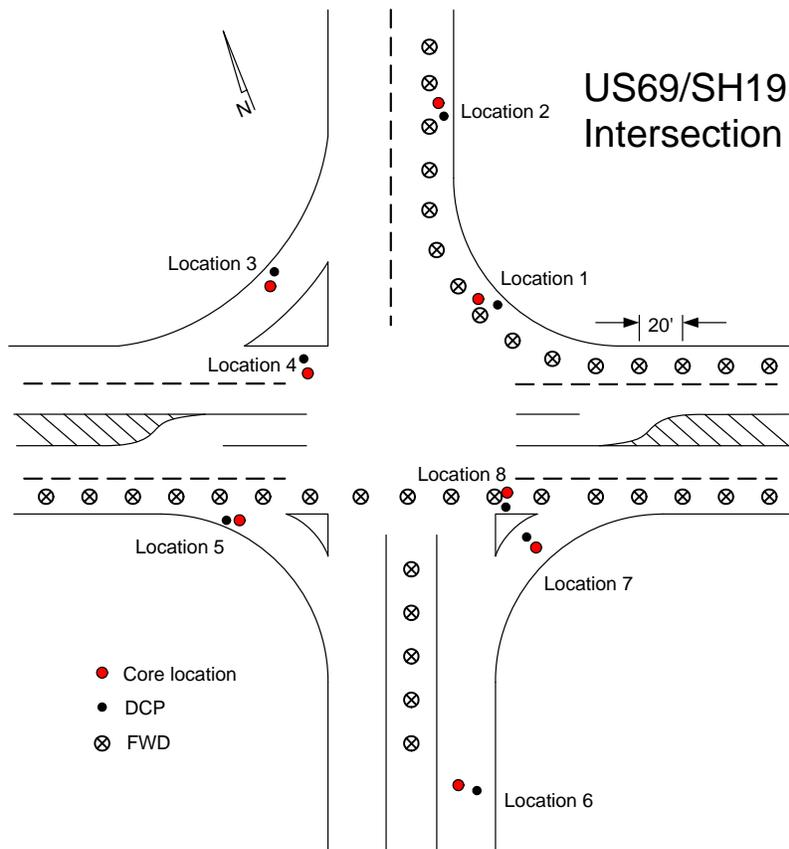
**Figure 2.11 Location for Coring, DCP and FWD**
