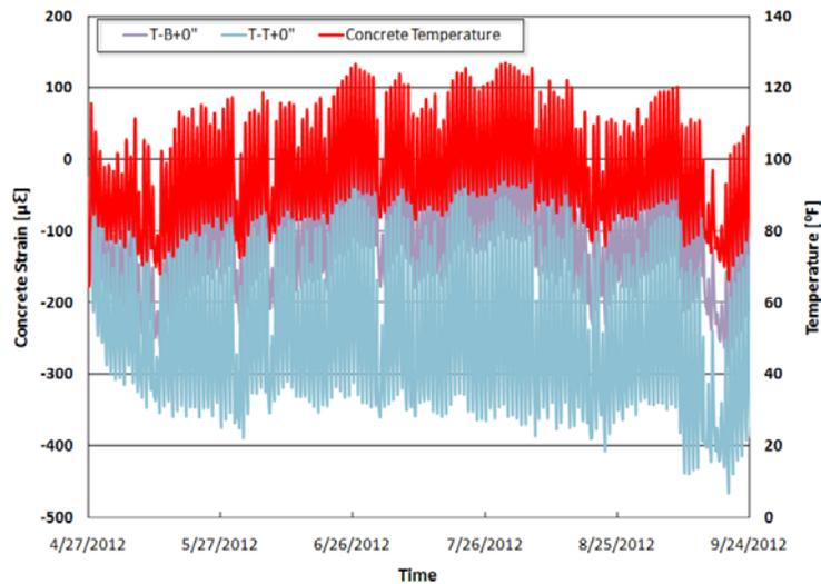
(c) Top and Bottom Concrete Strain in the Transverse Direction Near Free Edge (from VWSGs)
