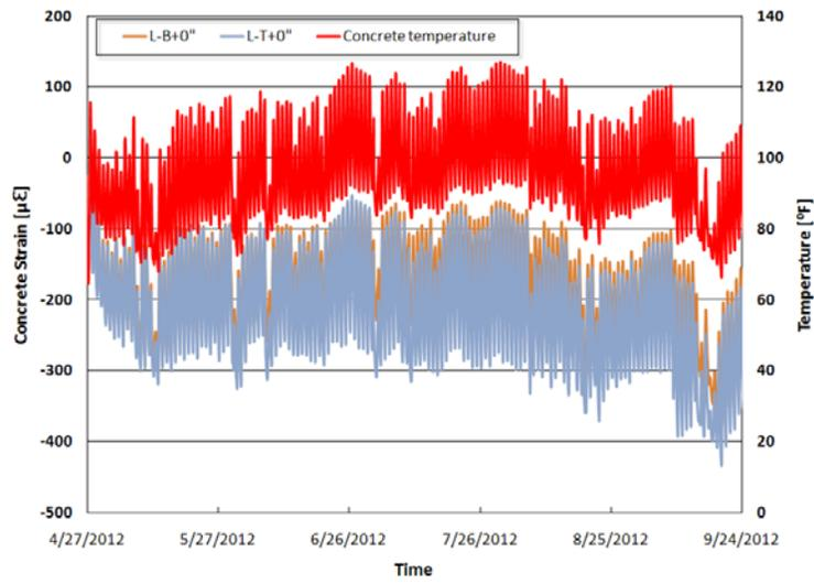
(a) Top and Bottom Concrete Strain in the Longitudinal Direction at the Center of Slab Between Joint #2 and 3
