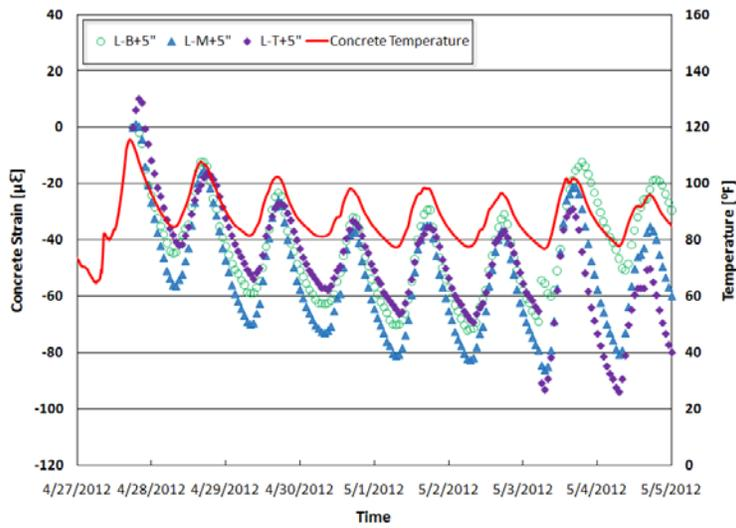
(a) Concrete Strain Variation at Top, Middle, and Bottom in Longitudinal Direction Near Joint #1 (measured by electric strain gages)
