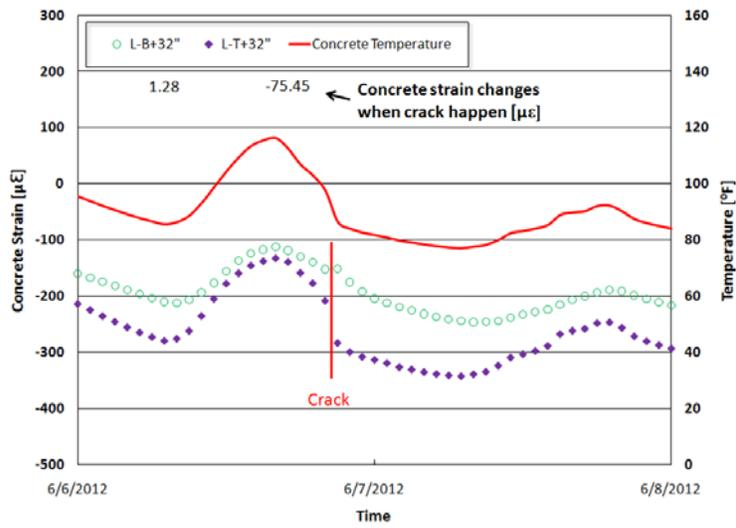
(a) Concrete Strain Changes Near Joint #3 When the Second Crack Was Detected (Measured from VWSGs)
