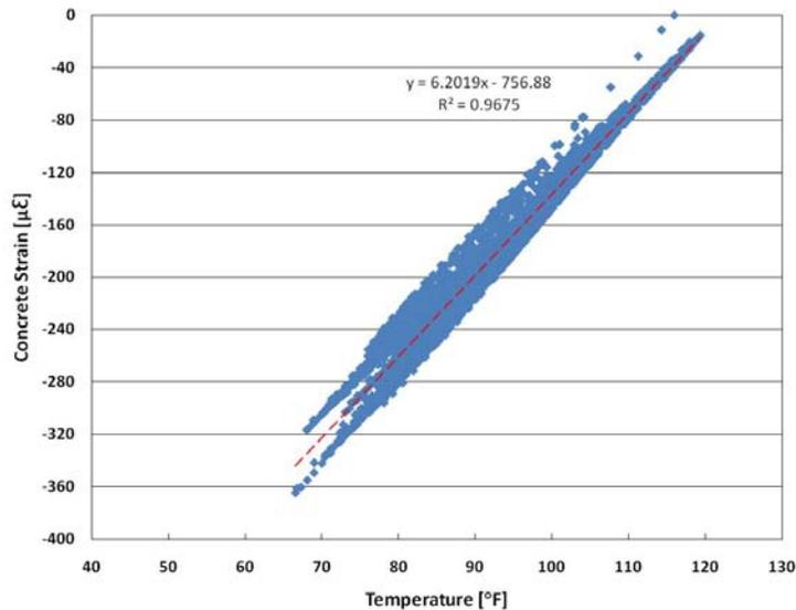
**Figure 3.10 Concrete Coefficient of Thermal Expansion (CoTE)**
