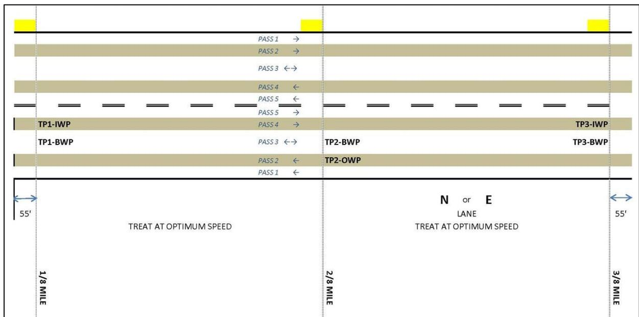
FIGURE 2.8. Test Site Layout for Production Sections
