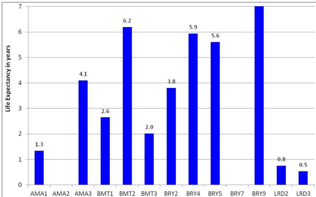
**FIGURE 4.8.** Treatment Life Expectancy, in Years, Predicted Based on Pavement Friction Estimated From SN Data
