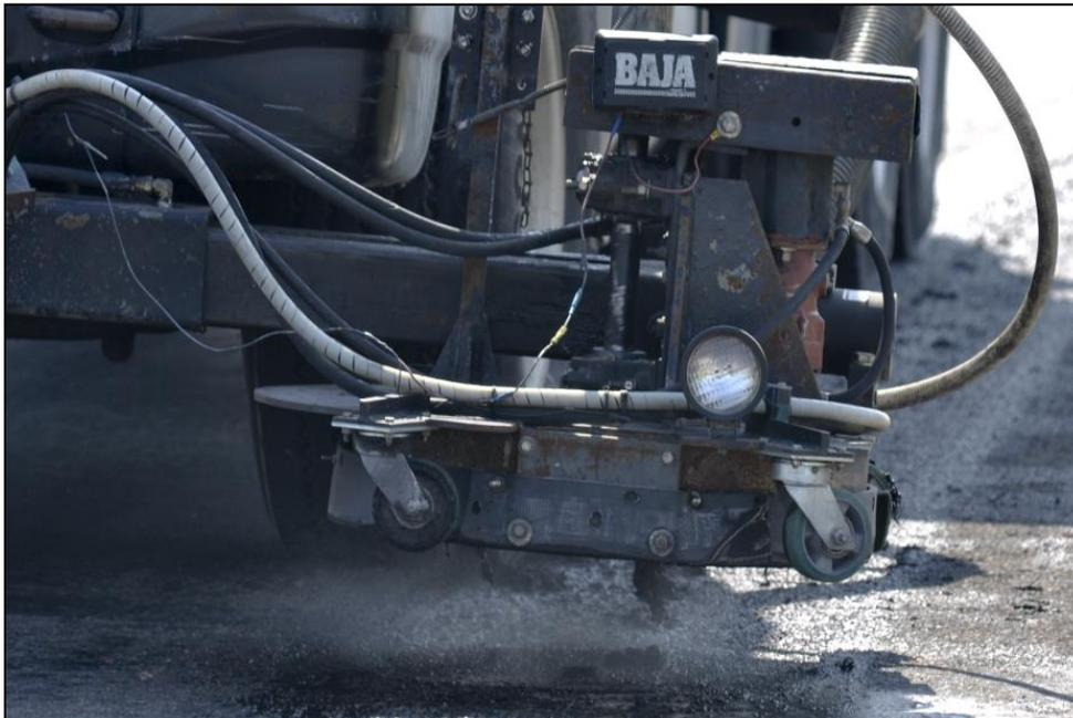
**FIGURE 5.4.** *Cutting Head, Rampart BlasterVac*
