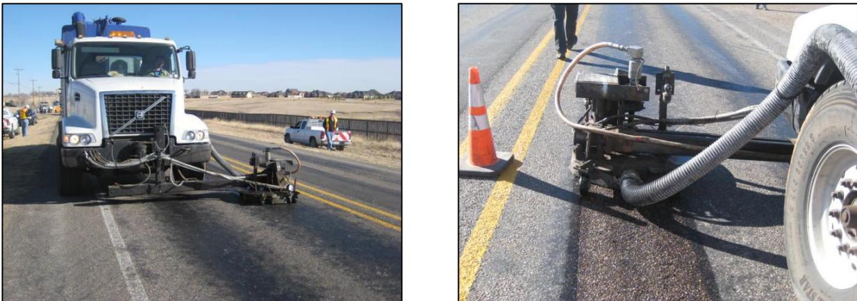
**FIGURE 1.1** UHP Water Cutter With Fixed Cutting Head Attachment
