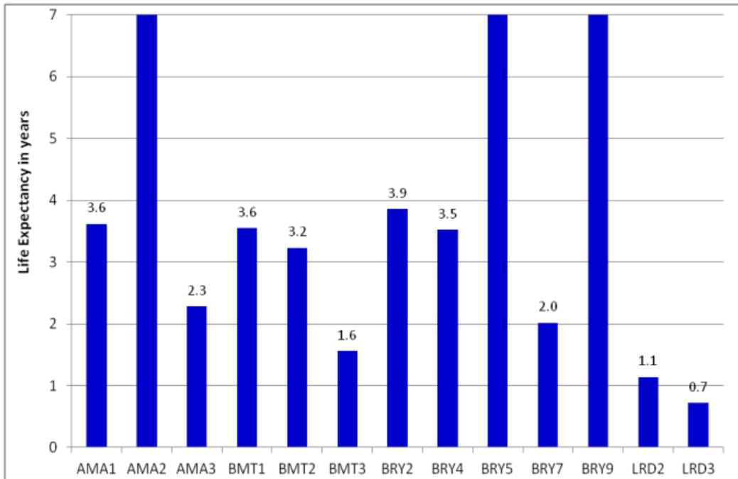
**FIGURE 4.7.** Treatment Life Expectancy, In Years, Predicted Based On Pavement Texture Estimated From SP Mean Texture Depth Data
