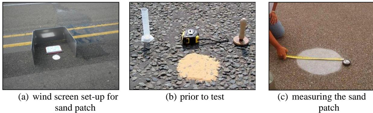
**FIGURE 2.10.** Sand Patch Test Method to Measure Pavement Surface Texture Depth
