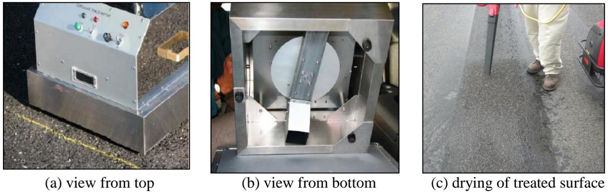
**FIGURE 2.9.** ASTM E-2157 Circular Texture Meter to Measure Pavement Macrotexture
