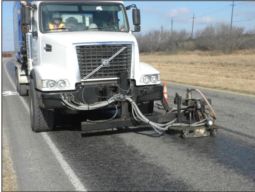
**FIGURE 2.3.** Cutting Head, Rampart BlasterVac Truck
