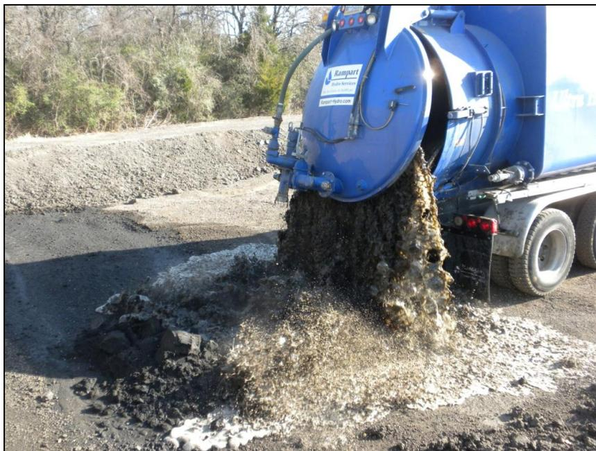
**FIGURE 2.5.** Debris Tank and Dump, Rampart BlasterVac Truck
