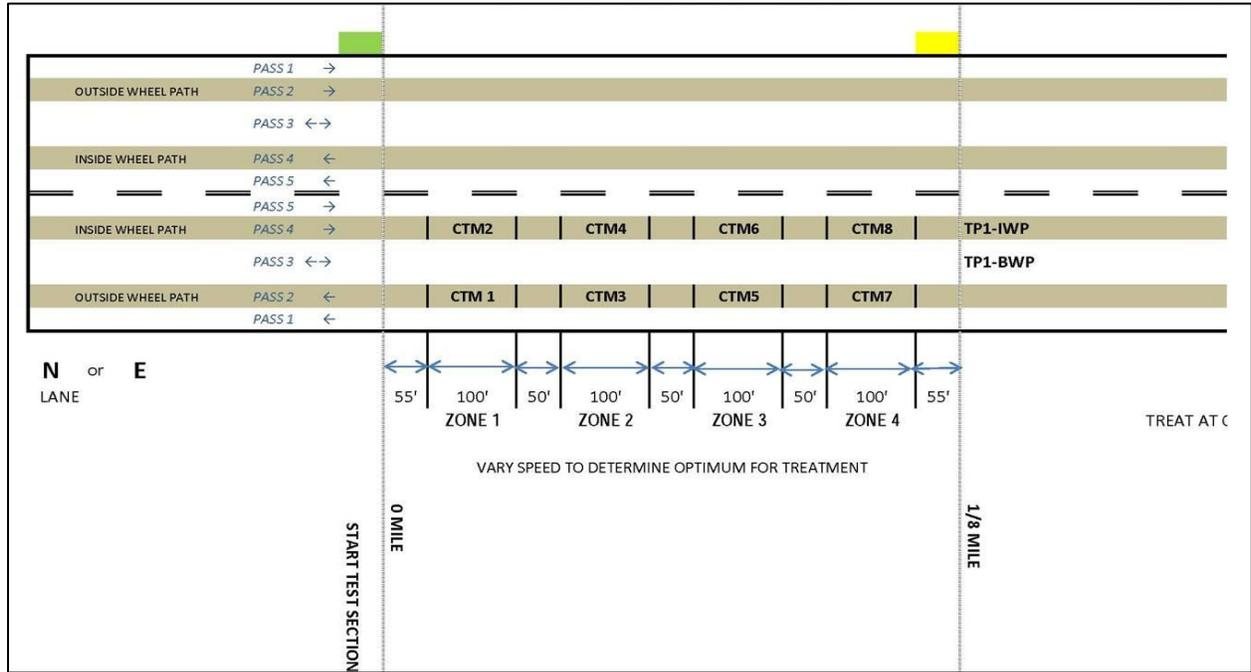
FIGURE 2.7. Test Site Layout for Speed Sections
