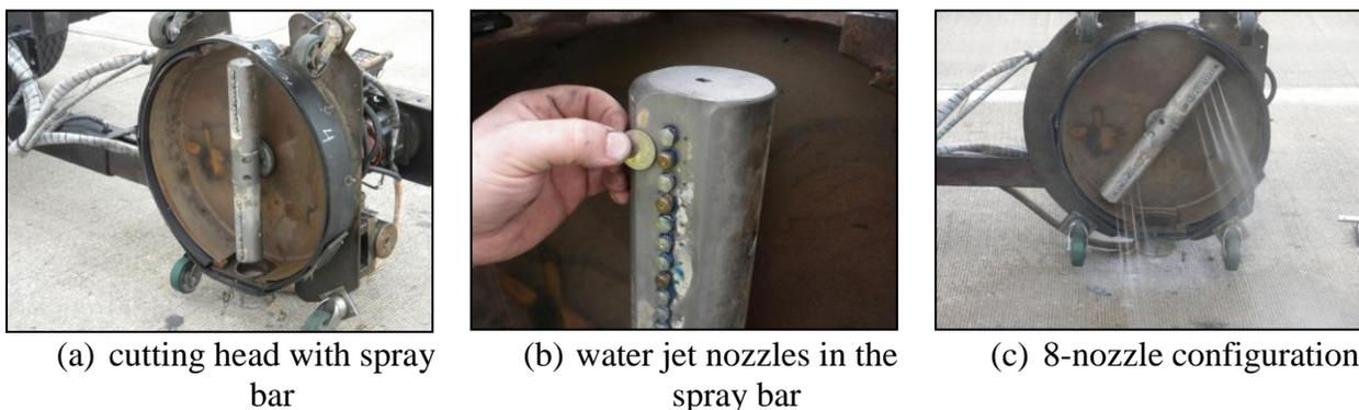
(a) cutting head with spray bar
