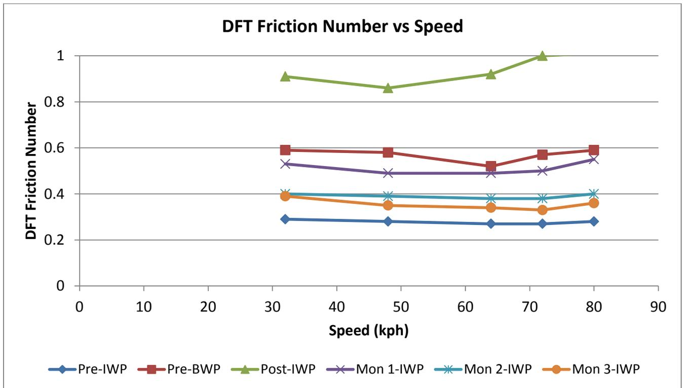
**Dynamic Friction Test (DFT) Friction Number Data for TP 2**
