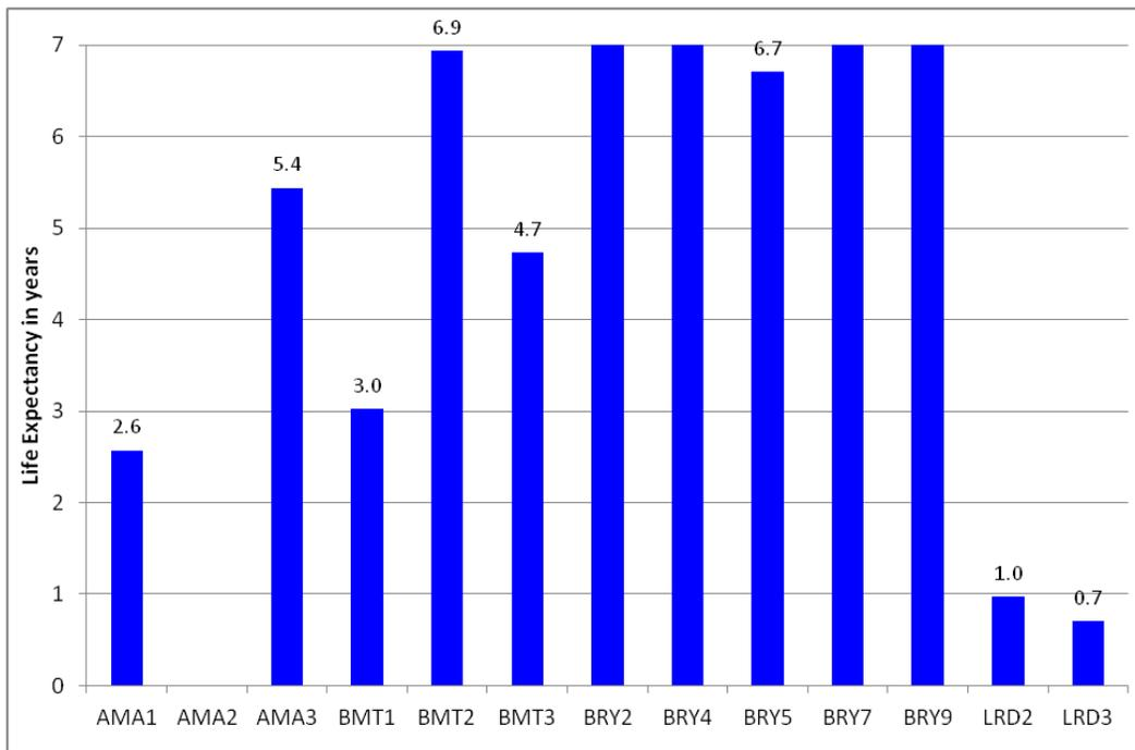
**FIGURE 4.9.** Treatment Life Expectancy, in Years, Predicted Based on Pavement Friction Estimated from DFT FN Data
