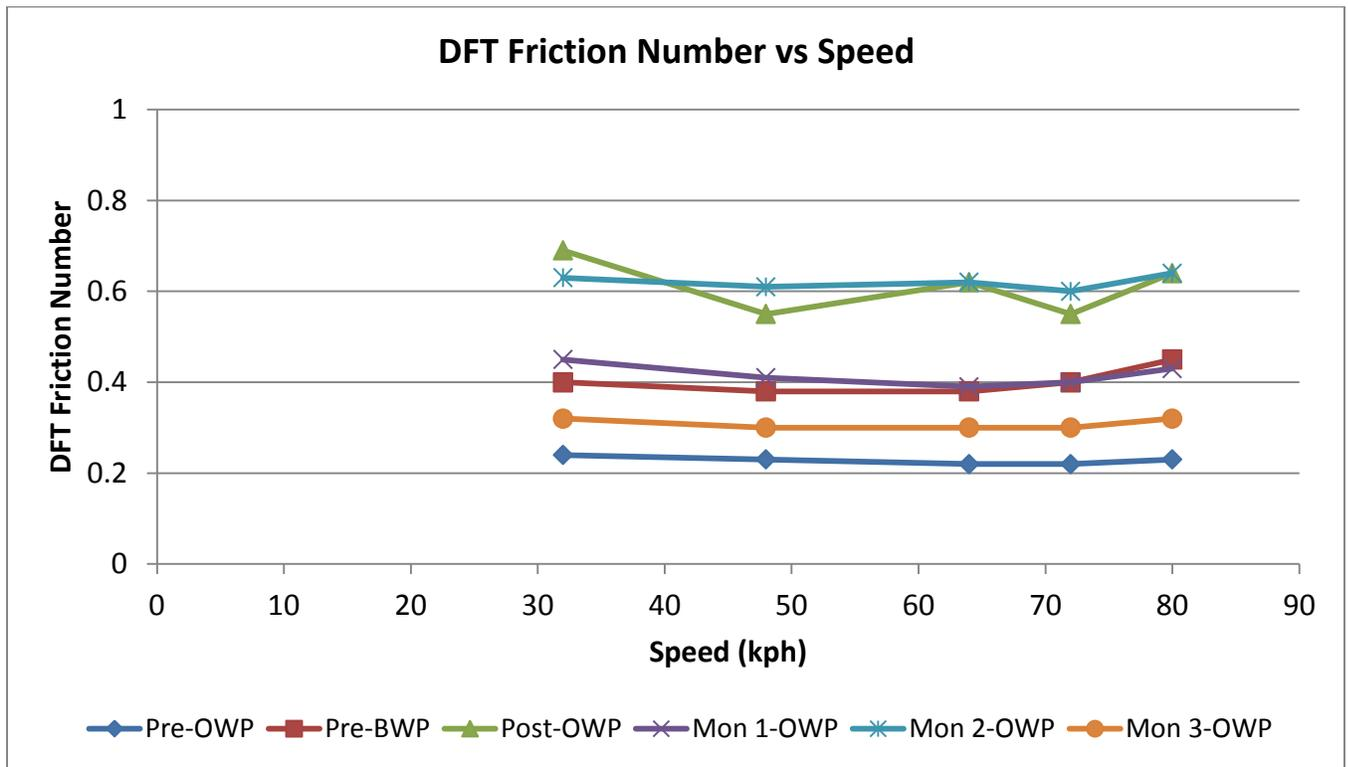
**Dynamic Friction Test (DFT) Friction Number Data for TP 3**
