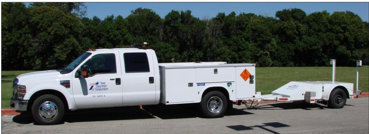
**FIGURE 2.11.** Skid Truck Used to Measure Skid Number (SN) of Pavement Surfaces.
