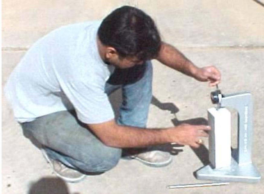
Figure 2.19 Taking Length Comparator Reading of the specimen
