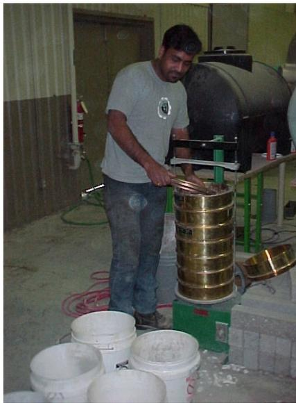
Figure 2.5 Coarse Aggregate being Sieved
