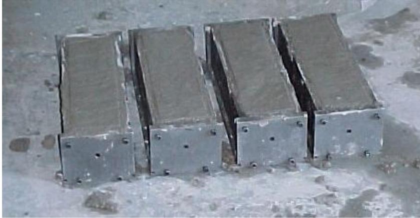
Figure 2.16 Shrinkage specimens in molds immediately after finishing
