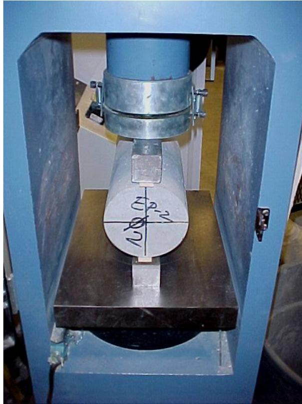
Fig. 2.26 Split cylinder test set-up
