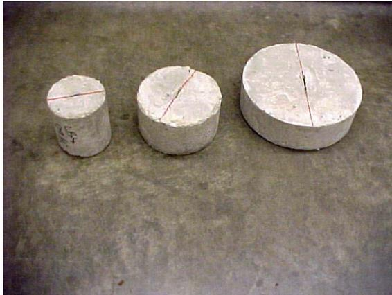
Figure 2.8 Size-Effect Specimens Ready for Testing.
