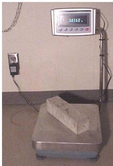
Figure 2.20 Measuring Weight of Shrinkage Specimen
