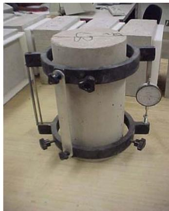
Figure 2.9 Apparatus Used to Determine Young's Modulus.
