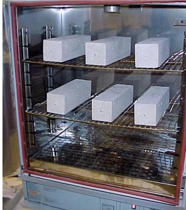
Figure 2.21 Specimens placed in the oven for drying at 110<sup>0</sup> C
