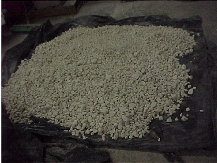
Figure 2.4 Coarse Aggregate being Air-Dried.
