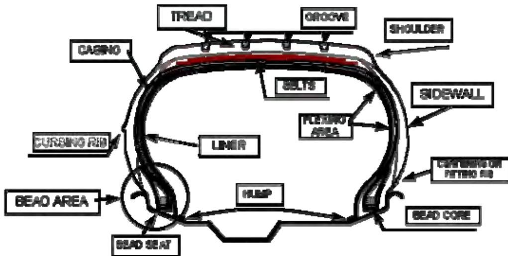
**Figure 2.3** Basic Components of a Tire (Pirelli Company 1999)
