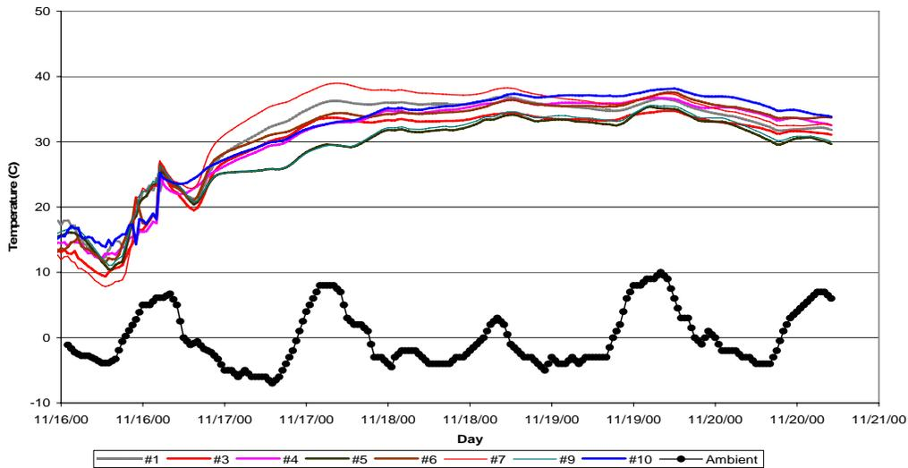
**Figures 4.1** Thermocouple and Ambient Temperatures for Six Days Following Span 6 Pour, 2<sup>nd</sup> Phase
