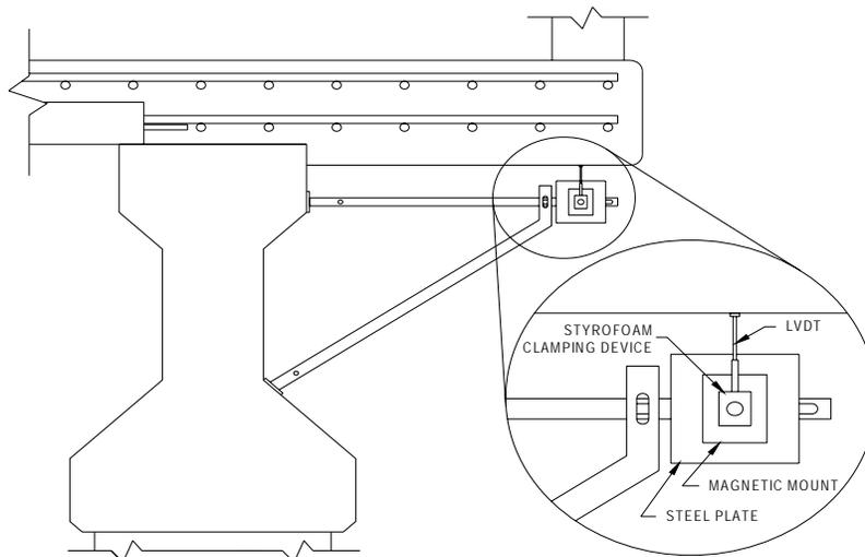
**Figure 3.3** LVDT Mounted to Measure Overhang Displacements
