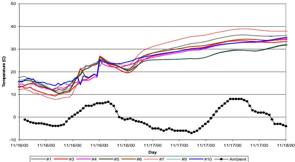
**Figures 4.2** Thermocouple and Ambient Temperatures for Two Days Following Span 6 Pour, 2<sup>nd</sup> Phase
