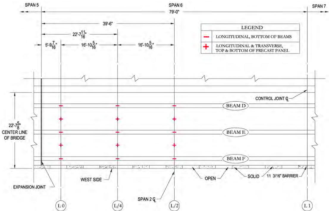
Figure 3.8 Surface-Mounted Strain Gauge Locations in Span 6
