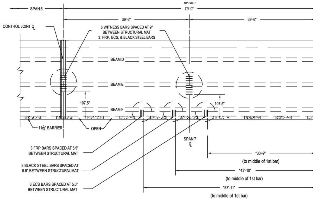
**Figure 3.15** Witness Bar Locations in Span 7
