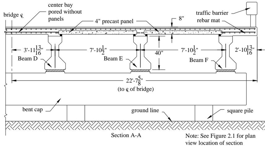
**Figure 1.2** Typical Cross Section of the Bridge Deck
