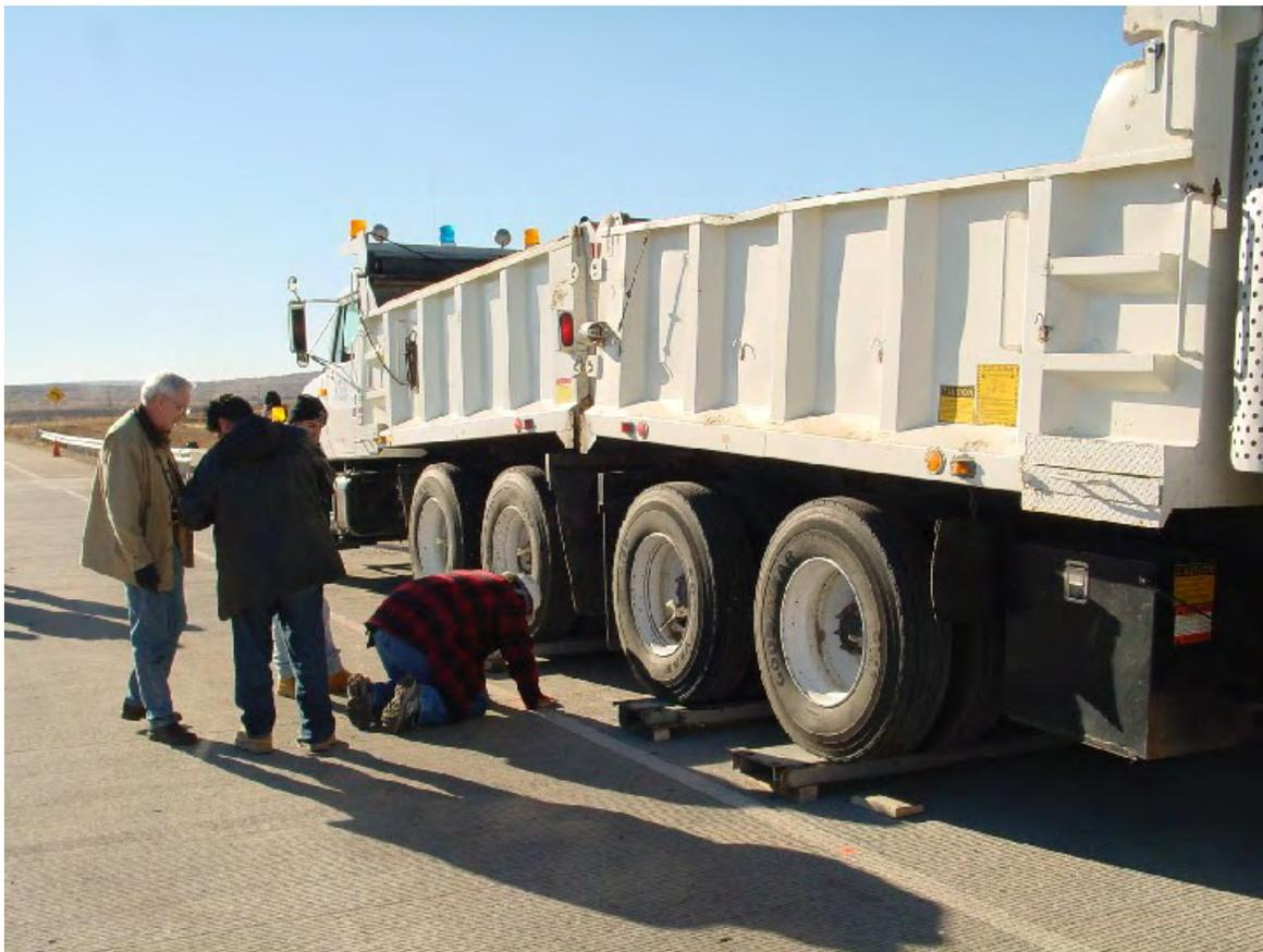
**Figure 4.3** Crack Measuring with TxDOT Dump Trucks in a Back-to-back Load Case
