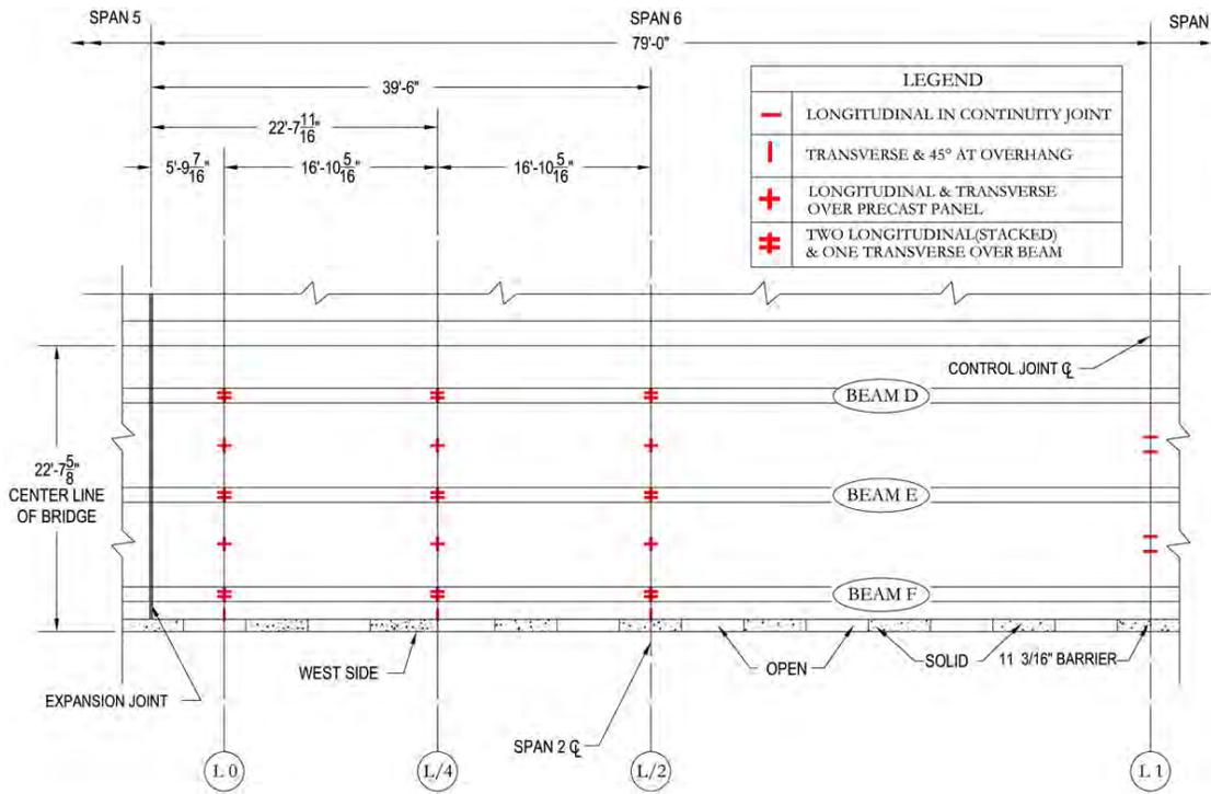
Figure 3.7 Embedded Strain Gauge Locations in Span 6
