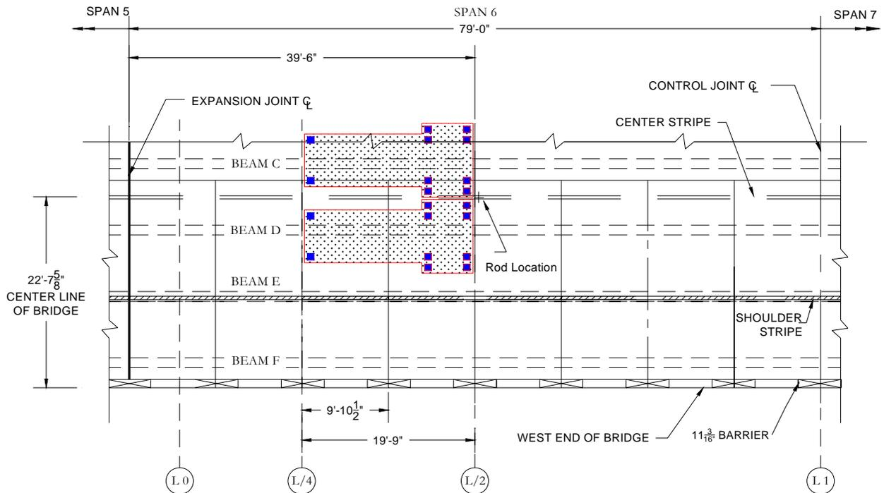
**Figure 4.7** Truck Locations for Deflection Measurement of September, 2002
