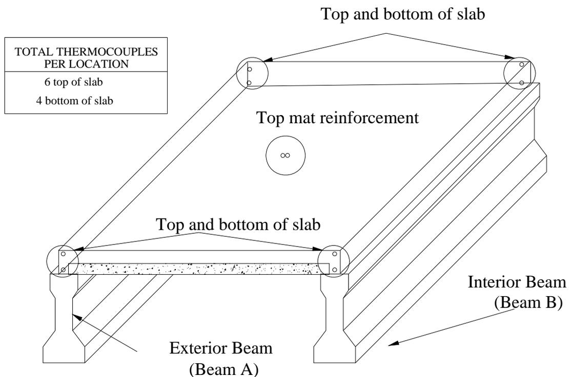
**Figure 3.2** Thermocouple Locations Centered Around a Precast Panel
