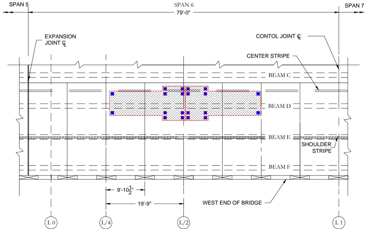
**Figure 4.6** Truck Positions for Supplemental Crack Testing
