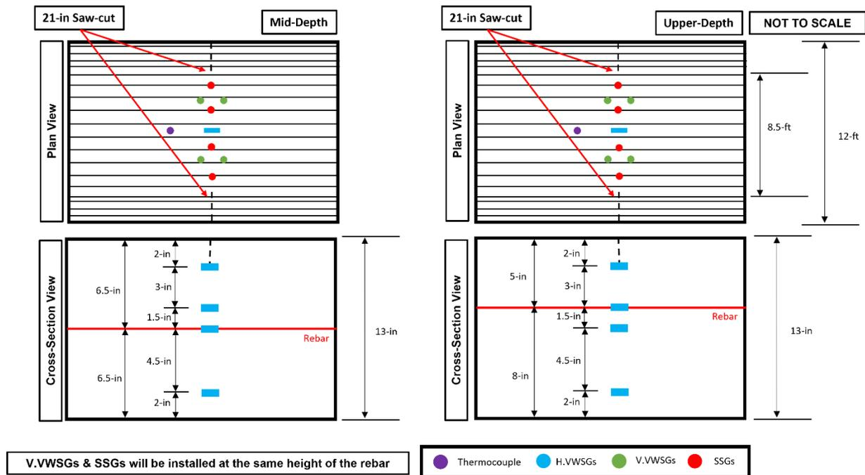
Meanwhile, another section was also instrumented with the REBEL sensors from Purdue University research team. The location of the section was at STA 212+00 where the location of the reinforcing steel was located at the upper depth (5-in from the surface). 6 REBEL sensors were installed at various locations on the north and south side of the active crack control sawcut and 4 VWSG strain gauges are various depths like the previous section's configuration as shown in the figures below.
