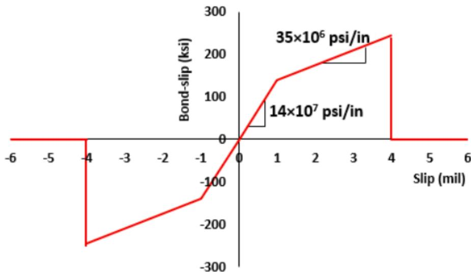
**Figure 6.6** Bond-slip #2 behavior between concrete and longitudinal steel
