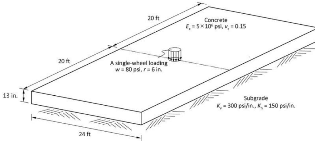
**Figure 4.1** Geometric configuration of a concrete slab
