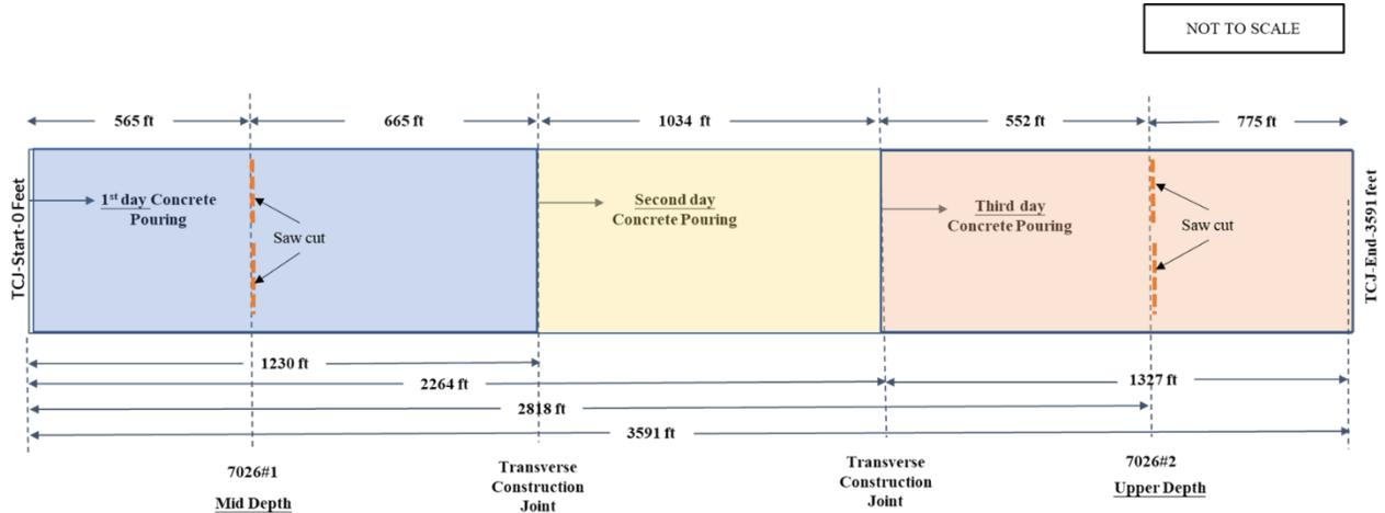
**Figure 5.11** Layout of test Section in San Antonio
