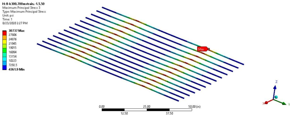
**Figure 4.18** Steel stress at transverse crack location
