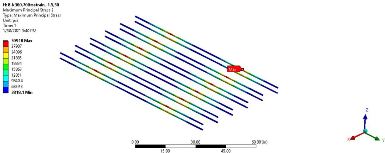
Figure 4.28 Steel stress at transverse crack location
