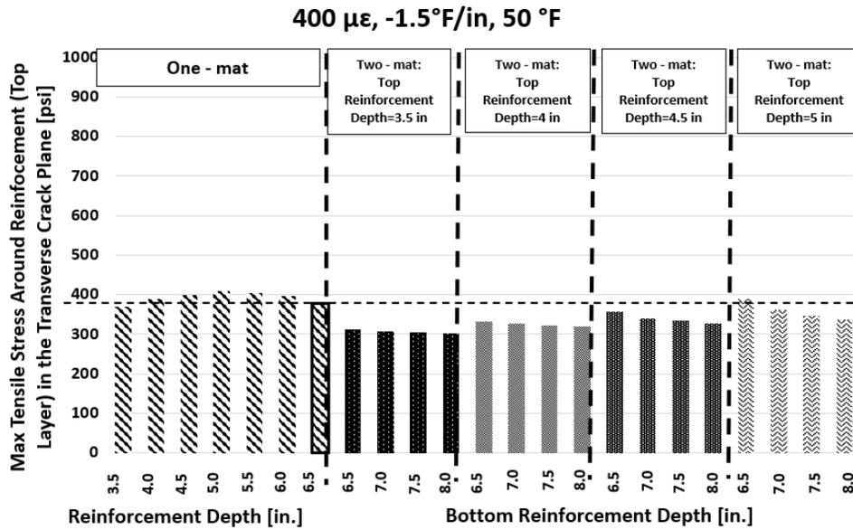
**Figure 4.31** Comparison of concrete stress on top surface in one-mat and two-mat for 400  $\mu\epsilon$  ultimate drying shrinkage
