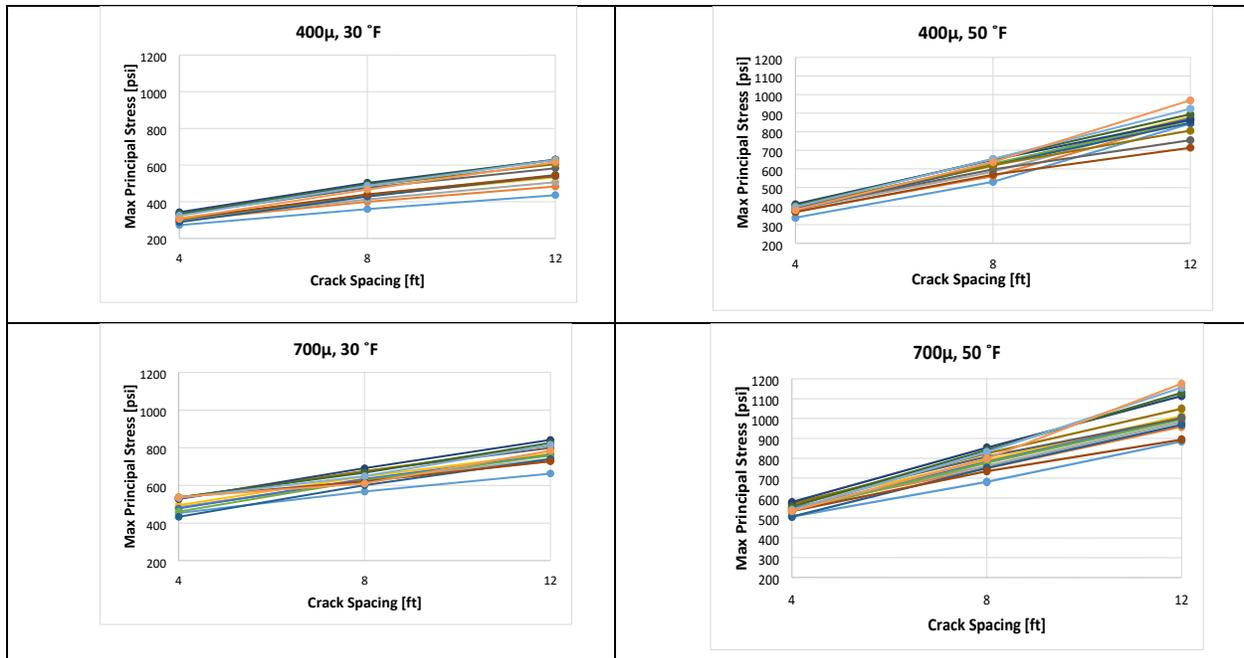
**Figure 4.15** Effect of shrinkage on crack spacing
