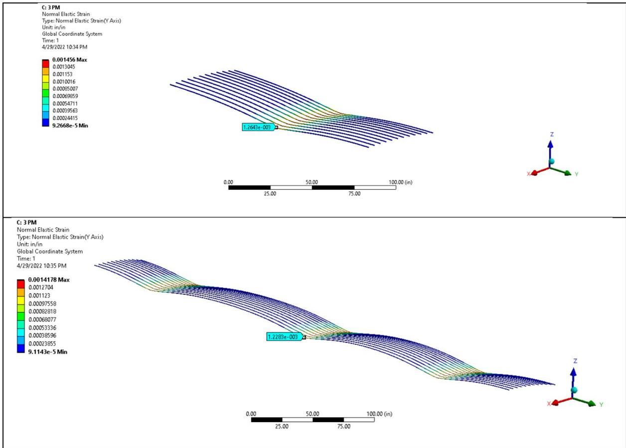
**Figure 6.4** Steel strain results from a) Model with one whole slab on east and west side of the transverse crack; b) Model with one half slab on east and west side of the transverse crack; c) Model with two slabs on east and two slabs on west side of the transverse
