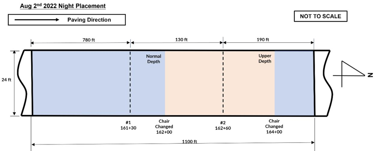
**Figure 5.13** Layout of test Section in Hillsboro
