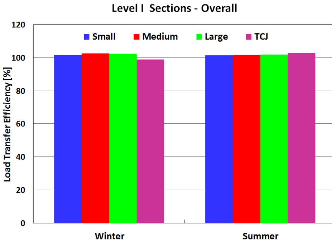
**Figure 2.16** LTE at cracks and TCJ in Texas
