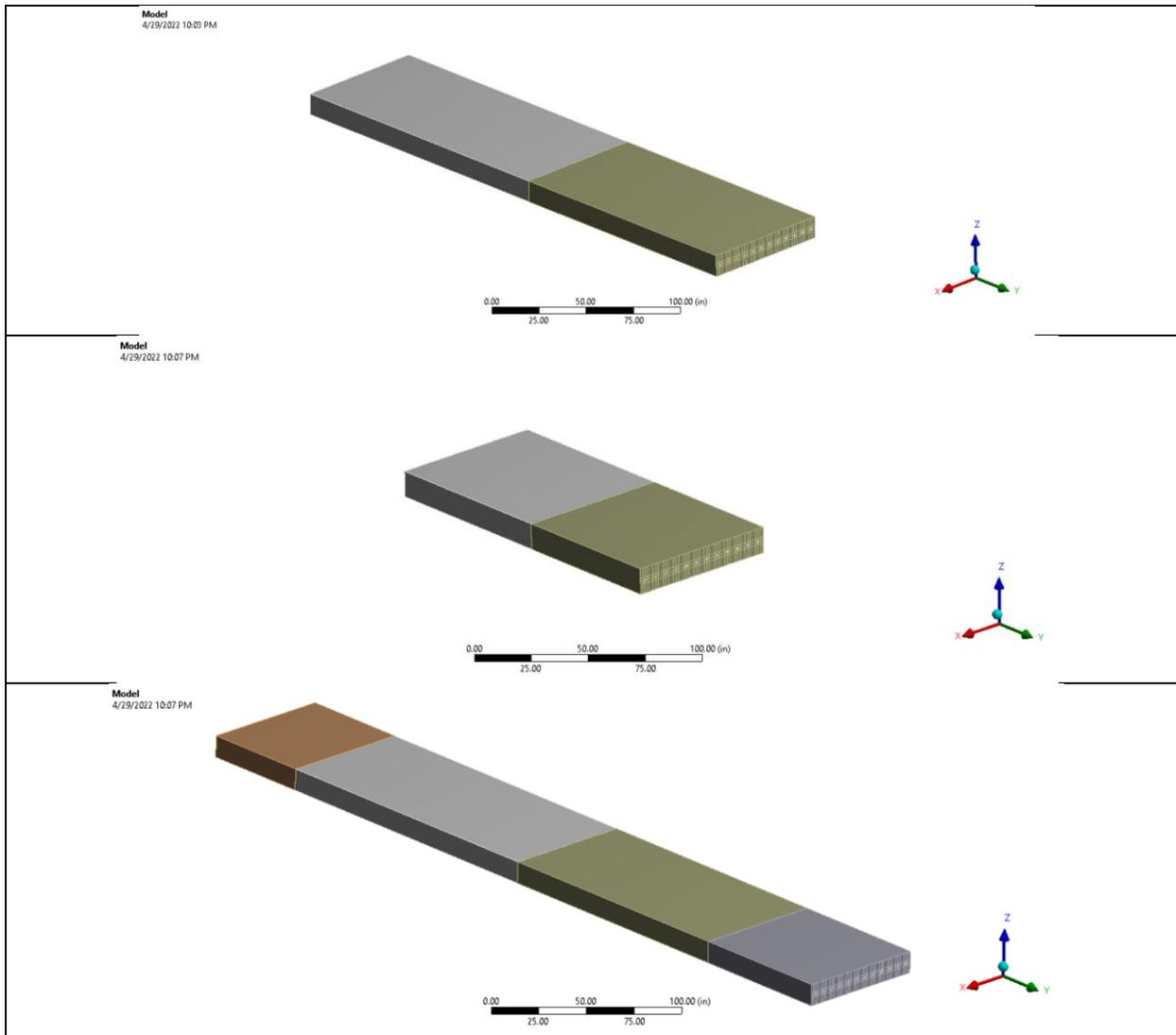
**Figure 6.3** Geometry of a) Model with one whole slab on east and west side of the transverse crack; b) Model with one half slab on east and west side of the transverse crack; c) Model with two slabs on east and two slabs on west side of the transverse crack
