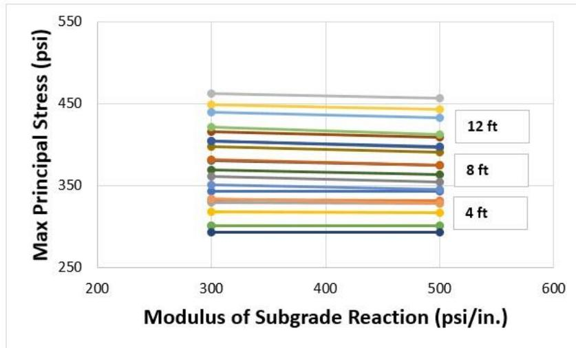
**Figure 4.11** Effect of modulus of subgrade reaction
