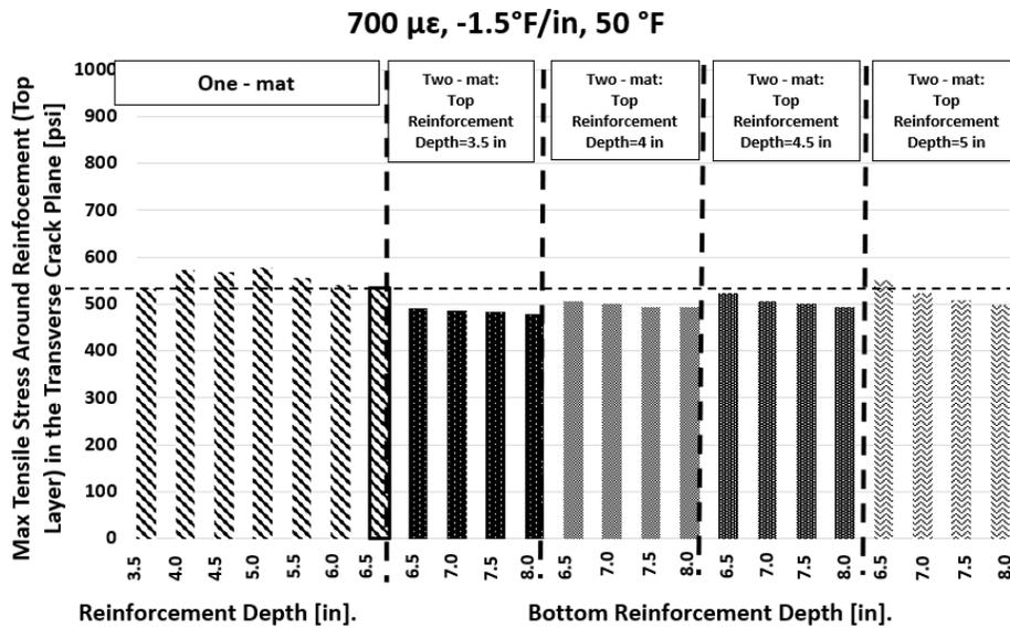
**Figure 4.32** Comparison of concrete stress on top surface in one-mat and two-mat for 700  $\mu\epsilon$  ultimate drying shrinkage
