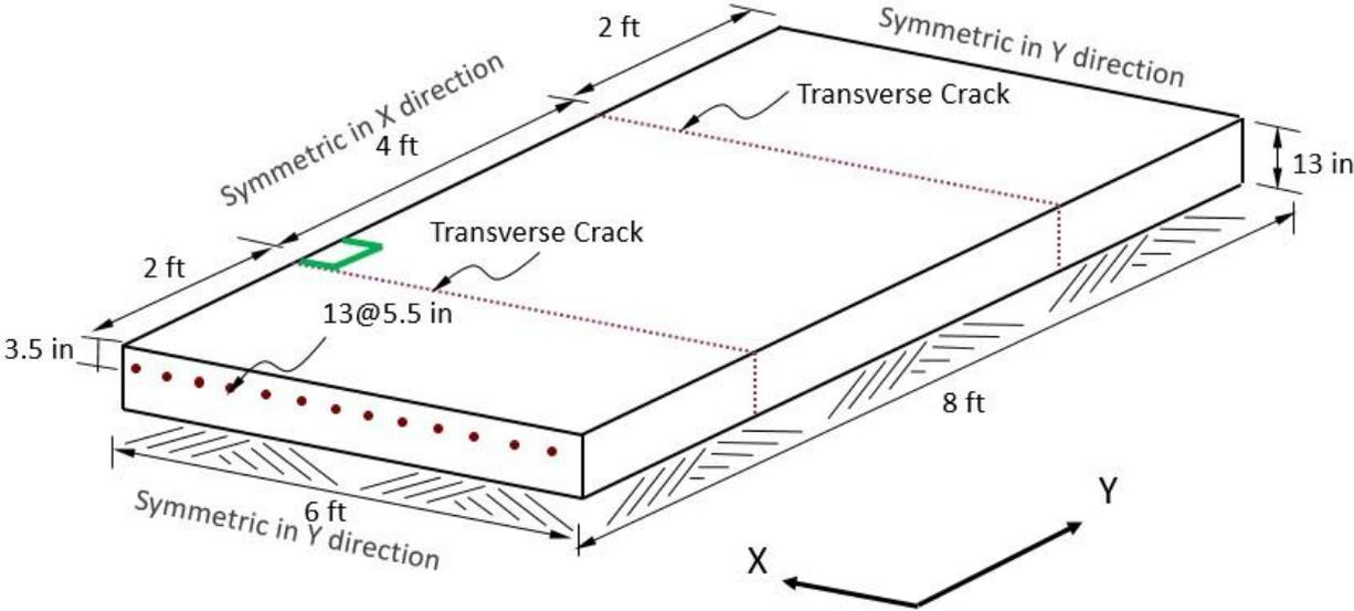
**Figure 4.8** Geometry of model of LTE evaluation
