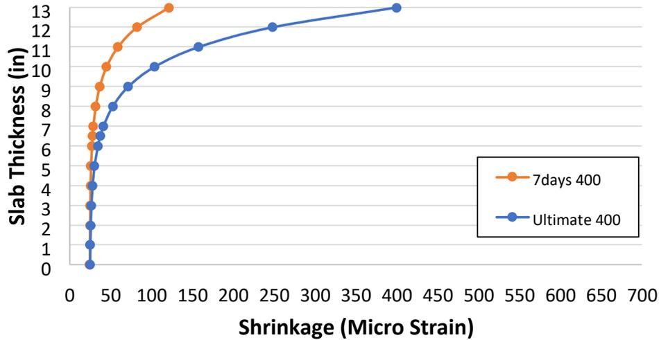
**Figure 4.6** Shrinkage changes through the slab depth with ultimate value of 400  $\mu$
