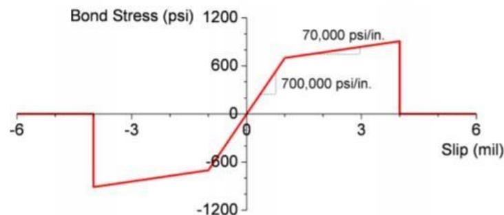
**Figure 4.5** Bond-slip behavior between concrete and longitudinal steel
