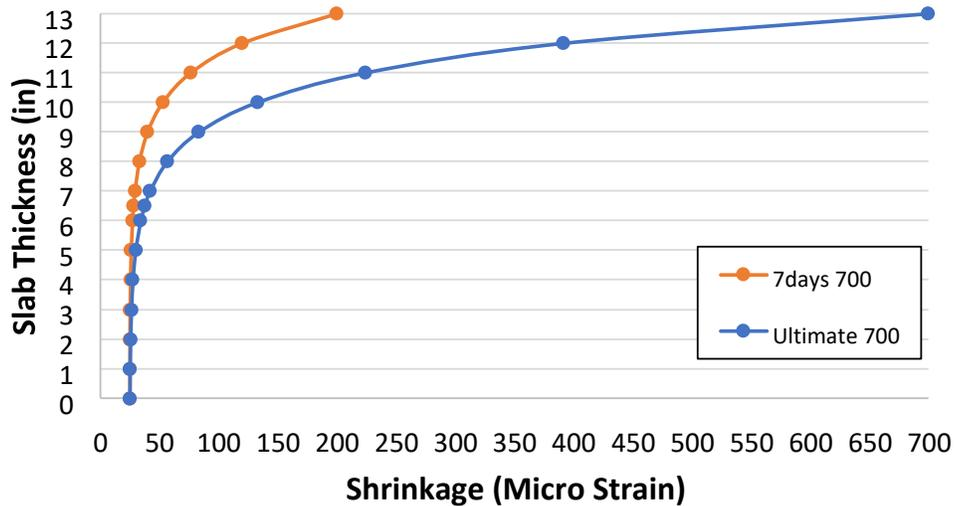
**Figure 4.7** Shrinkage changes through the slab depth with ultimate value of 700  $\mu$
