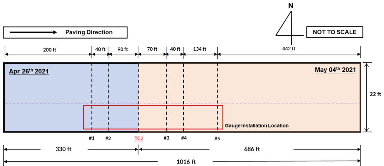
**Figure 5.7** Layout of test Section in Waxahachie
