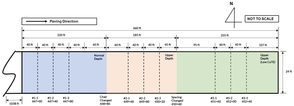
**Figure 5.9** Layout of test Section in El Paso
