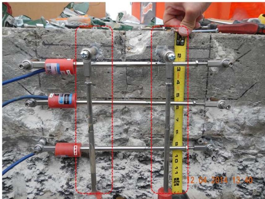
**Figure 4.9 Vertically installed crackmeters on SH 288**
