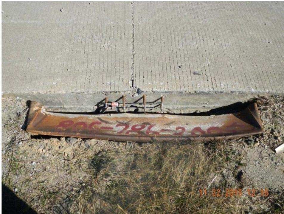
**Figure 4.12 Destroyed gages during the FDR on SH 288**
