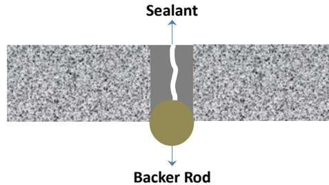
**Figure 2.2 Cohesion failure**
