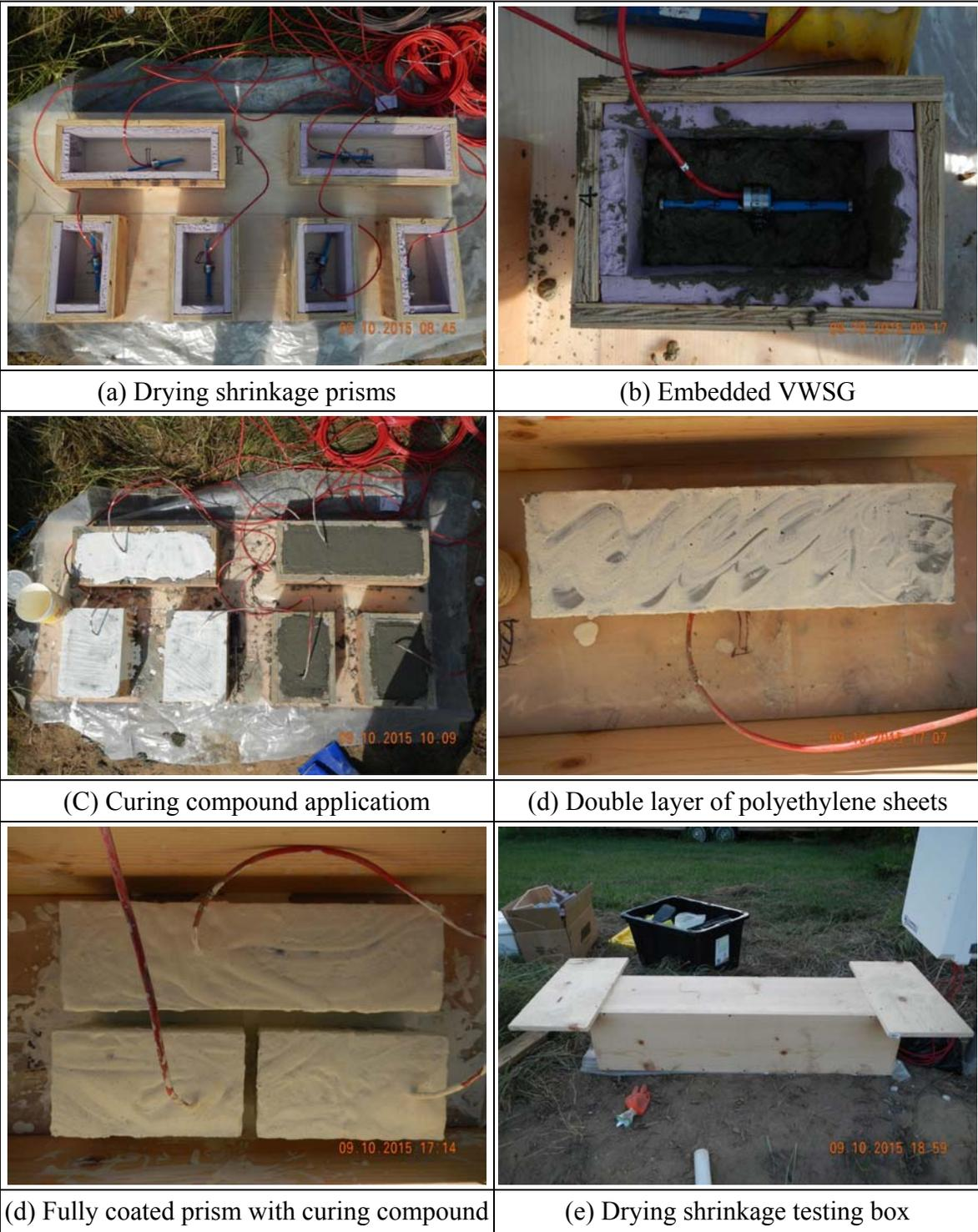
**Figure 4.14 Drying shrinkage testing on SH 288**
