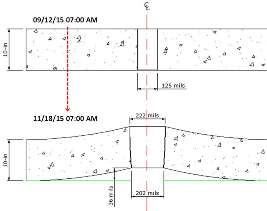
**Figure 4.25 Actual joint shape at Joint #2**
