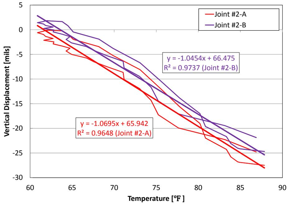
**Figure 4.11 Air temperature vs vertical displacement on SH 288**
