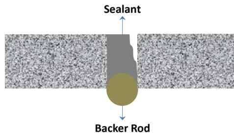
Figure 2.1 Adhesion failure
