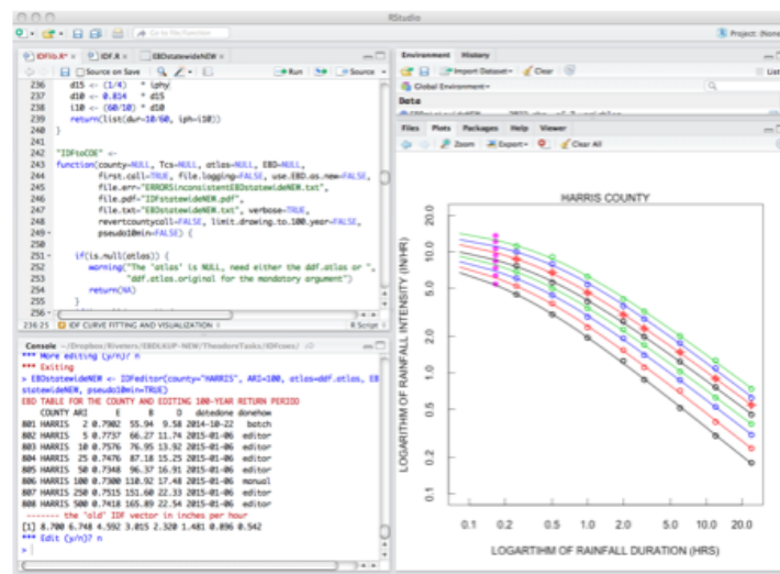
Figure 4: Screen capture of the R Software used for graphically displaying, editing, and estimating IDF curves. IDF curves displayed for Harris County, Texas is the result of adjustments from team member to construct quasi-parallel curves. Original DDF estimates are derived from Asquith (1998) and Asquith and Roussel (2004) for 2-, 5-, 10-, 25-, 50-, and 100-year ARI.
