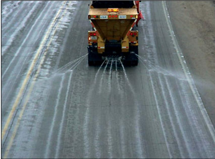
**FIG 3.** Anti-icing consists of placing liquid snow and ice control chemicals onto the roadway surface prior to the storm event
